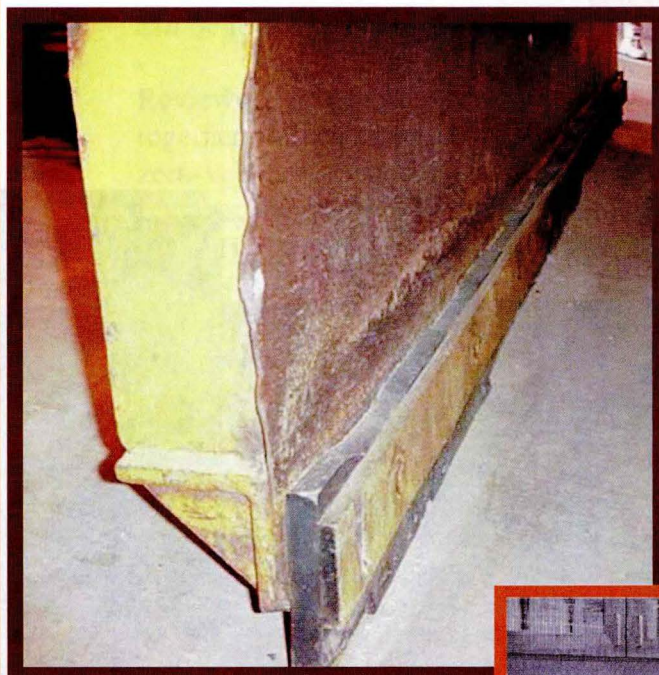
Corrosion on snow plow blade
