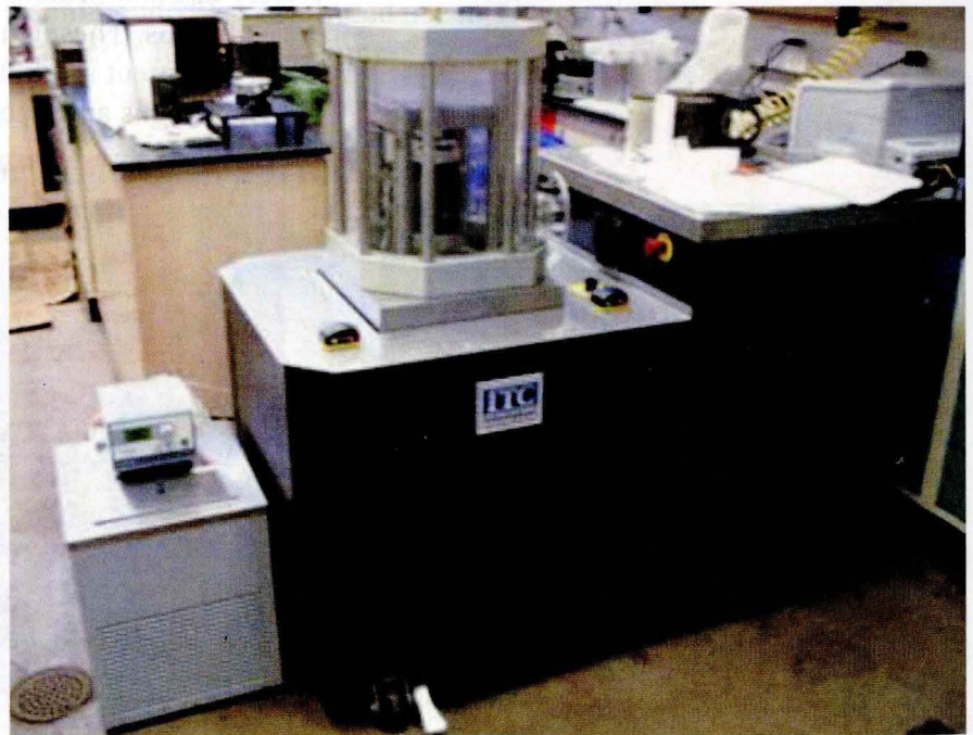
Simple Performance Testing Equipment at The University of Iowa Photo: Dr. Hosin "David" Lee, The University of Iowa/IHR
