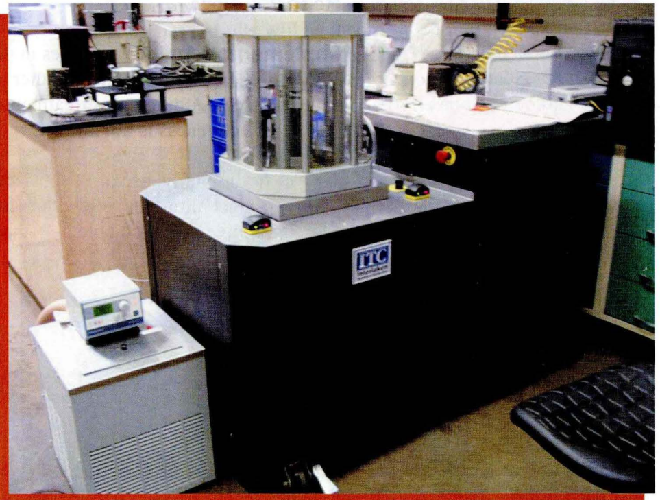
CIR-emulsion mixtures tested using Interlaken Performance Testing Equipment Photo: Dr. Hosin "David" Lee, The University of Iowa/IHR
