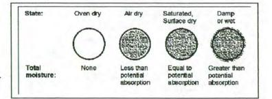
Wet batch wt. =  $\underline{Batch wt., SSD} \times 100$ (100 - % Moisture)
