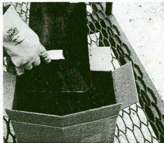
Scraping Sample off Shovel Into sample Box
