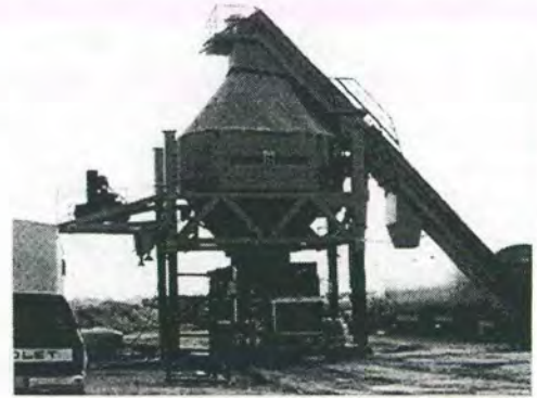
Portable Self-Erecting Silo
