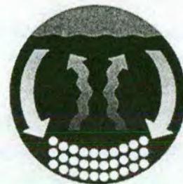
Natural Convective Currents in Asphalt Storage Tanks
