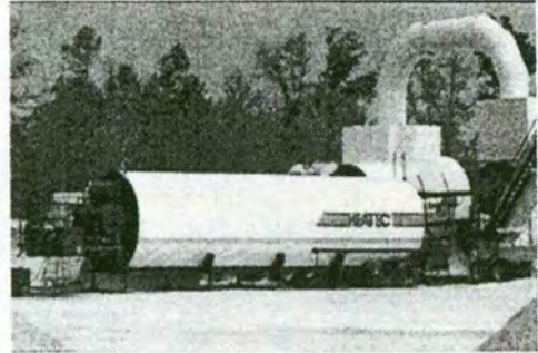
Portable Asphalt Tank
