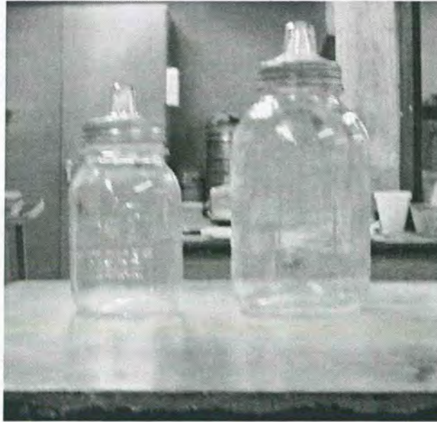
Pycnometers for Coarse and Fine Aggregates
