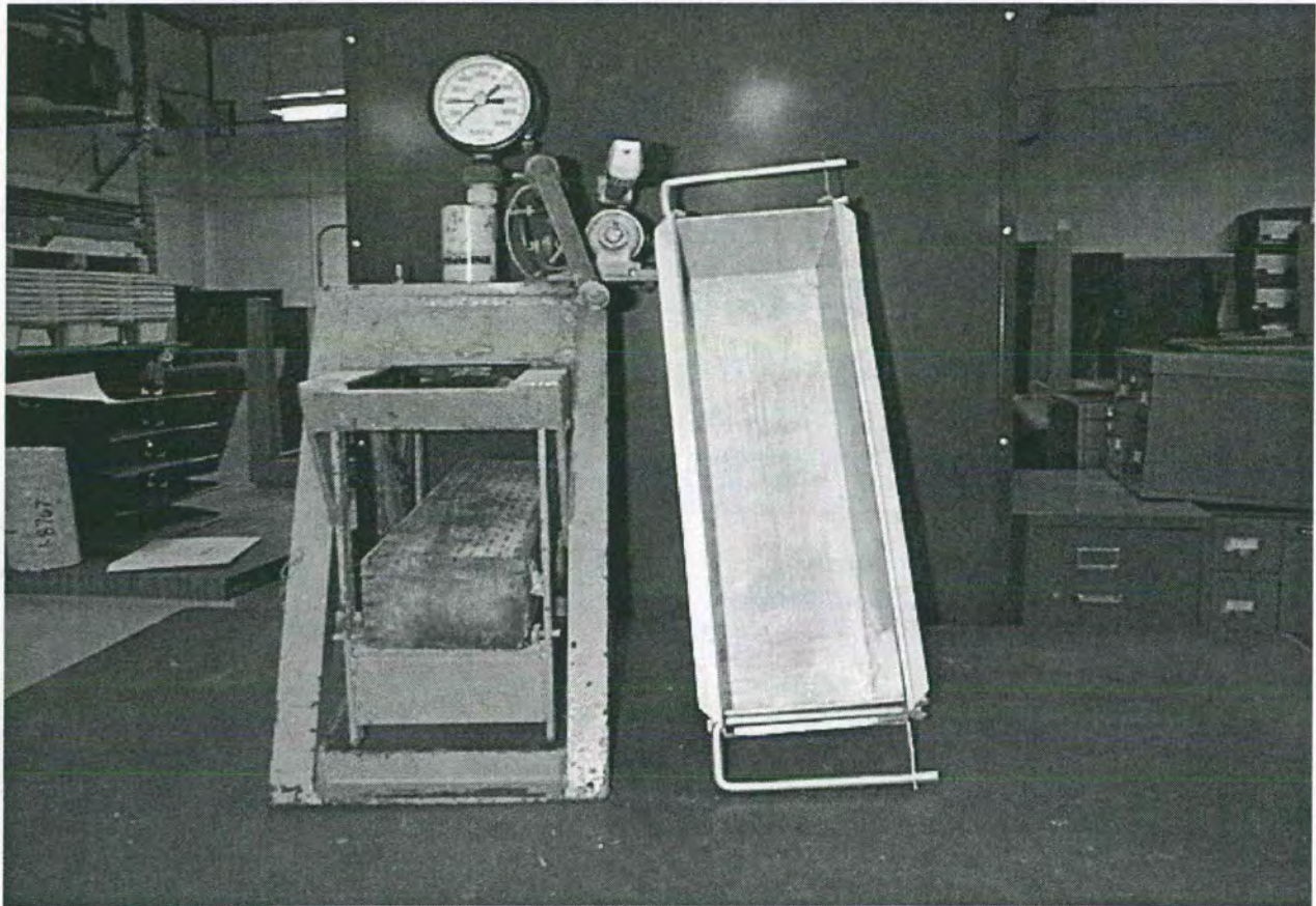
Figure 2. Concrete Specimen in Hydraulic Testing Machine
