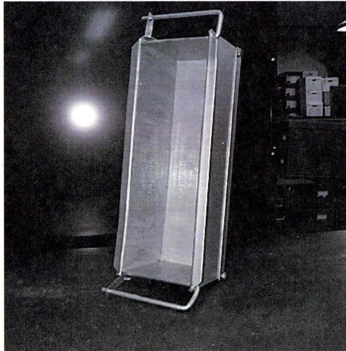
Concrete Beam Mold
