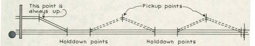
The exact position of a drape cable is shown on the Standards. The difference in cable length from the down position to the final draped position must be calculated and becomes part of the total elongation of the draped cables.
