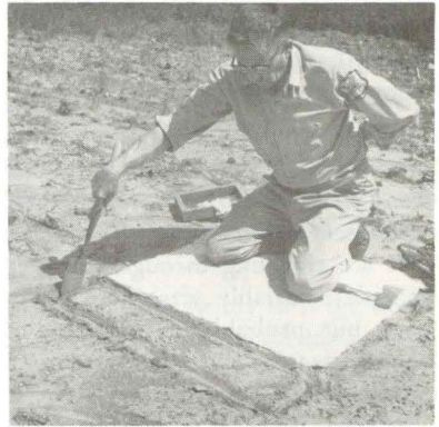
2. Ground cloth is spread and an eight-inch by 36-inch trench is dug (1½ inches deep).
