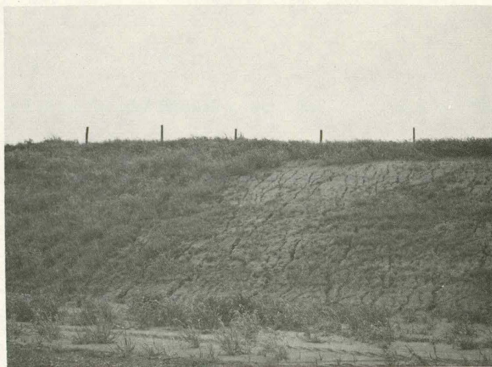
Figure 13b. Comparison of PVA with Aerospray-70, Ida County site -- vegetation difference of PVA on the left and Aerospray-70 on the right
