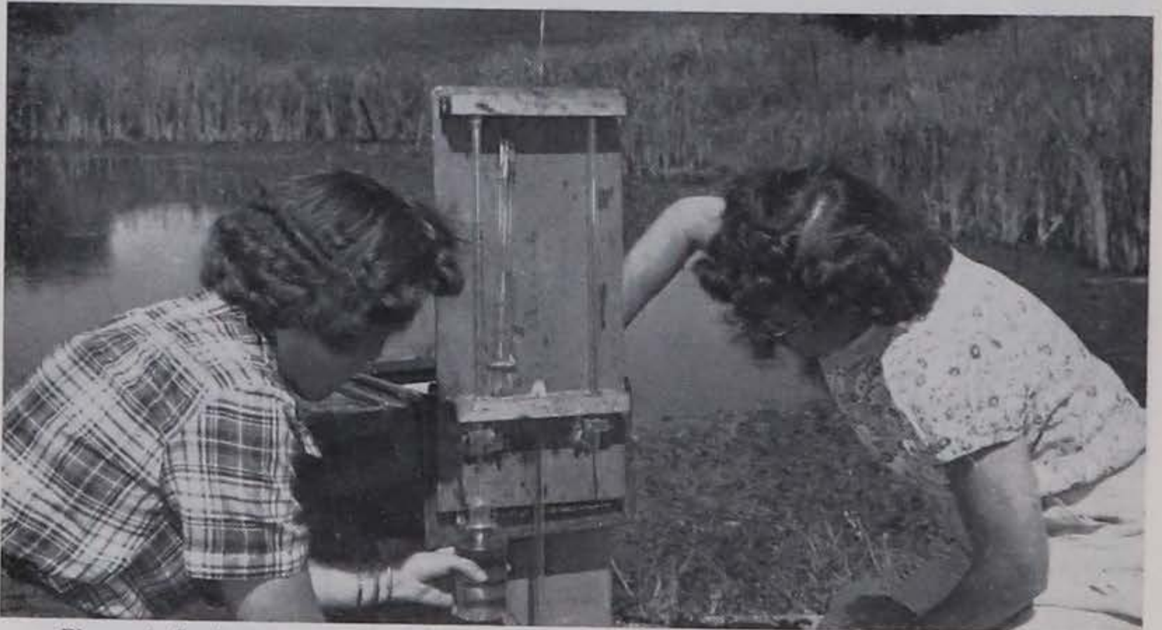
Figure 4. Students use the Winkler test for dissolved oxygen to help determine the optimum fish population for this farm pond.
