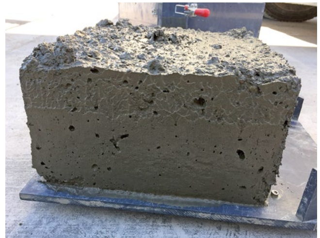
Step 4 After removing the clamps and the forms, inspect the sides for surface voids and edge slumping.
