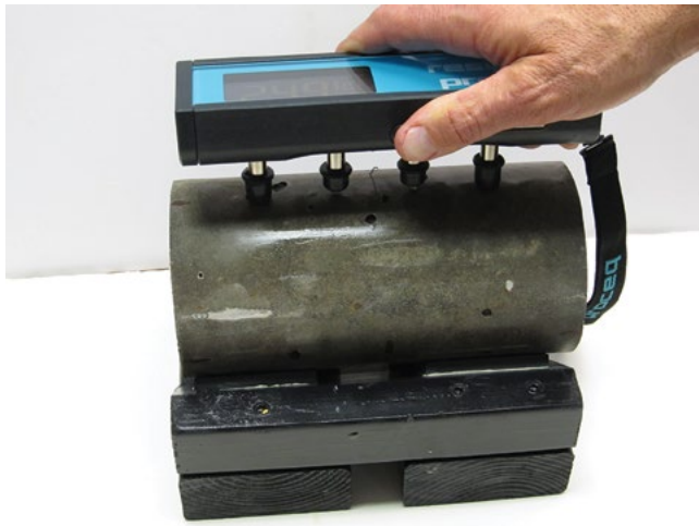
Figure 9-9. Surface resistivity gauge
