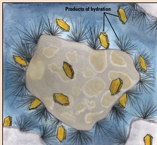
Figure 5-8. Hydration products grow
