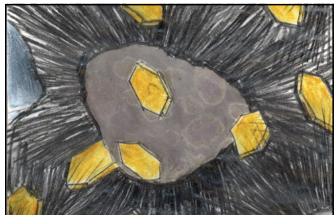
Figure 5-12. Hydration products mesh into a dense solid
