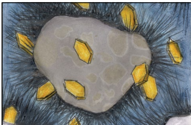
Figure 5-10. Hydration products grow during cooling
