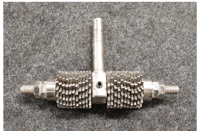
Figure 6-18. Rotating cutter with dressing wheels for the ASTM C944 abrasion resistance test
