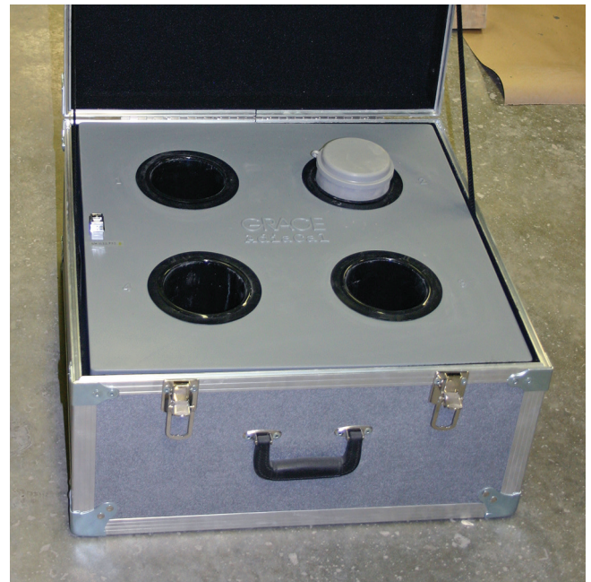
Figure 6-8. A typical field semi-adiabatic temperature monitoring system for mortar
