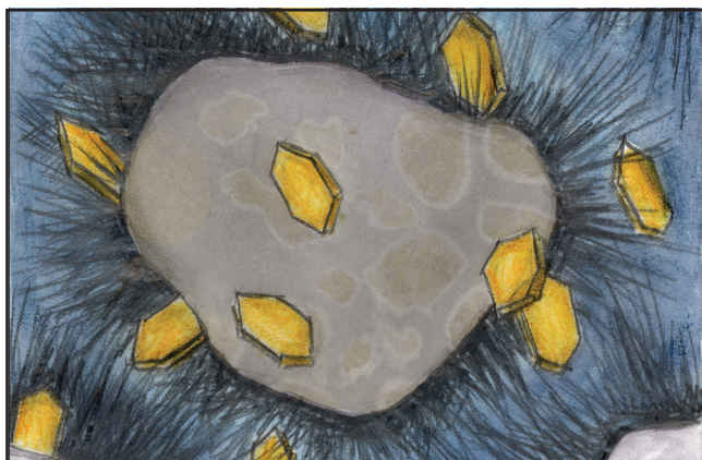
Figure 5-10. Hydration products grow during cooling
