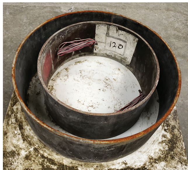
Figure 6-25. Gauged invar rings for casting concrete to monitor both expansion and shrinkage stresses
