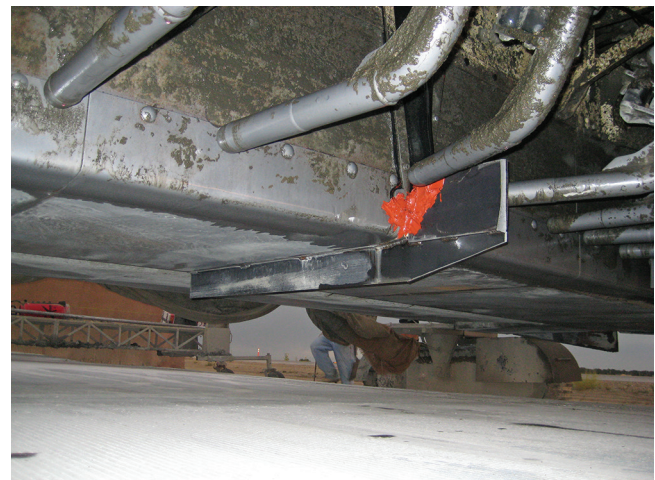
Figure 8-14. An array of vibrators under a slipform paver
