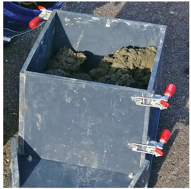
Step 2 Construct box and place clamps tightly around box. Hand scoop mixture into box until the concrete height is 9.5 in.
