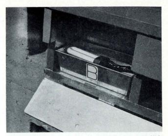
Fig. 16. A compartment of the experimental light trap. A blacklight lamp is suspended over a pan of detergent water. Note that the front of the trap is hinged.
