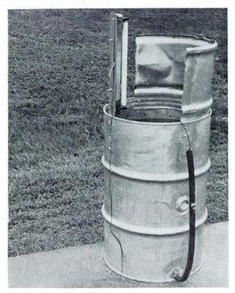
Fig. 17. Blacklight caddisfly trap used at Keokuk. Recommended for use in possible control measures.
