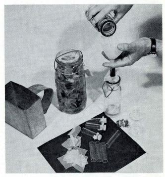
Fig. 3. Collecting pan, funnel, sections of glass tubing and certain materials used to collect, concentrate and store large numbers of small Fig. 3.
