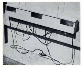
Fig. 15. Experimental light trap which tested three types of lights as caddisfly attractants.
