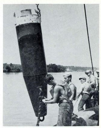
Fig. 9. Navigation buoy and its anchor chain being raised from the river.
