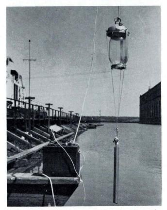
Fig. 7. Light trap used to capture caddisflies which oviposit underwater.
