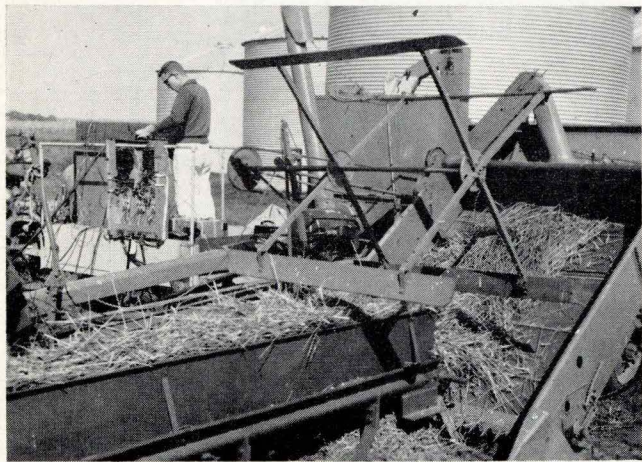
Fig. 12. Conveyor belt feeding of the combine in the stationary load study.
