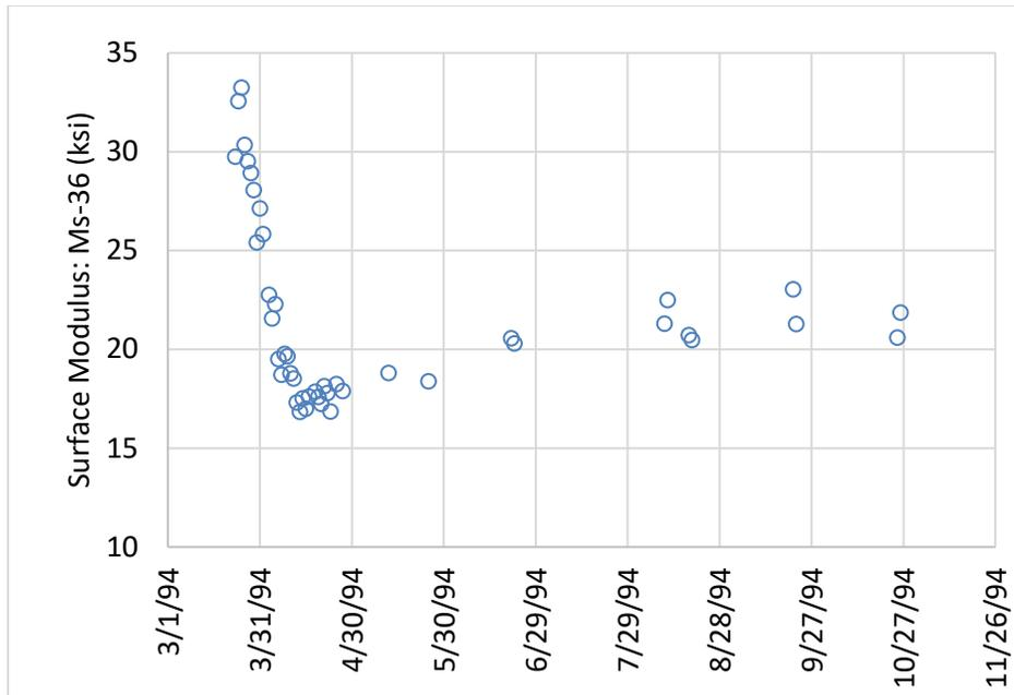
**Figure 12. Daily average surface modulus (Ms-36) values from Cell 26 (1994)**
