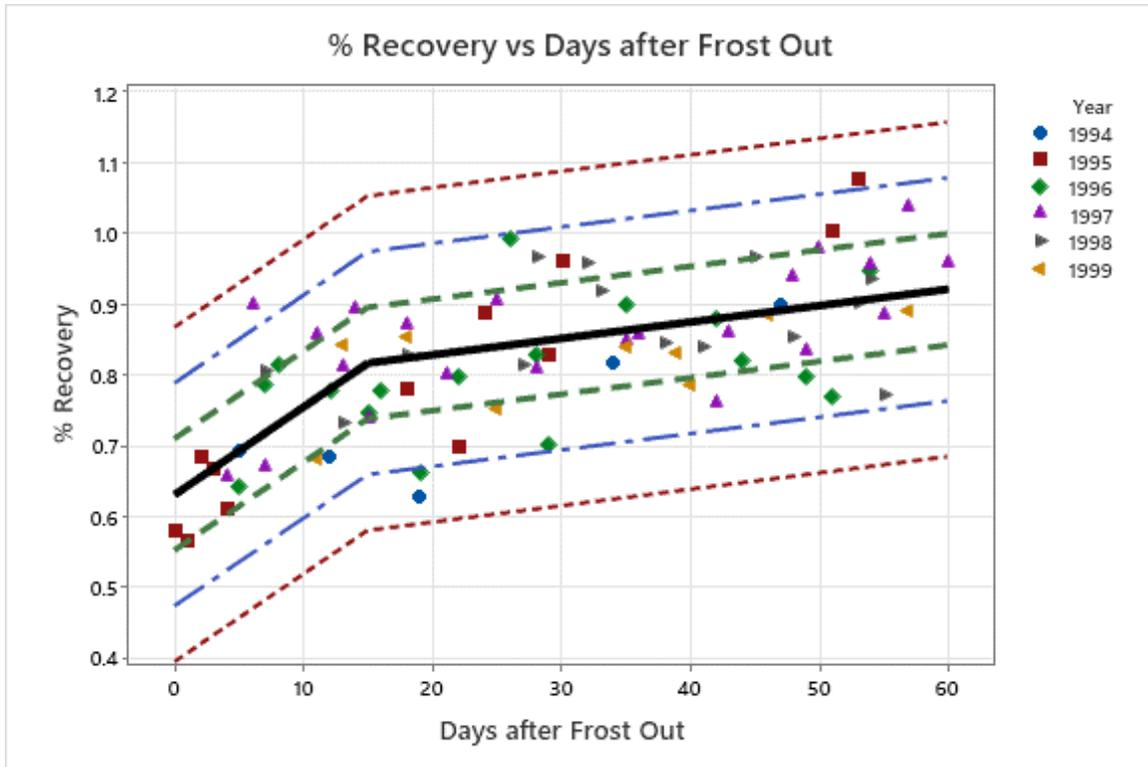
**Figure 35. Final model with  $\pm 3$  standard error bands showing data used to build model**
