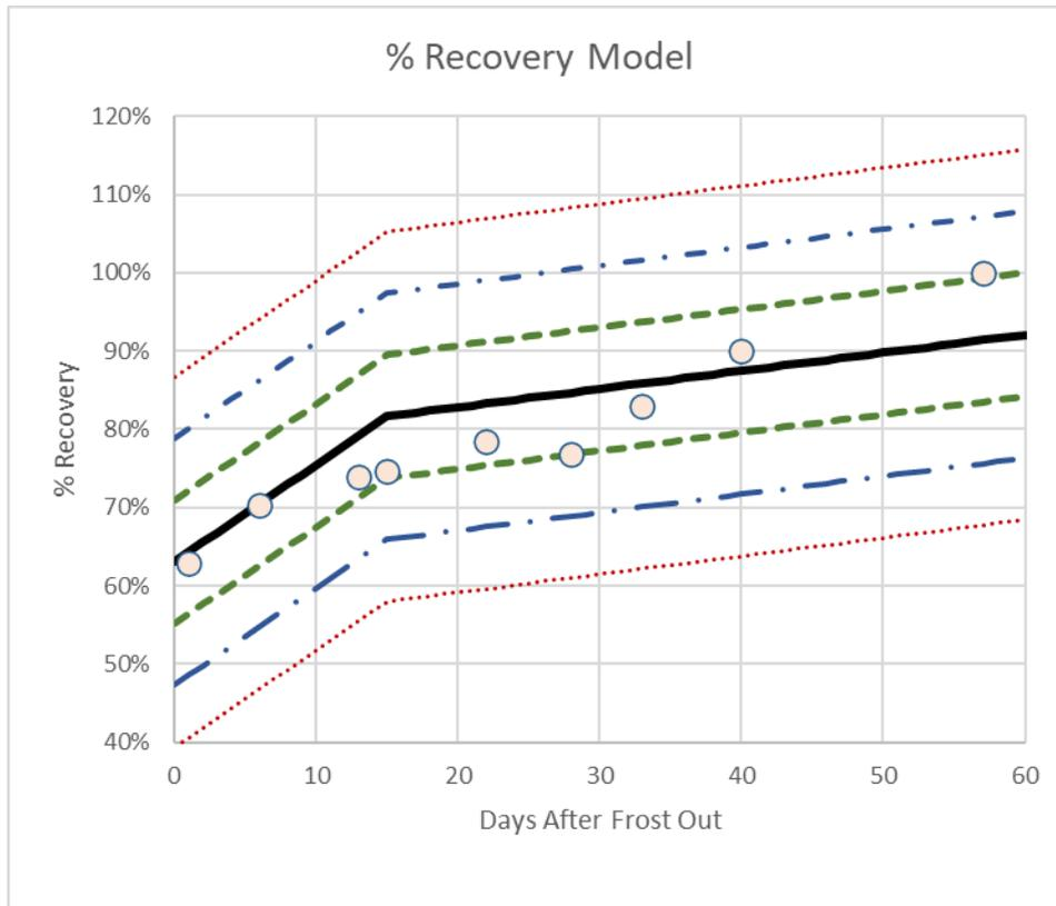
**Figure 41. Final model with  $\pm 3$  standard error bands with Stinson Lake, New Hampshire, data**
