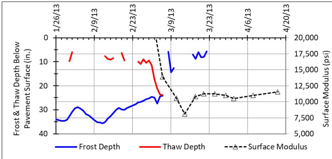
**Figure 46. Frost and thaw depths (including secondary freezing) and surface modulus values at Madison, Maine (2013)**
