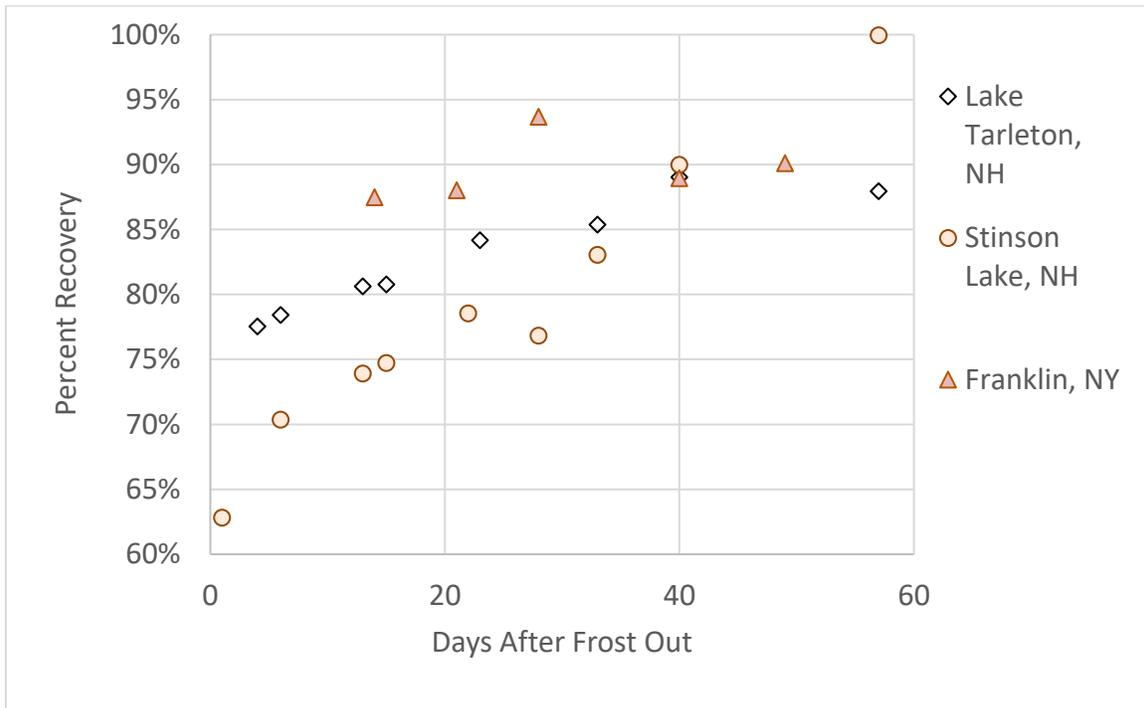
**Figure 28. Validation data from three silty sand subgrade sites**
