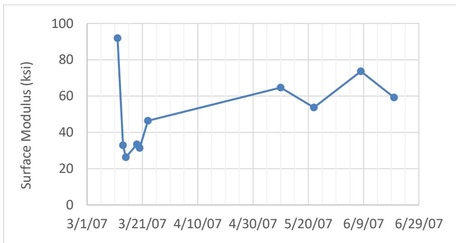
**Figure 50. Surface modulus values at MnROAD Cell 28 (2007)**
