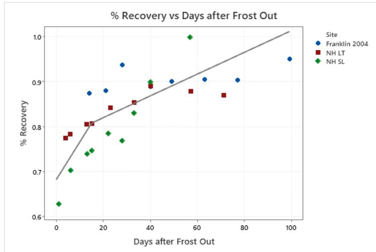
**Figure 20. Scatterplot of percent recovery for three sites with silty sand subgrades**
