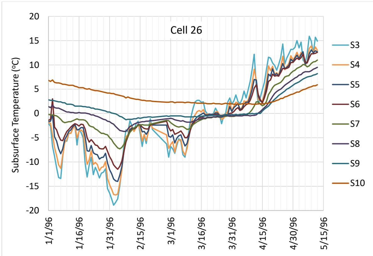
**Figure 9. Plot of subsurface temperatures at MnROAD Cell 26 (January 1 through May 15, 1996)**
