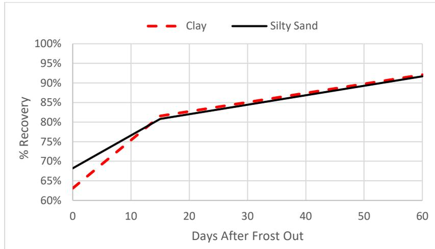
**Figure 21. Percent recovery trends for clay versus silty sand subgrades**
