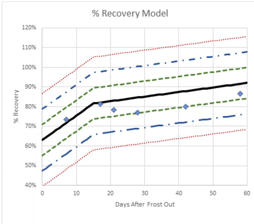
**Figure 37. Final model with  $\pm 3$  standard error bands with Lyme, Jefferson County, New York, data**
