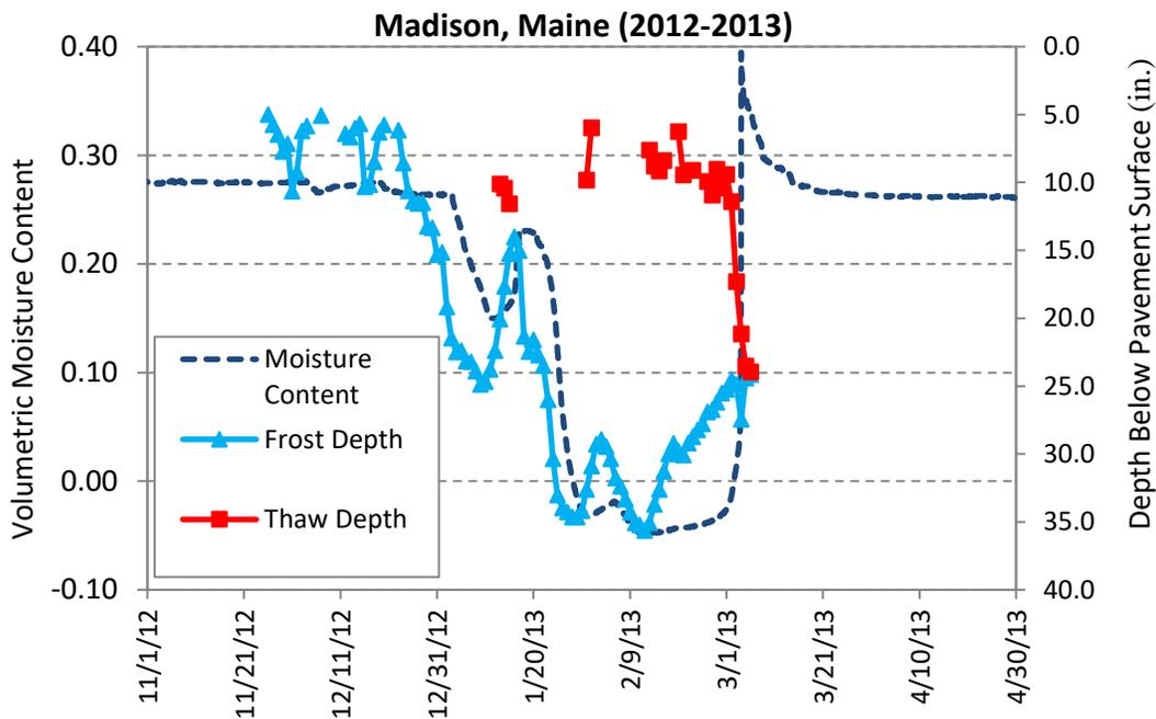
**Figure 45. Frost and thaw depths and volumetric moisture content at Madison, Maine (2012–2013)**
