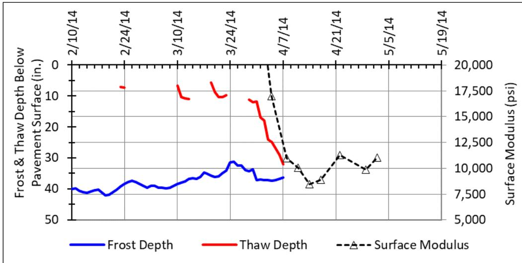
**Figure 48. Frost and thaw depths and surface modulus values at Madison, Maine (2014)**
