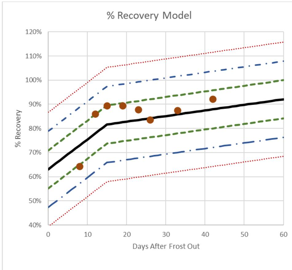
**Figure 38. Final model with  $\pm 3$  standard error bands with 2013 Madison, Maine, data**
