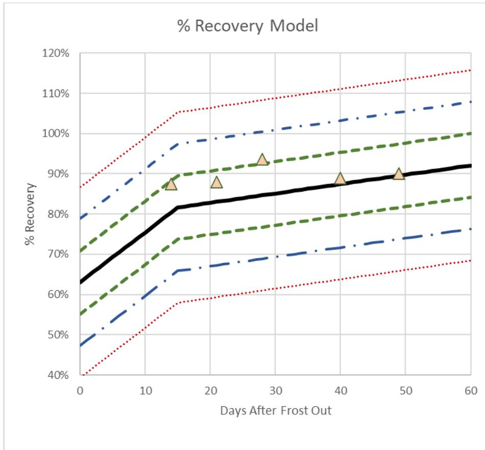
**Figure 42. Final model with  $\pm 3$  standard error bands with 2004 Franklin, New York, data**
