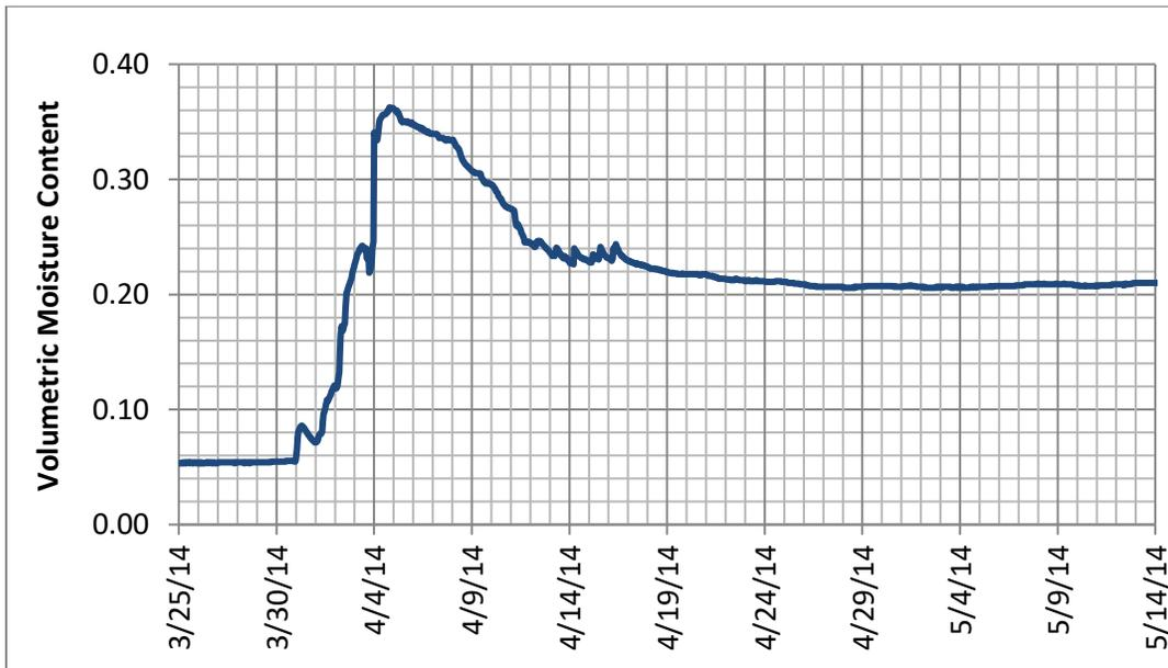
**Figure 49. Volumetric moisture content at Madison, Maine (2014)**
