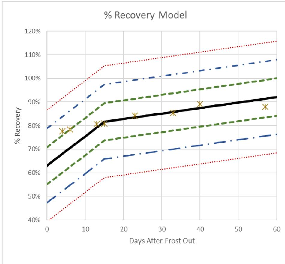
**Figure 40. Final model with  $\pm 3$  standard error bands with Lake Tarleton, New Hampshire, data**
