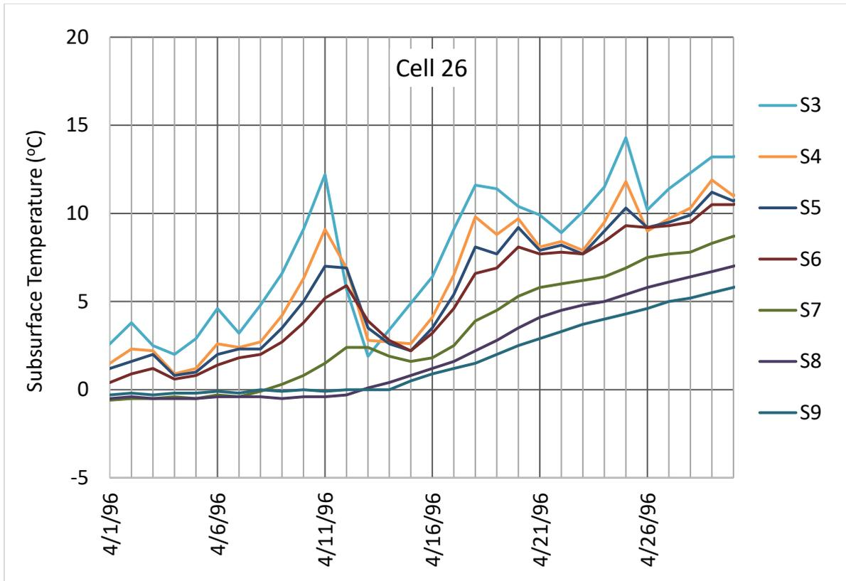
**Figure 10. Plot of subsurface temperatures at MnROAD Cell 26 (April 1 through 30, 1996)**
