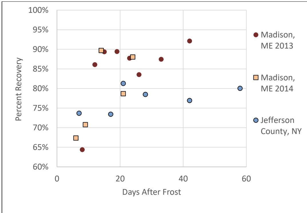
**Figure 29. Validation data from two clay subgrade sites**
