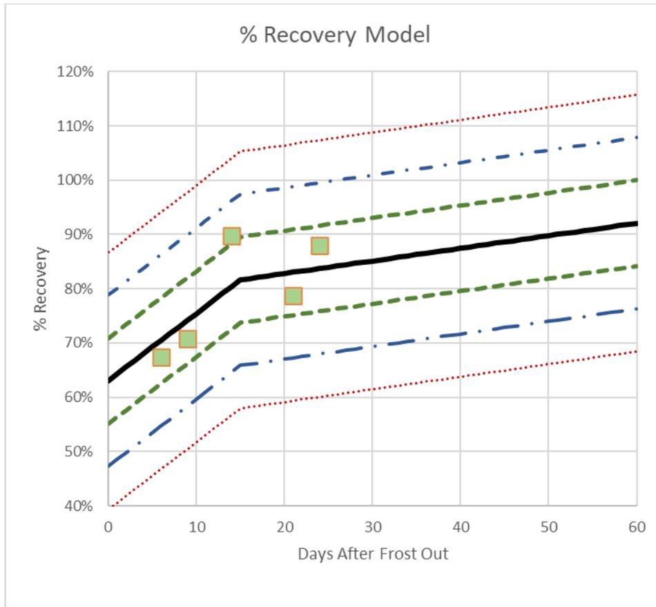
**Figure 39. Final model with  $\pm 3$  standard error bands with 2014 Madison, Maine, data**
