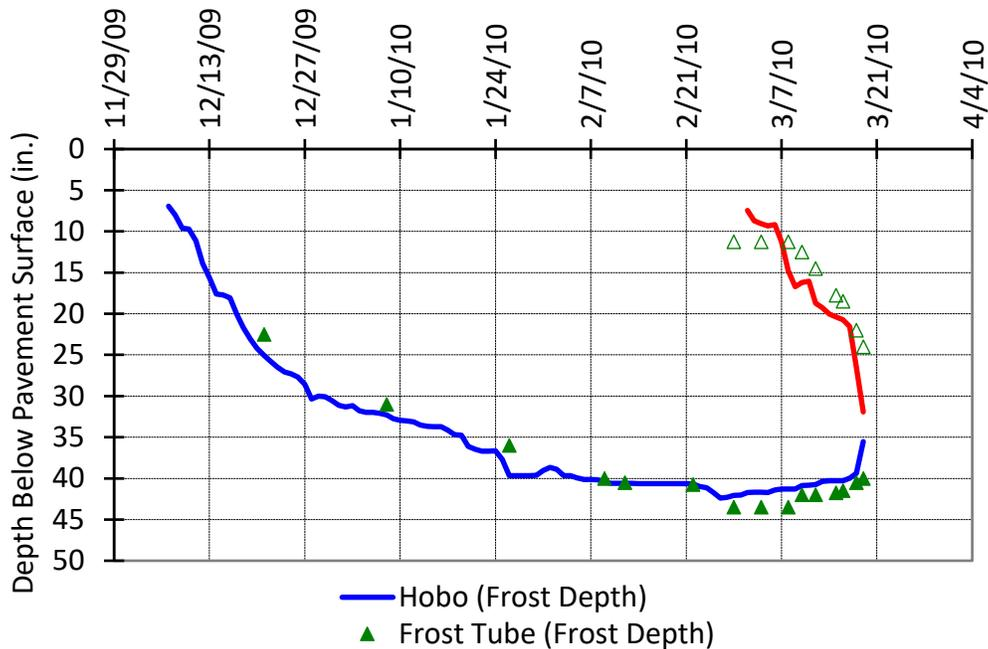
**Figure 8. Comparison of frost and thaw depths determined from thermistors and frost tubes at the Lake Tarleton, New Hampshire, site**
