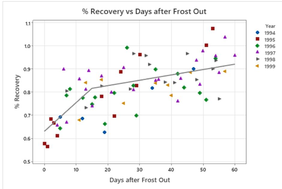
Figure 18. Scatterplot of percent recovery for MnROAD Cell 28 during 1994–1999
