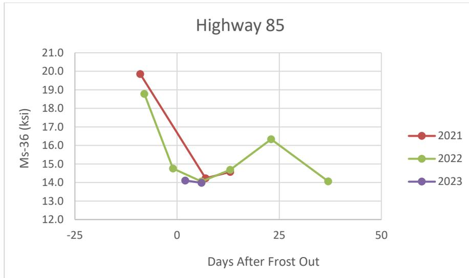
**Figure 32. Plot of Ms-36 versus days after frost out at Highway (US) 85**
