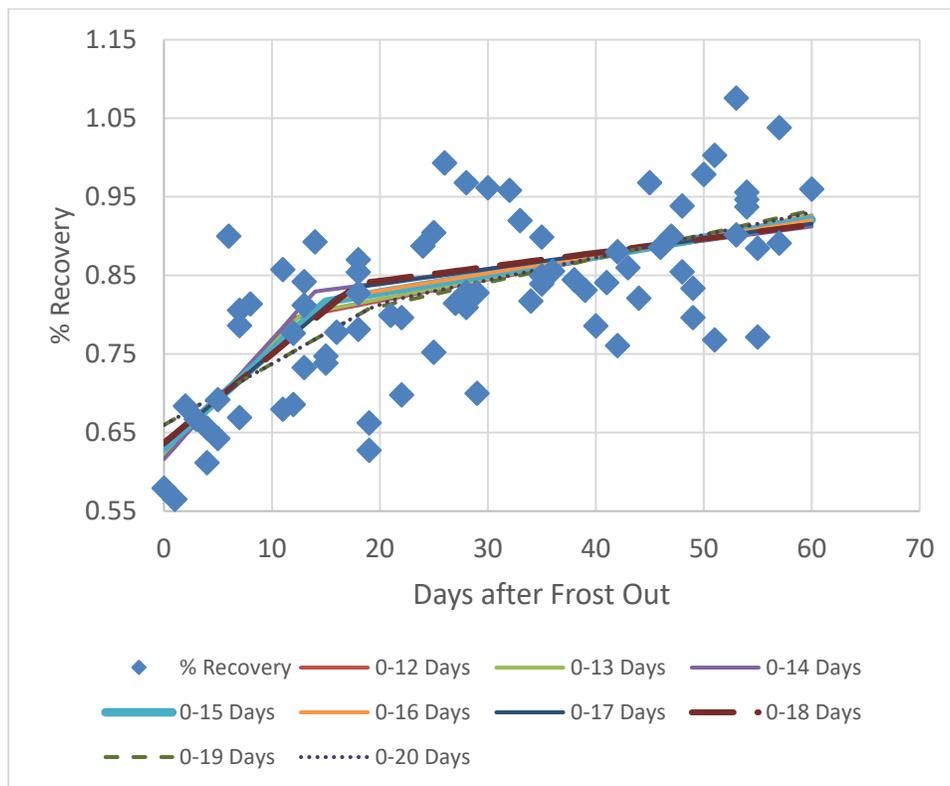
**Figure 19. Bilinear regression lines with breakpoint varied from 12–20 days**
