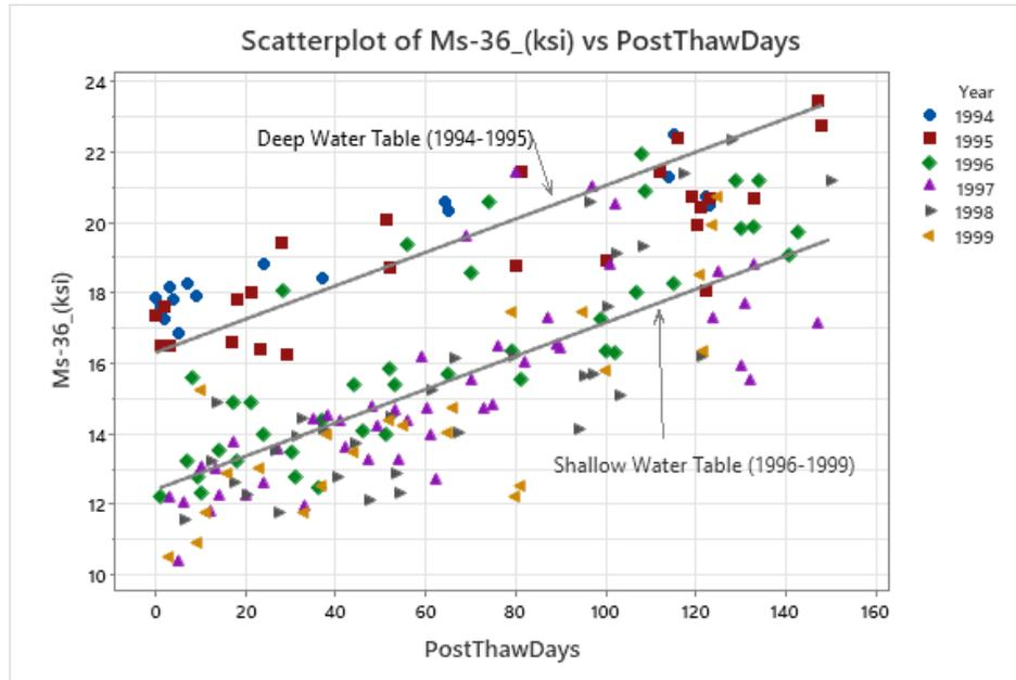
**Figure 16. Cell 26 Ms-36 0–150 days post frost 1994–1999 with regression lines based on days after frost out and GWT**
