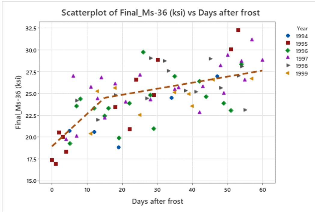
**Figure 17. Cell 28 Ms-36 (ksi) 0–60 days post frost 1994–1999 with high residual data removed and dashed line showing fitted bilinear regression line**
