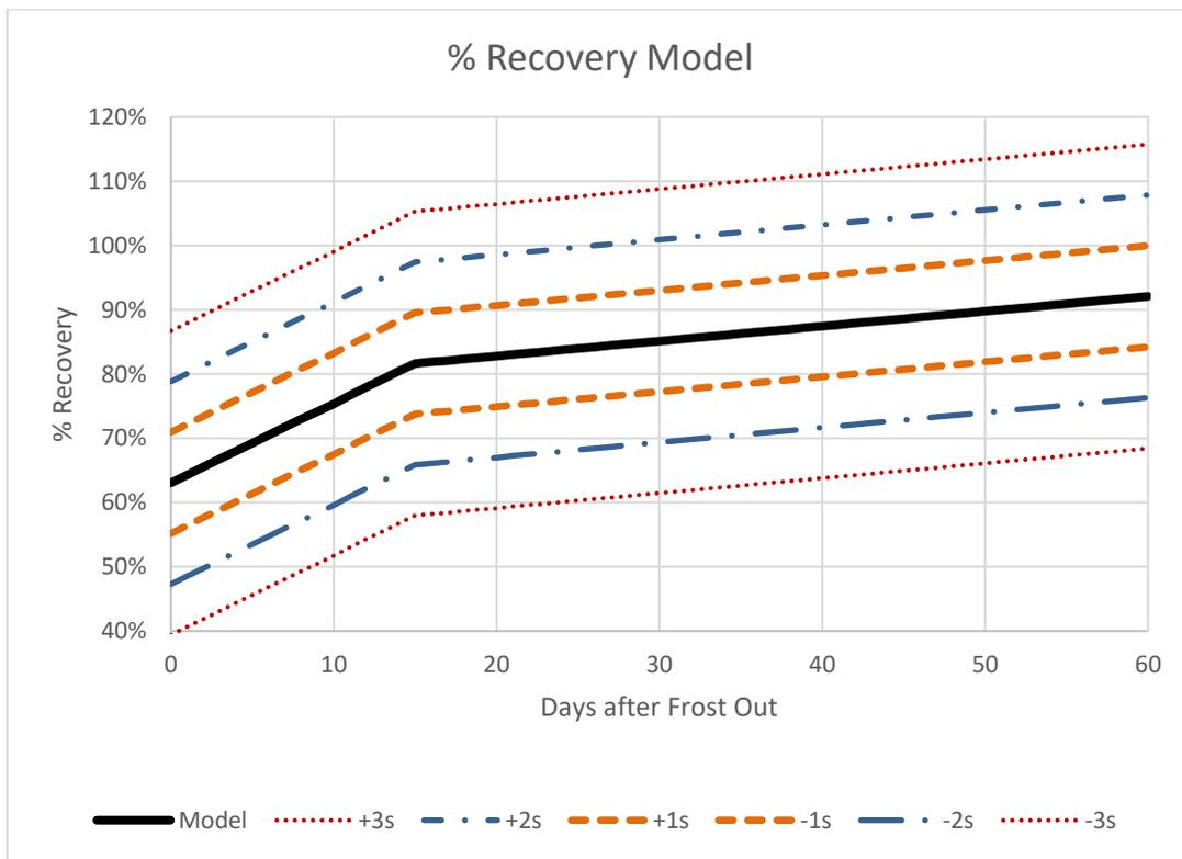
**Figure 34. Final model with  $\pm 3$  standard error bands with no data**
