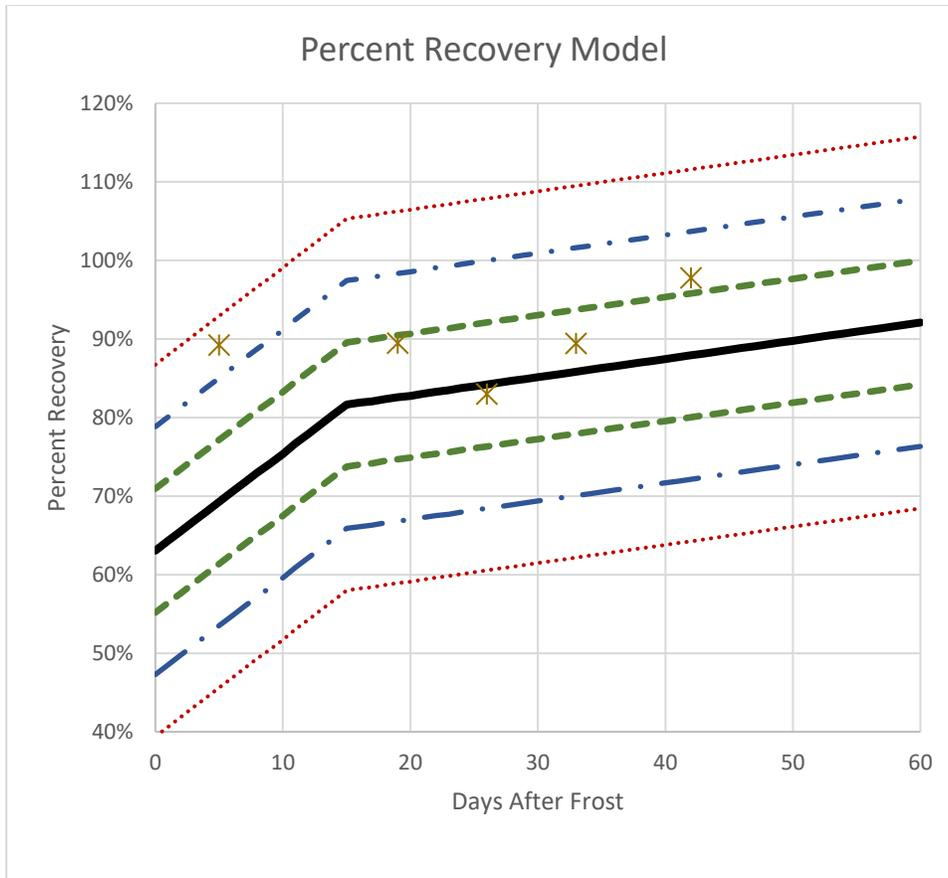
**Figure 44. Final model with  $\pm 3$  standard error bands with 2020 North Dakota Highway 8 data**
