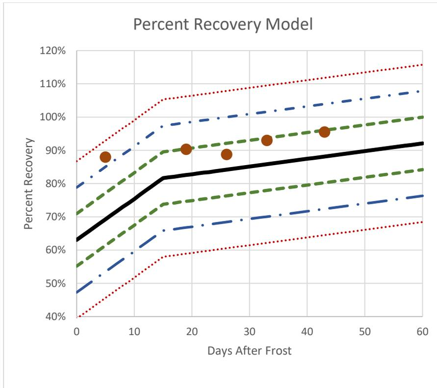
**Figure 43. Final model with  $\pm 3$  standard error bands with 2020 North Dakota Highway 6 data**
