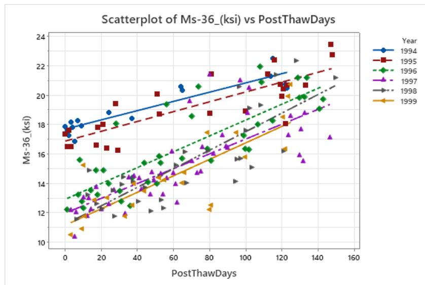
**Figure 15. Cell 26 Ms-36 0–150 days post frost 1994–1999 with yearly regression lines**
