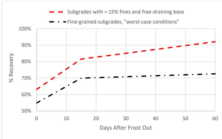
**Figure 23. Recommended model for roadways constructed on subgrades with more than 15% fines and free-draining base layers and recommended model for worst-case conditions**
