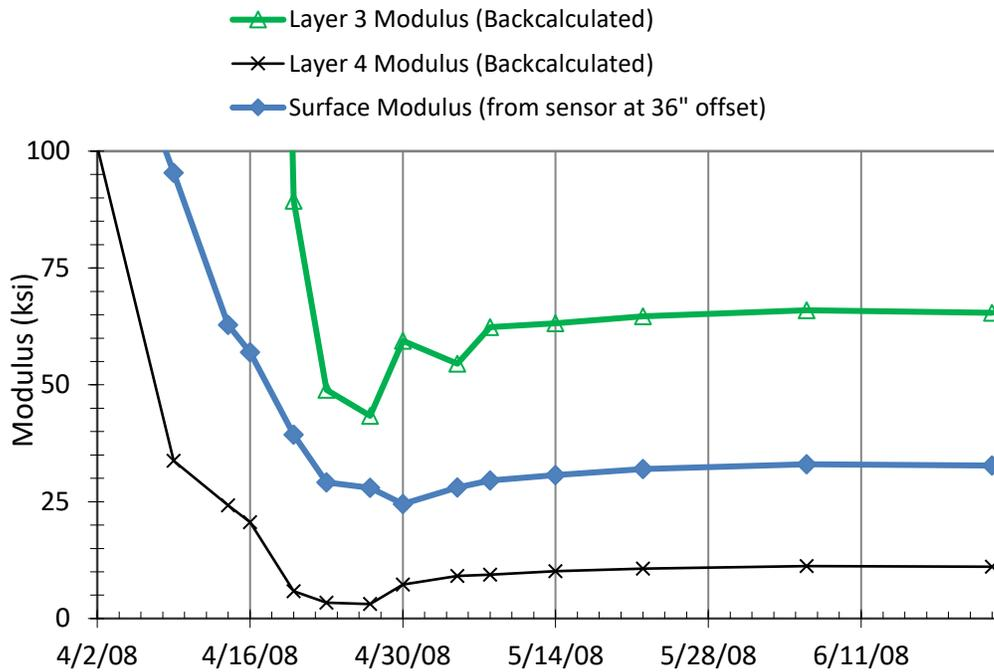
**Figure 27. Comparison of backcalculated modulus values with surface modulus values at Kancamagus Highway site**
