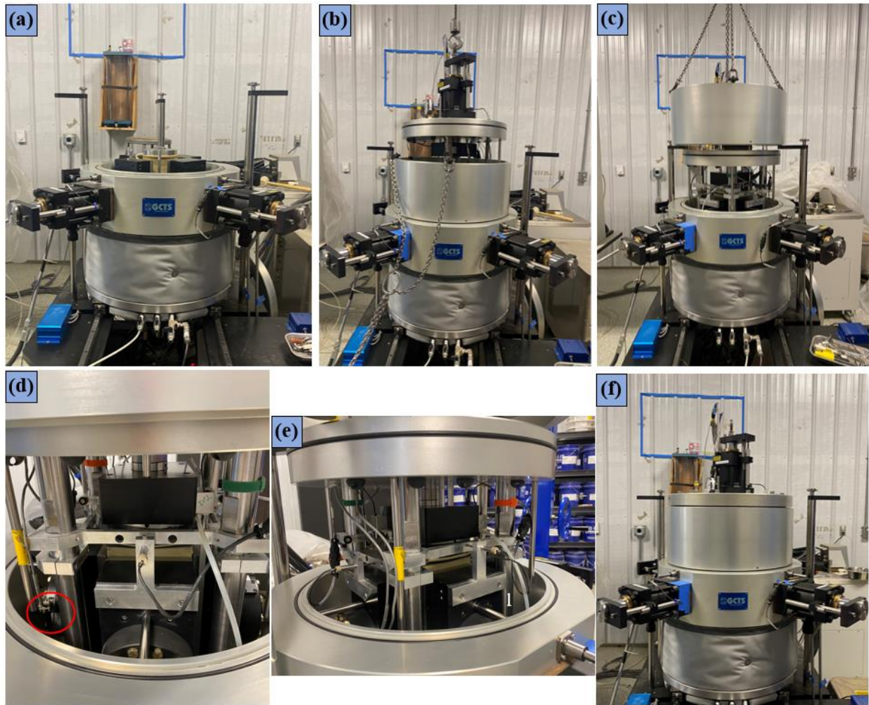
Figure 23. SPAX-3000 assembly process for prismatic specimen: (a) lower cell slid back, (b) placement of upper cell and top plate, (c) lifted upper cell, (d) load cell cable connection, (e) LVDT installation, (f) assembly completed
