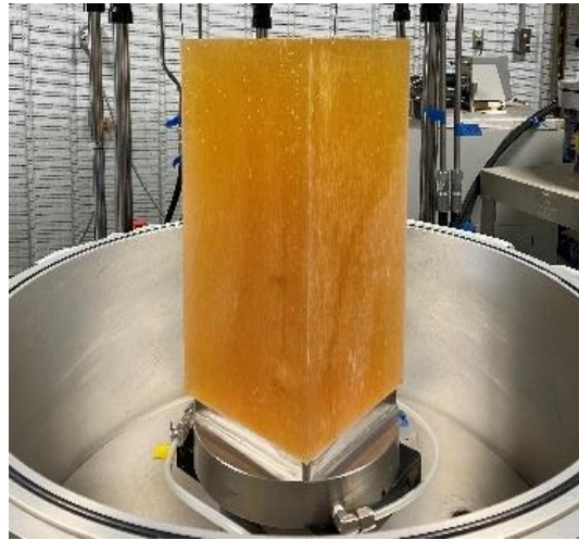
Figure 24. Prismatic isotropic urethane rubber sample
