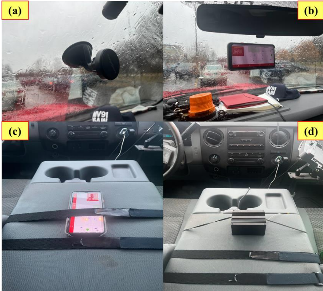
Figure 18. Alignment methods: (a) magnetic windshield mount, (b) smartphone mounted to the windshield, (c) smartphone banded to the center console, and (d) smart box banded to the center console
