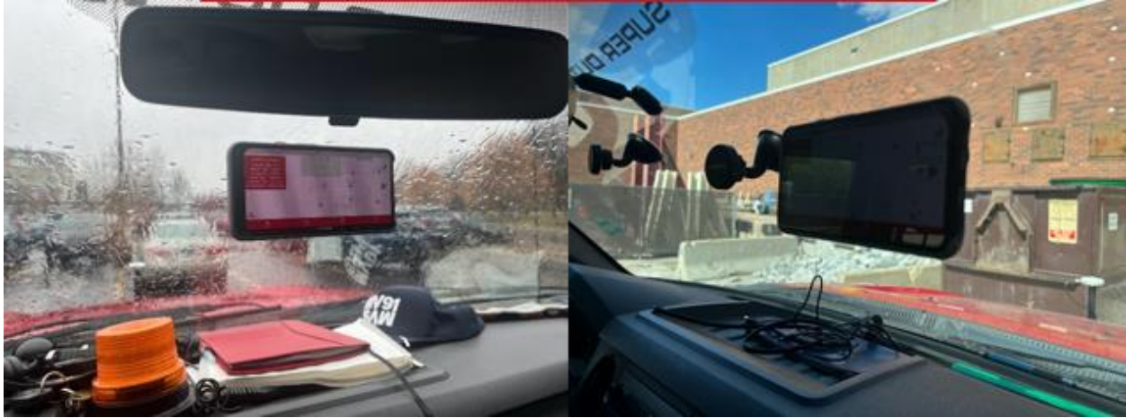
Figure A6. Mount mode using a ChargeWorx Dash and Windshield Magnetic Mount
