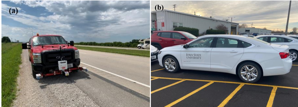
Figure 17. Vehicles used for data collection: (a) Ford F250 equipped with a high-speed profilometer and (b) 2018 Chevrolet Impala
