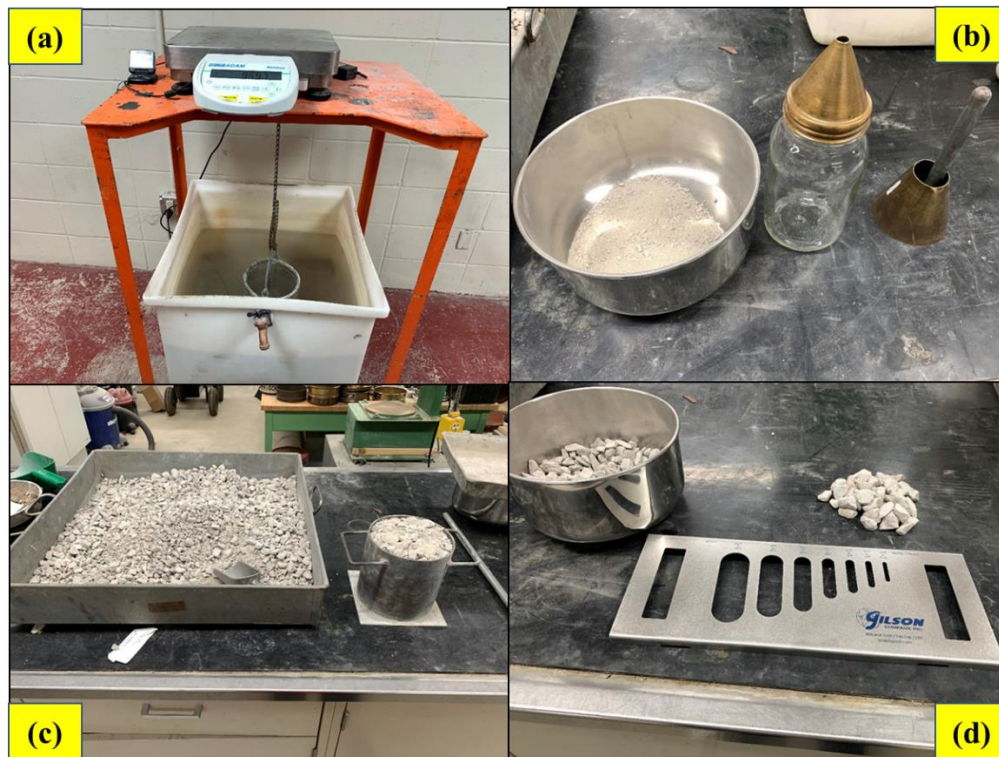
Figure A1. Required laboratory testing for determining (a) bulk specific gravity of aggregate coarse fraction, (b) bulk specific gravity of aggregate fine fraction, (c) voids in loose aggregate for particles larger than ½ in., and (d) average least dimension of aggregate
