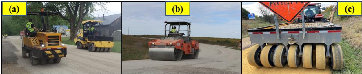
Figure A4. Rollers: (a) pneumatic-tired roller, (b) steel roller, and (c) fully loaded tractor
