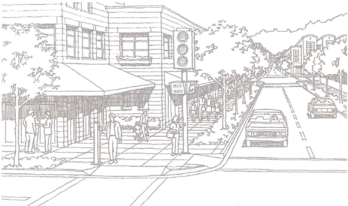
Figure 13. Pedestrian facilities include not only sidewalks, but curb ramps, crosswalks, traffic control devices, furnishings such as benches, and other amenities. Reprinted from Georgia Department of Transportation, p. 21.
