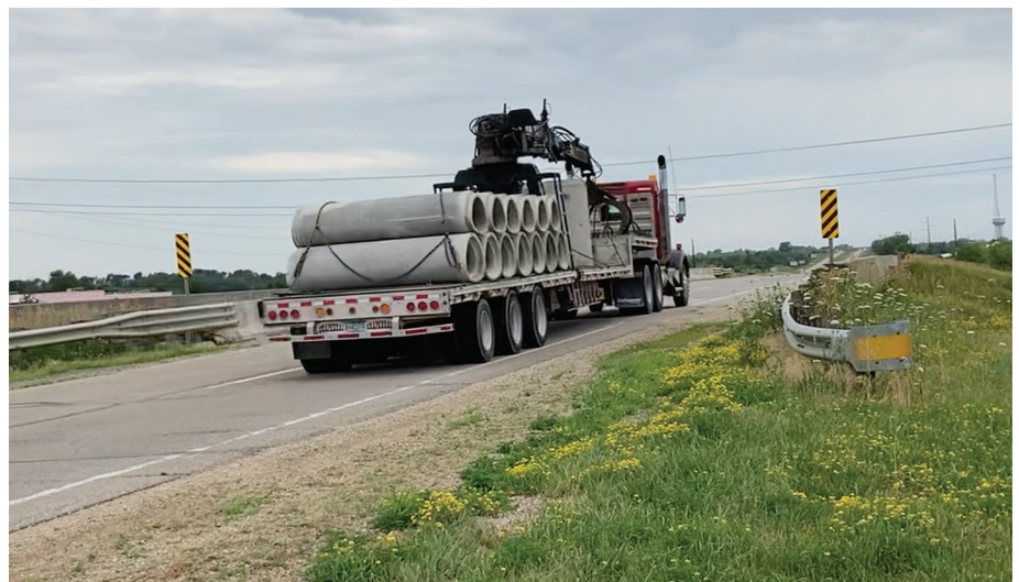
Truck event measuring bridge dynamic response subject to a live load on one of the bridges instrumented with strain gauges
