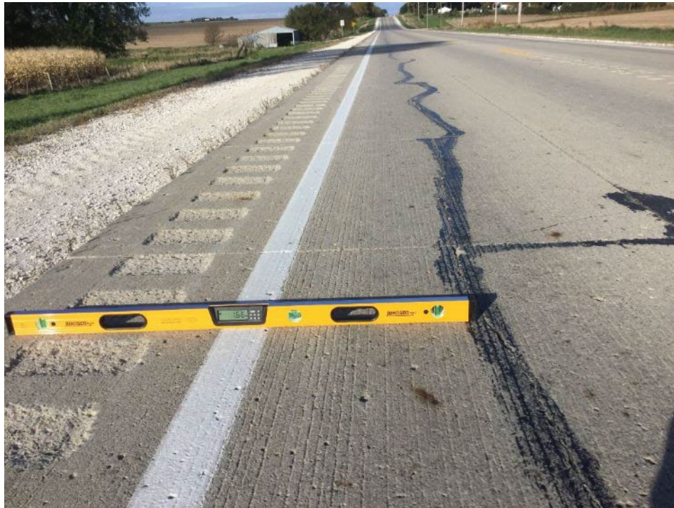
Figure 10 – Sac IA 175 UBOL Left Shoulder Crossslope 1.66%
