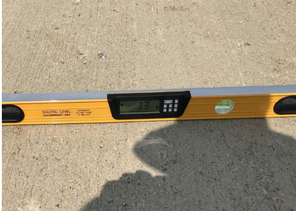
Figure 38 – Shoulder slope 3.3%, Paved 4%
