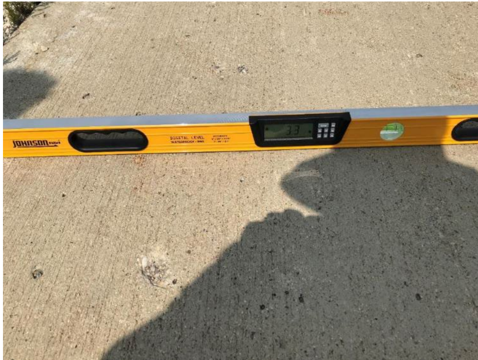
Shoulder cross slope 3.3%, Design 4%.
