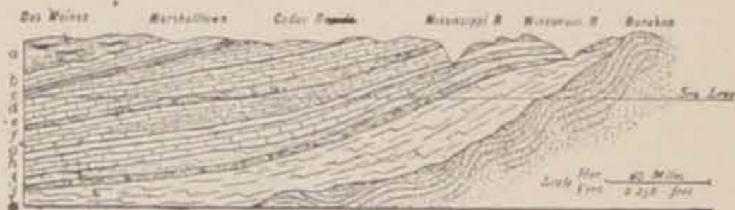
FIG. 1. Geological section from Baraboo, Wis., to Des Moines, Iowa, showing the general stratigraphy of the Iowa artesian area and of the Wisconsin gathering ground. The chief aquifers are the Saint Peter , the Jordan and the Basal sandstone . The line of juncture of the Basal sandstone and the Algonkian is hypothetical. a Des Moines; b Mississippi; c Kinderhook; d Devonian; e Silurian; f Hudson River; g Galena-Trenton; i Oneota; j Saint Croix; including the Jordan , St. Lawrence and Basal sandstone .
