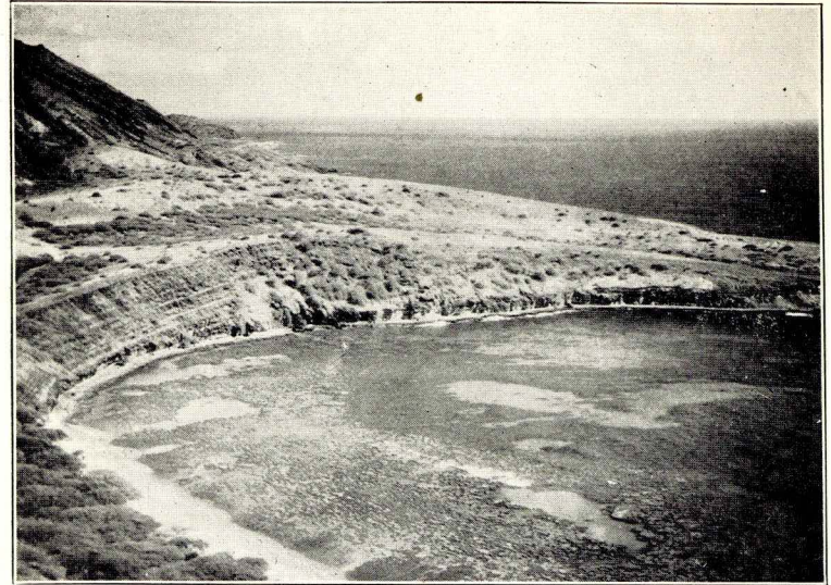
Fig. 7. View of Hanauma Bay, Koko Head region, Oahu, Hawaii. Taken with panchromatic film and orange (G) filter. The delineation of underwater reef detail over the entire area of the bay would be far less satisfactory without the filter and appropriate film.
