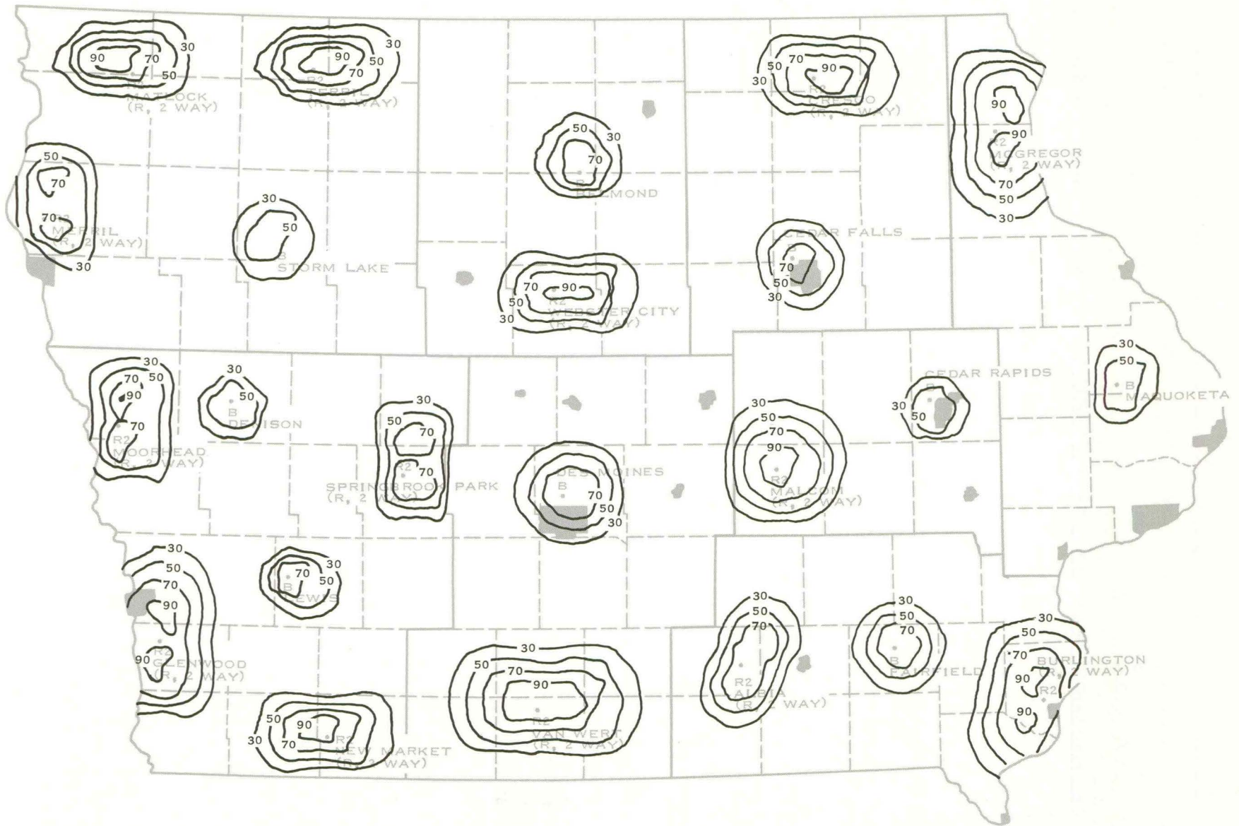
Figure 2-10. Type 1 Mobile to Base Service Probability Reduced by Severe Precipitation Static at Low Band.
