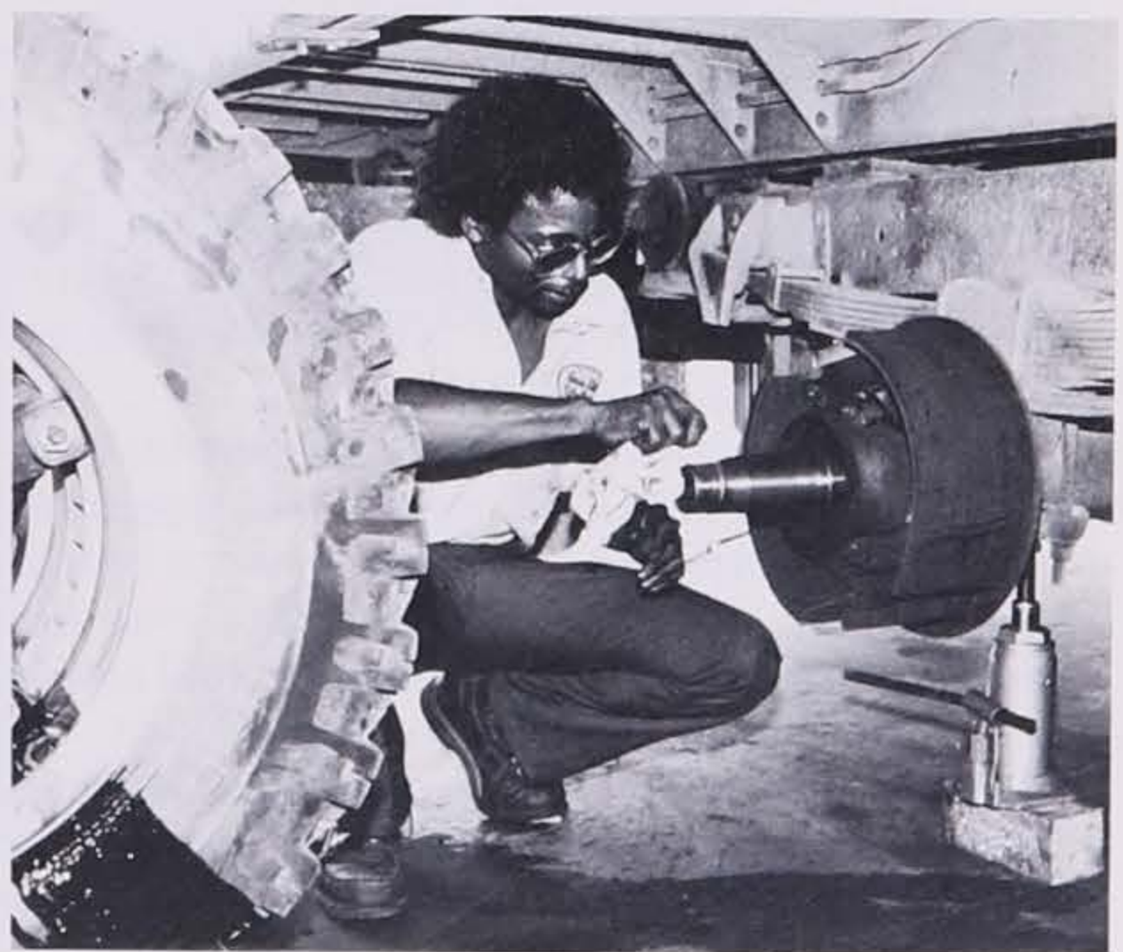
John Tate repairing the brakes on the GMC truck.
