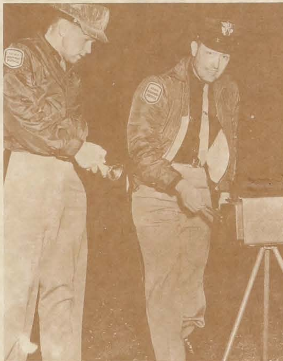
Patrolmen Orville Beaman and Wendell Stream are calibrating the radar for a night operation. This type of radar remained in one spot and the officer would have to leave the unit behind when pursuing and stopping a violator.
