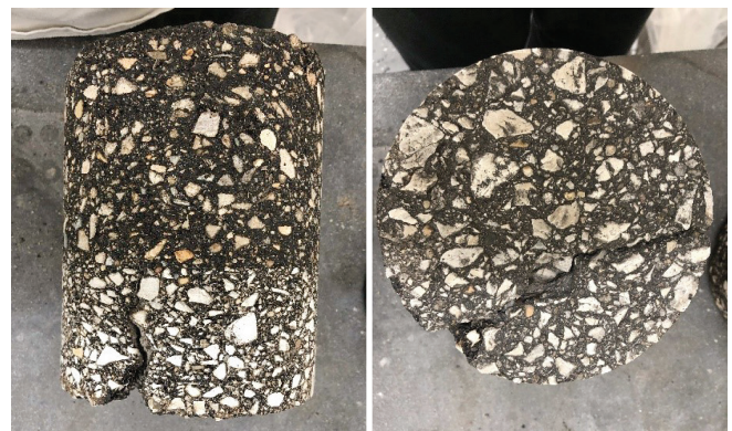
Side view (left) and top view (right) of a cracked core with an insufficient HMA layer thickness
