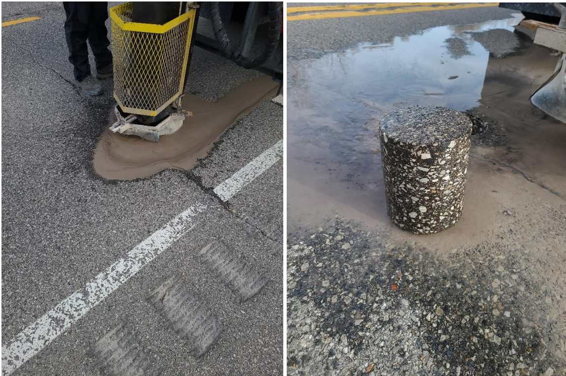
Figure 3-1. Process of collecting cores from US 34
