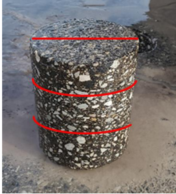
Figure 3-2. Cuts made to prepare a semicircular specimen with a thickness of 50 mm
