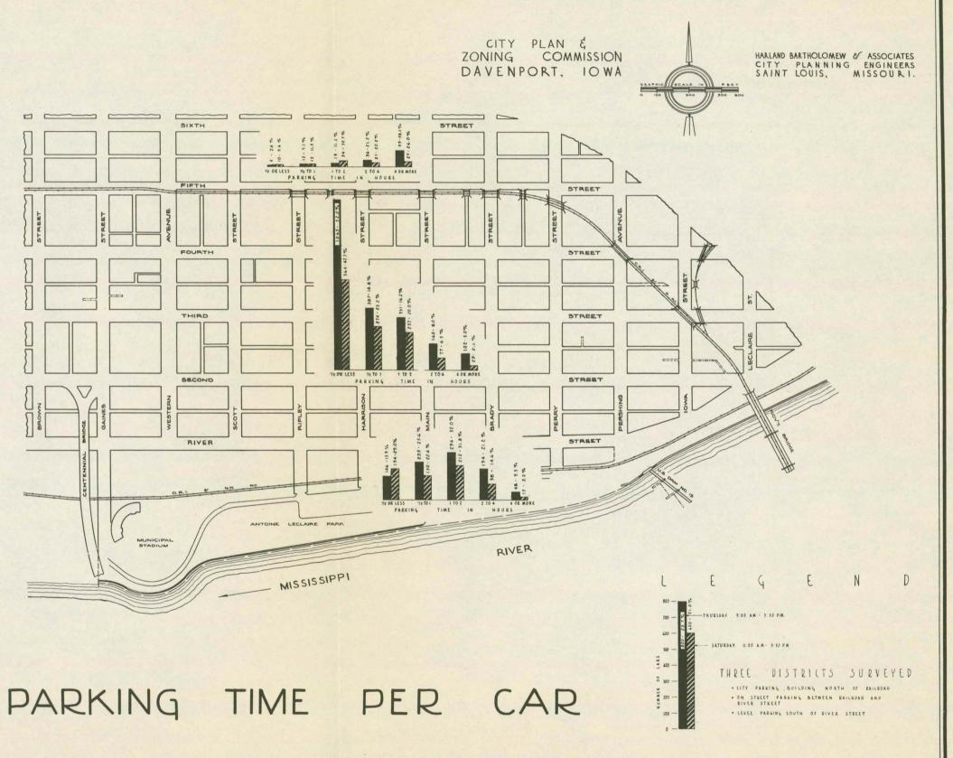
The number and proportions of cars parked for the different periods of time are graphically indicated on Plate 4, based on the parking survey. The parking durations shown at the top of this map relate to the new city parking garage north of the Rock Island Railroad and those at the bottom to the LeClaire and Levee lots south of River Street; the central chart indicates the utilization of representative curb parking facilities in the area between the Rock Island Railroad and River Street.
