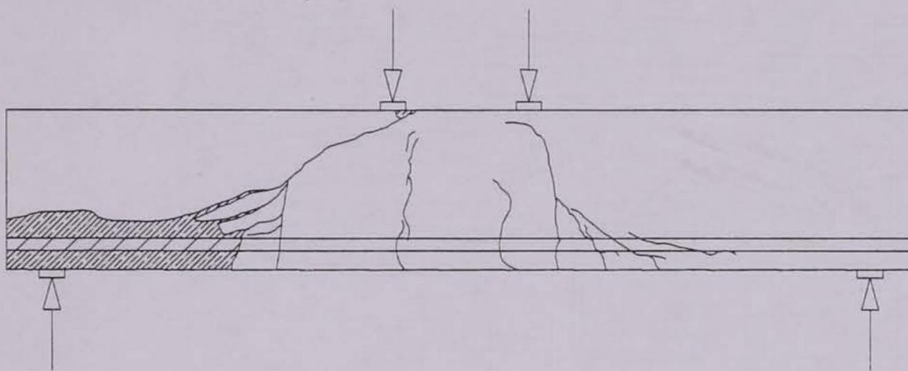
Figure 6a – Crack pattern for FRP 1. Typical crack pattern for the FRP-normal series.
