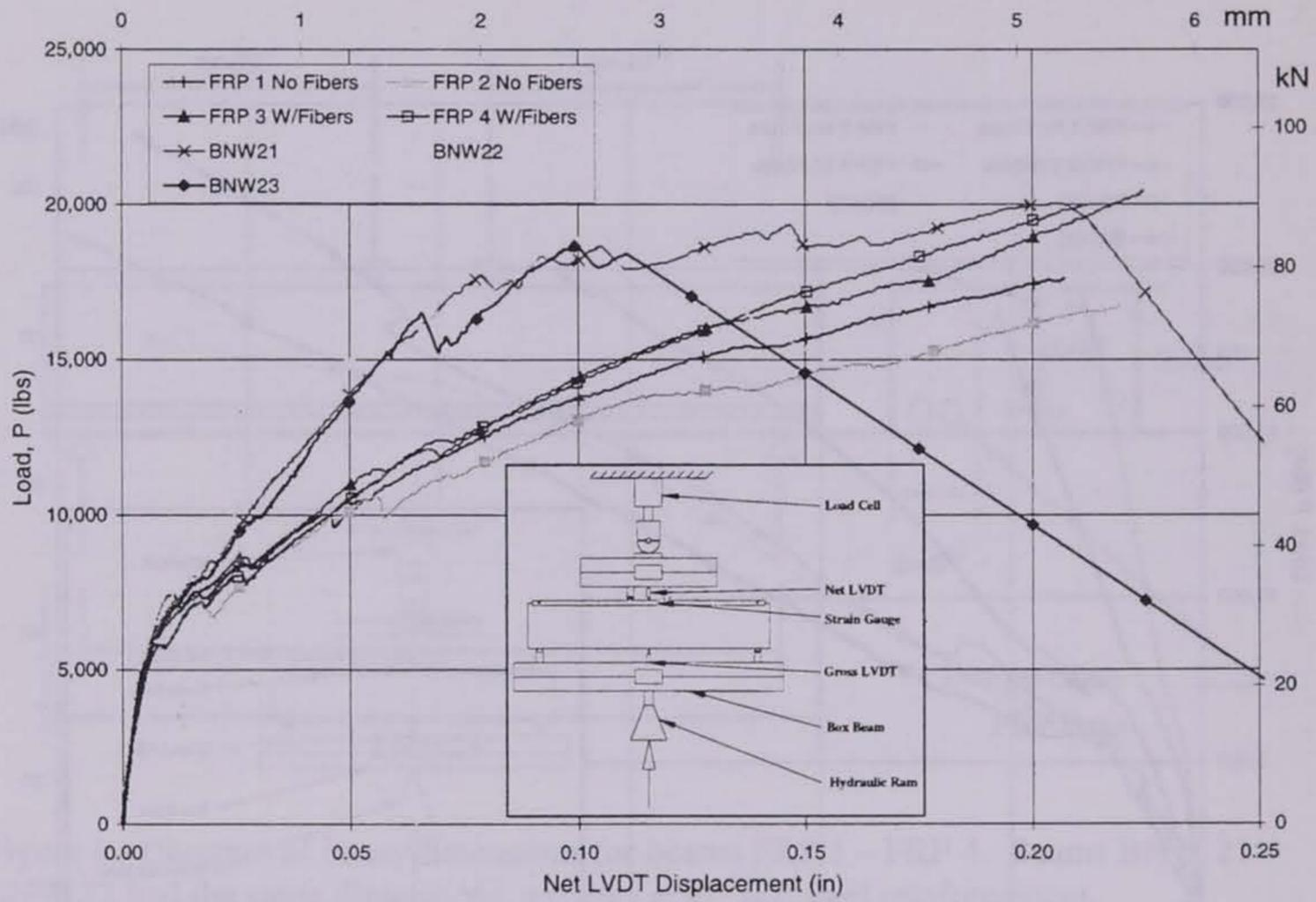
Figure 4 – Comparison of the load vs net-deflection response for FRP 1 – FRP 4 and BNW 21 - BNW 23.
