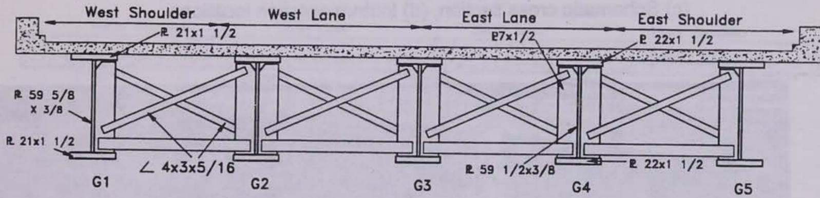
(c) Schematic cross section
