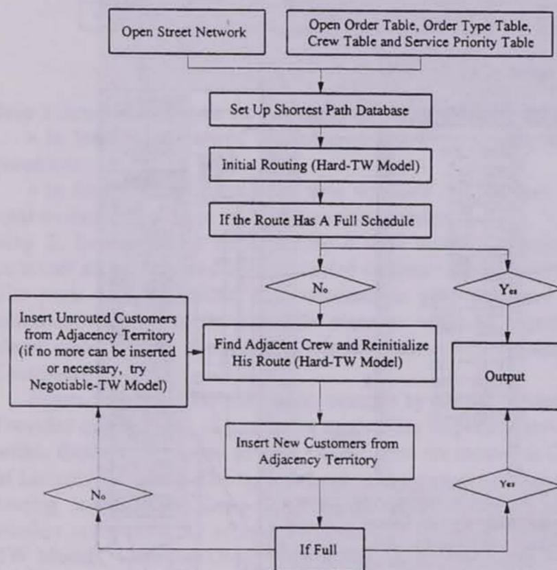
Figure 2-4. Flowchart of Procedure Designed for Division-Duty Model
