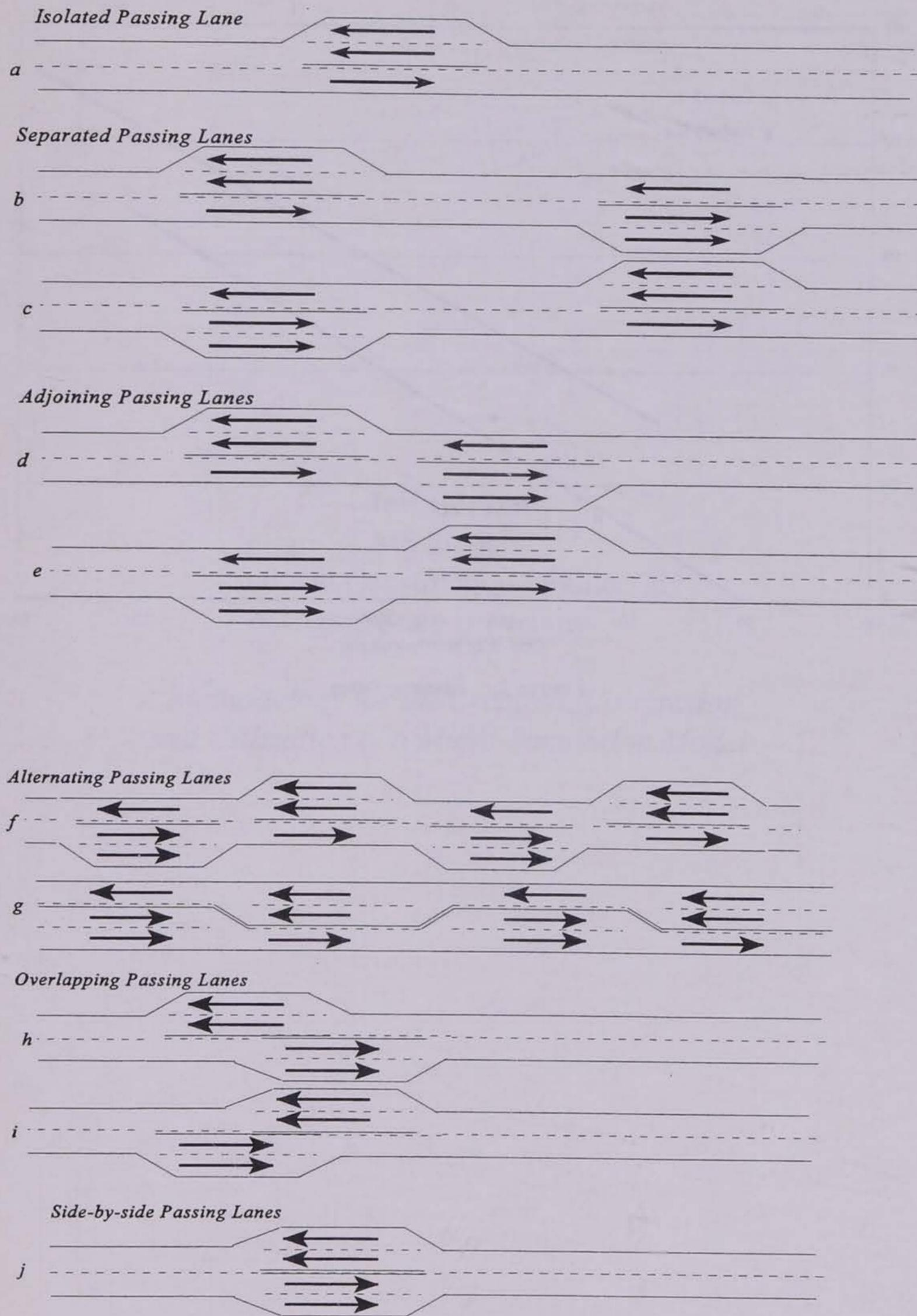
Figure 1: Passing Lane Configurations. Source: (8)
