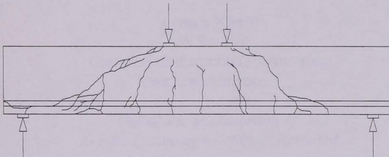
Figure 6b – Crack Pattern for FRP 4. Typical crack pattern for the FRC-FRP series.
