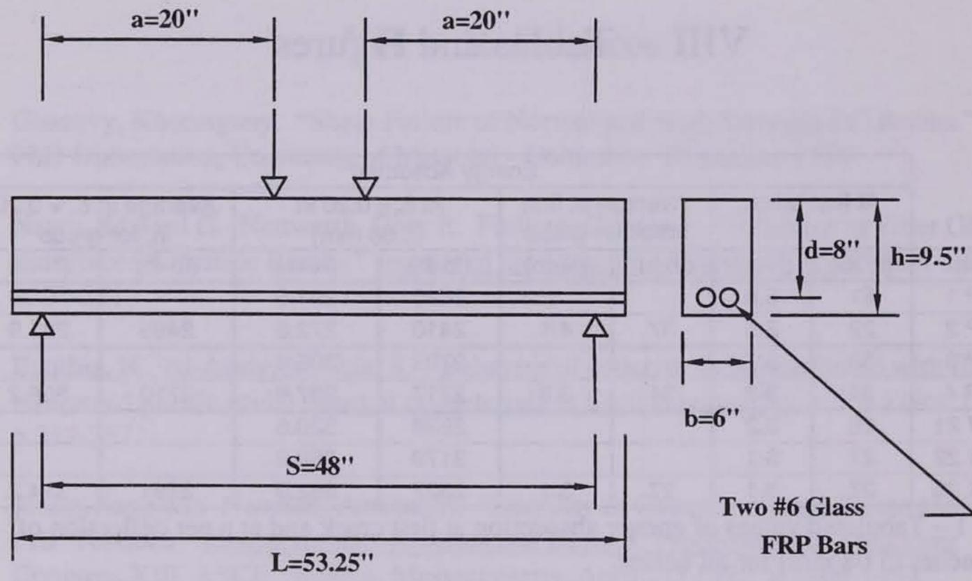
Figure 1 - Diagram of beam dimensions for beams FRP 1 – FRP 4. Beams BNW 21 – BNW 23 had the same dimensions, except  $L=56''$  and steel reinforcement.
