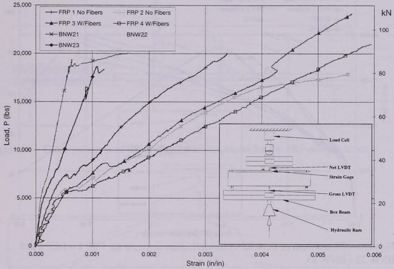
Figure 3 – Comparison of the load vs concrete compressive strain response for FRP 1 – FRP 4 and BNW 21 – BNW 23.
