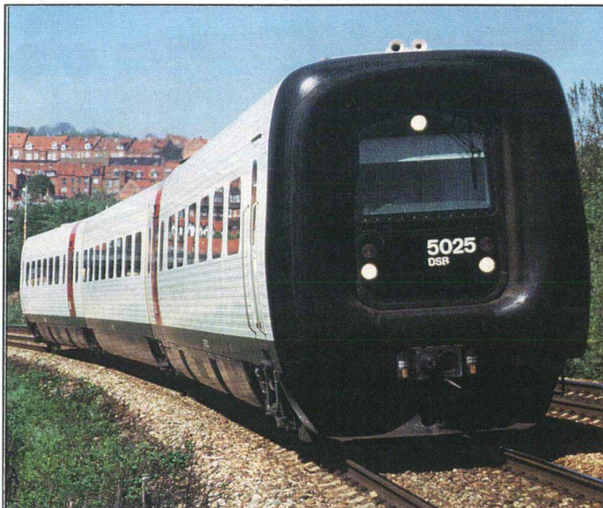
Exhibit 6-17 Type IC3D Flexliner as built by ABB Skandia
