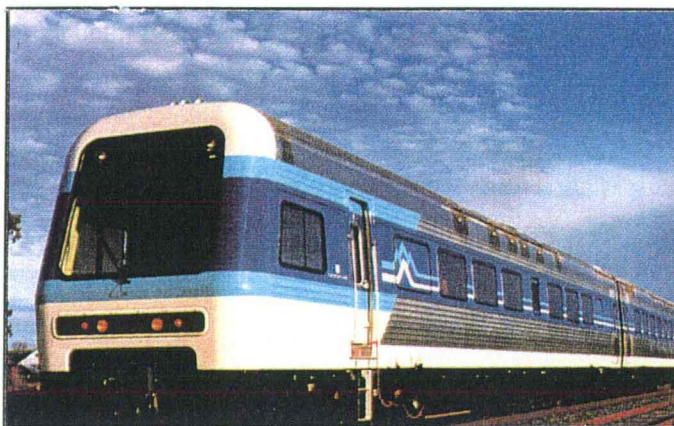
Exhibit 6-16 DMU Type Xplorer for New South Wales State Rail Authority as built by ABB Transportation
