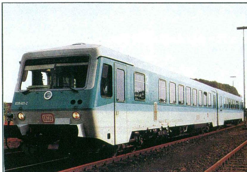
Exhibit 6-18 Type 628 as built by Siemens Duewag
