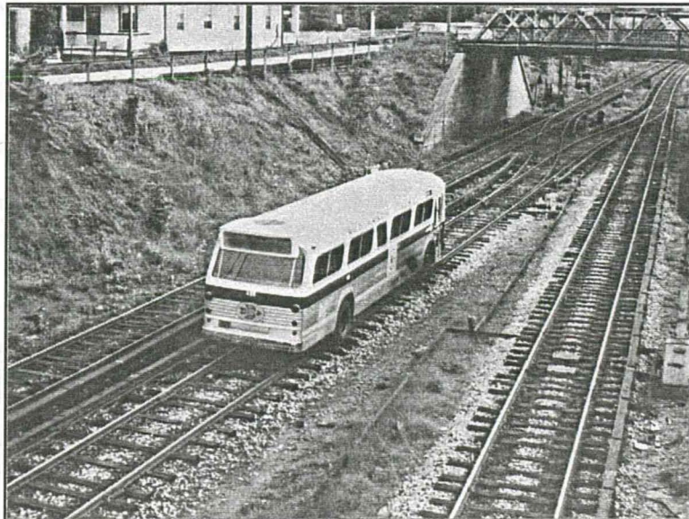
Exhibit 6-13 Red Arrow "railbus"
