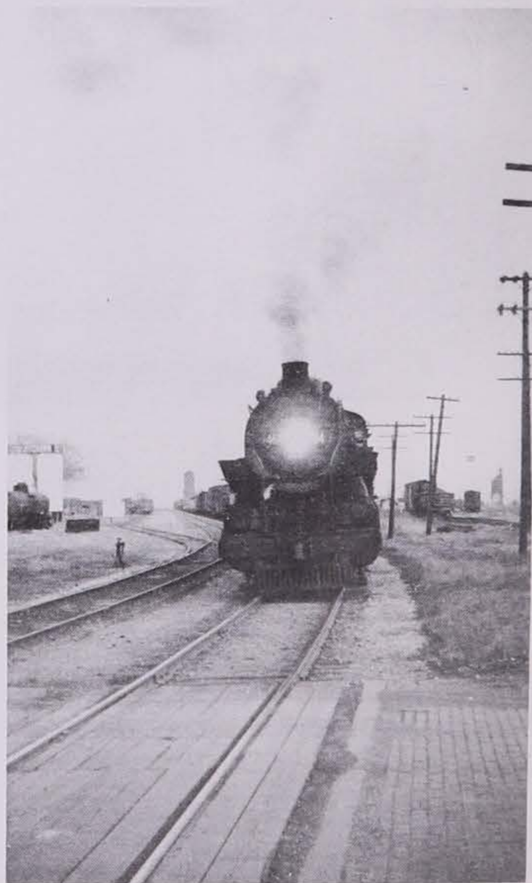
Milwaukee No. 484 a 2-8-2 westbound local freight Washington. Both coal chutes are shown in background. North 4th Ave. 1948.
