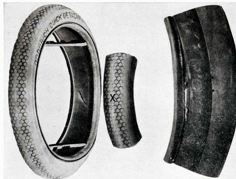
A clean break in the fabric resulting from hitting an obstruction with tire underinflated. —Courtesy Goodrich.
