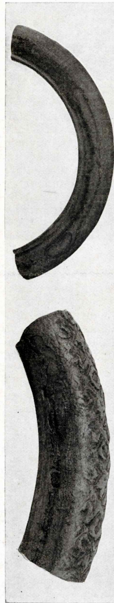
Running in ruts destroys the side wall of the casing. —Courtesy Goodrich and Firestone
