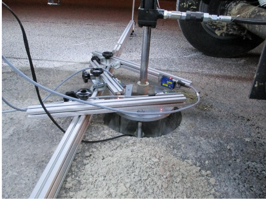
Figure 19. 12 in. diameter loading plate setup for cyclic APLT to measure resilient modulus values under an existing pavement in a core hole
