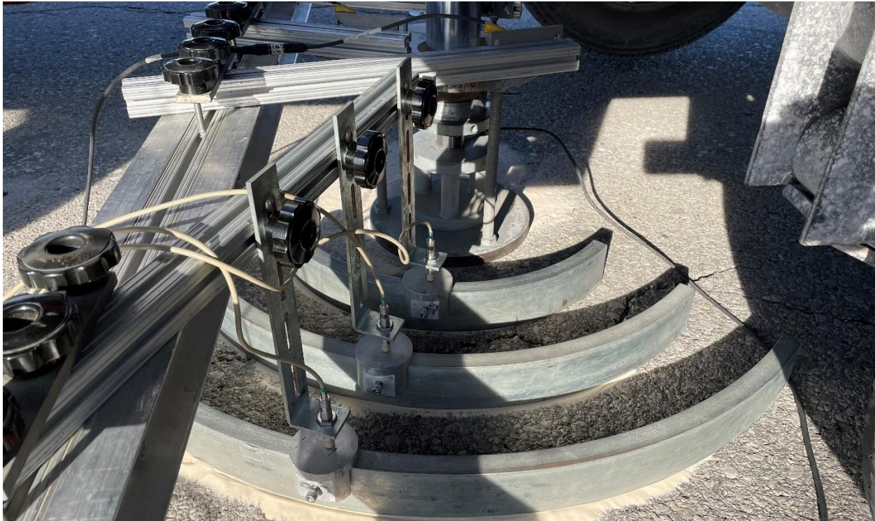
Figure 22. 12 in. diameter loading plate setup with layered analysis sensor kit on asphalt pavement surface
