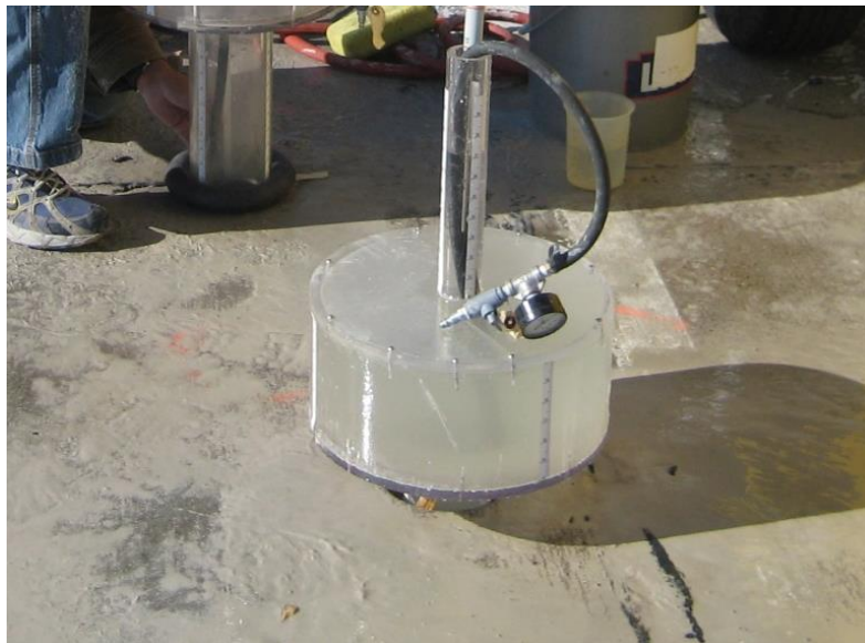
Figure 26. Core hole permeability testing under PCC pavement
