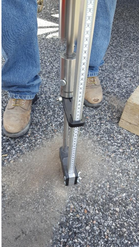
Figure 27. DCP test through a 1 in. diameter hole in the pavement layer
