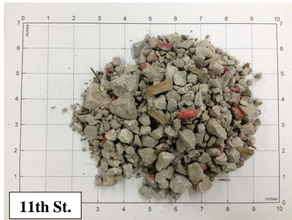
Figure 8. Modified subbase samples collected from the three test sections after construction (July 2012)
