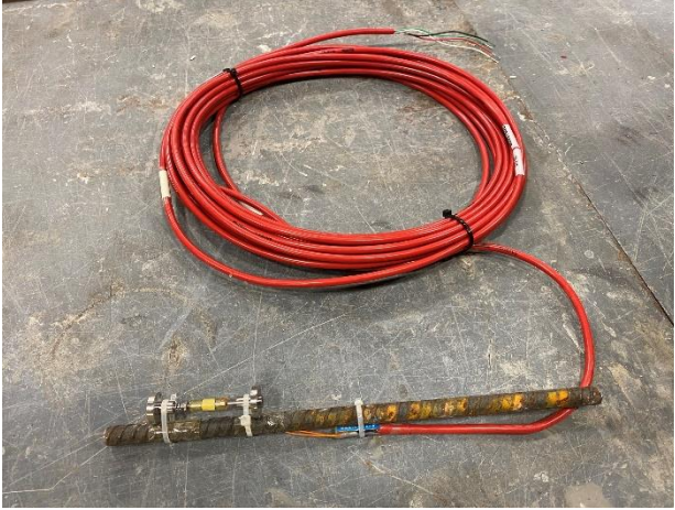
(a) Strain gauge attached to a piece of rebar
