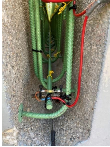
(a) Strain gauge placed at the top of a joint (b) Strain gauge placed at the bottom of a joint
