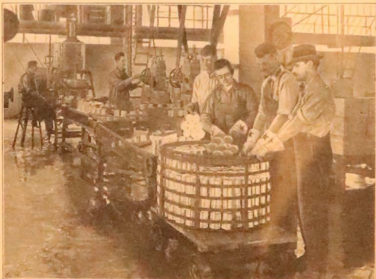
FIG. 72. The man at the farther end of this picture is soldering on the lids of the cans, which are then packed in a crate to be placed in the big steam cookers shown in Fig. 73. (Photograph by Hostetler)
