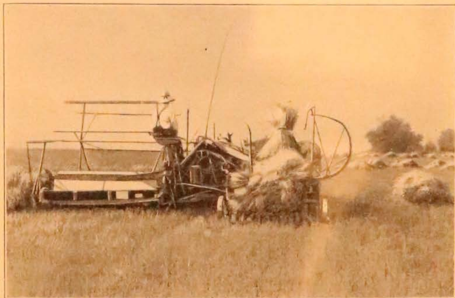
FIG. 57. With the aid of this machine, which cuts, binds, and shocks the grain, one man with a team does the work that formerly required several men and teams. Tractors are often used instead of horses in operating these machines (see Fig. 58). (Courtesy of International Harvester Company)
