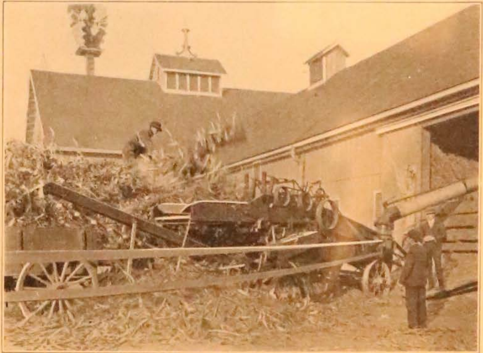
FIG. 60. A combined husker and shredder. Is this corn ripe or green? Give two proofs for your answer. (Courtesy of Iowa State Agricultural College)
