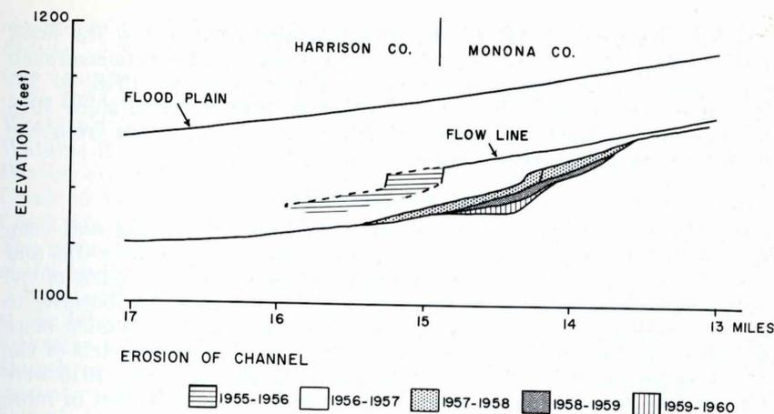
Figure 28.—Changes in the Willow drainage ditch since 1955.
