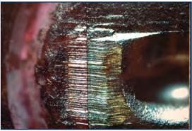
Above: side-by-side microscopic comparison of breech face marks on cartridge casings caused by shearing against the firing pin aperture.
