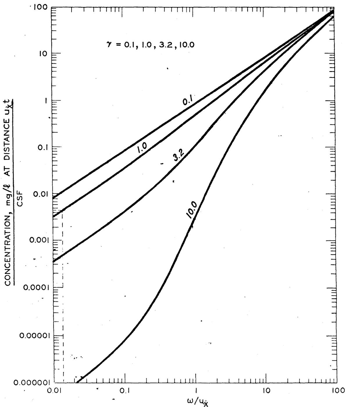
Figure 5-1. Relationship between  $\omega/u_x$  and  $\frac{\text{Solids concentration at distance } X}{\text{CSF}}$  for  $\gamma = 0.1, 1, 3.2$  and  $10$ .
