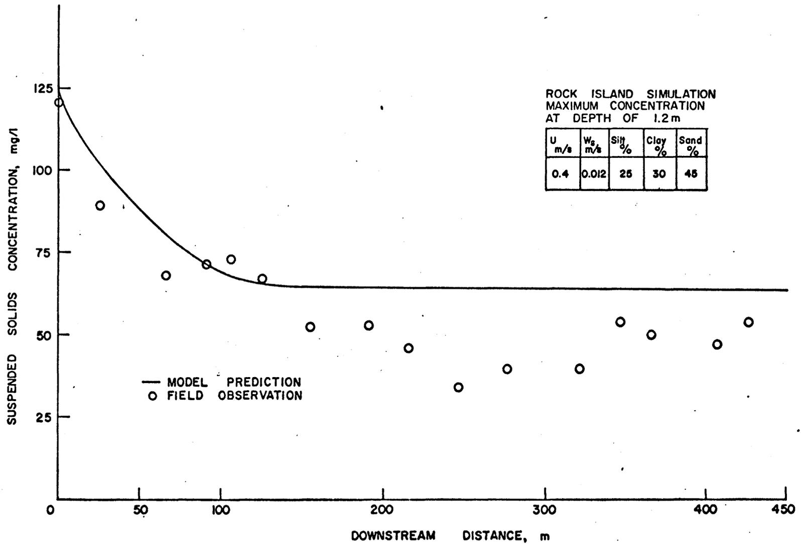
Figure 6-13. Line of maximum sediment concentration at depth of 1.2 m - Rock Island, Illinois.
