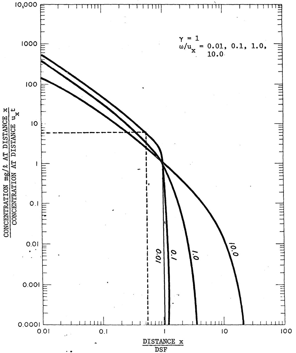
Figure 5-2. Relationship between  $\frac{\text{Distance } x}{\text{DSF}}$  and  $\frac{\text{Solids concentration at distance } x}{\text{Solids concentration at distance } u_x t}$  for  $\omega/u_x$  equal to 0.1, 1, and 10, and  $\gamma = 1$ .
