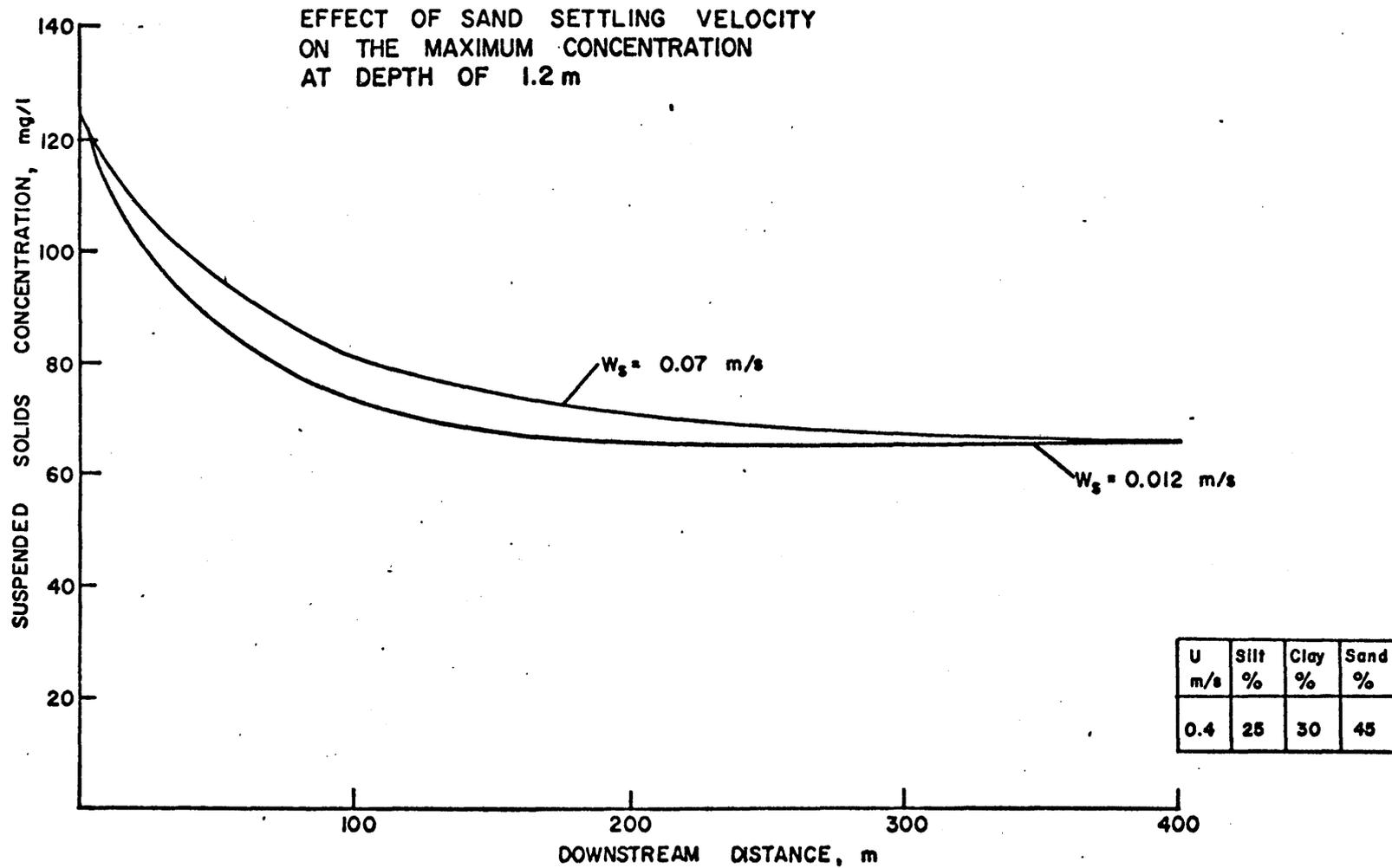
Figure 6-14. Effect of sand settling velocity on maximum concentration at depth of 1.2 m - Rock Island, Illinois.
