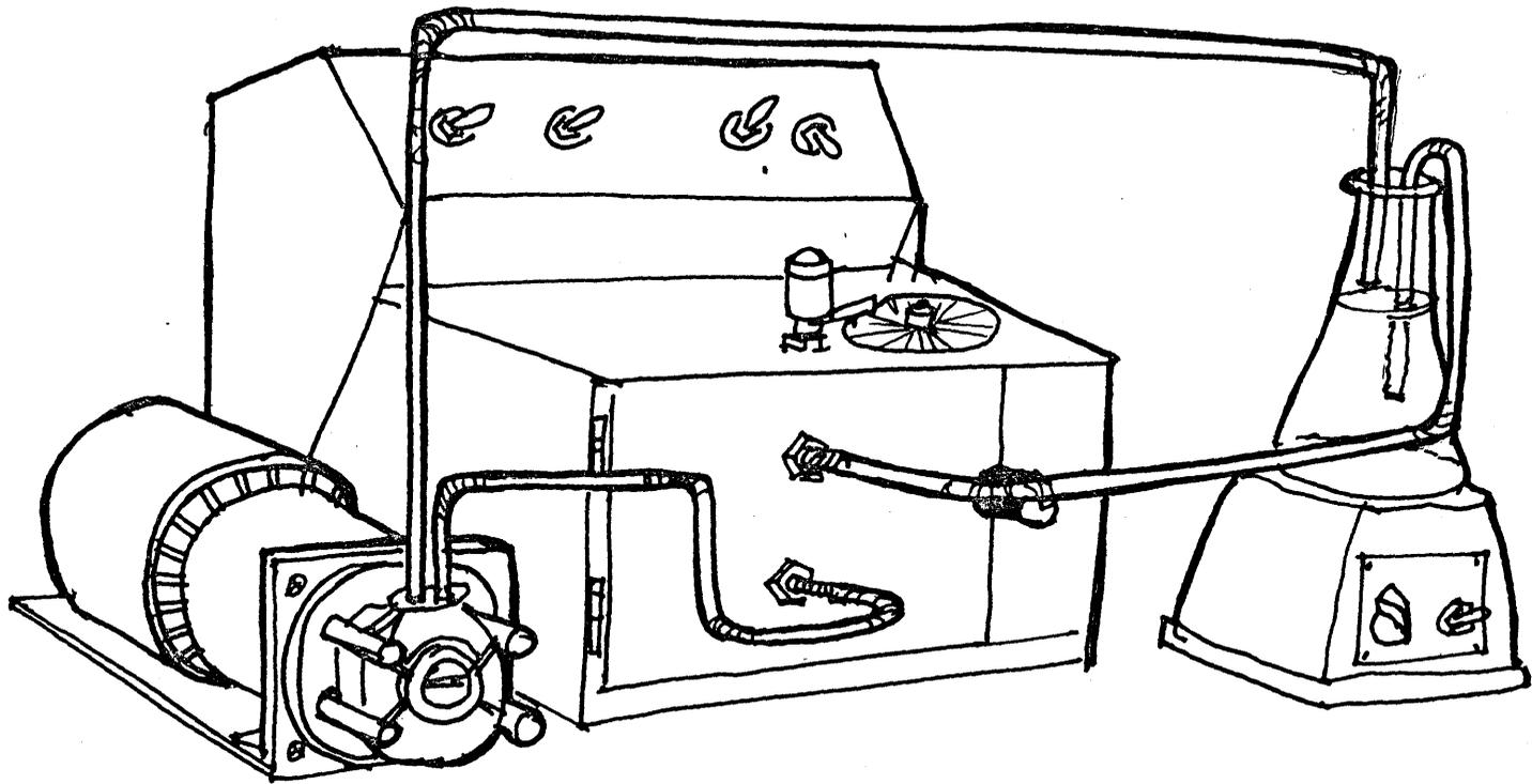
Figure 4-1. Experimental apparatus used to develop turbidity vs. suspended solids relationships.
