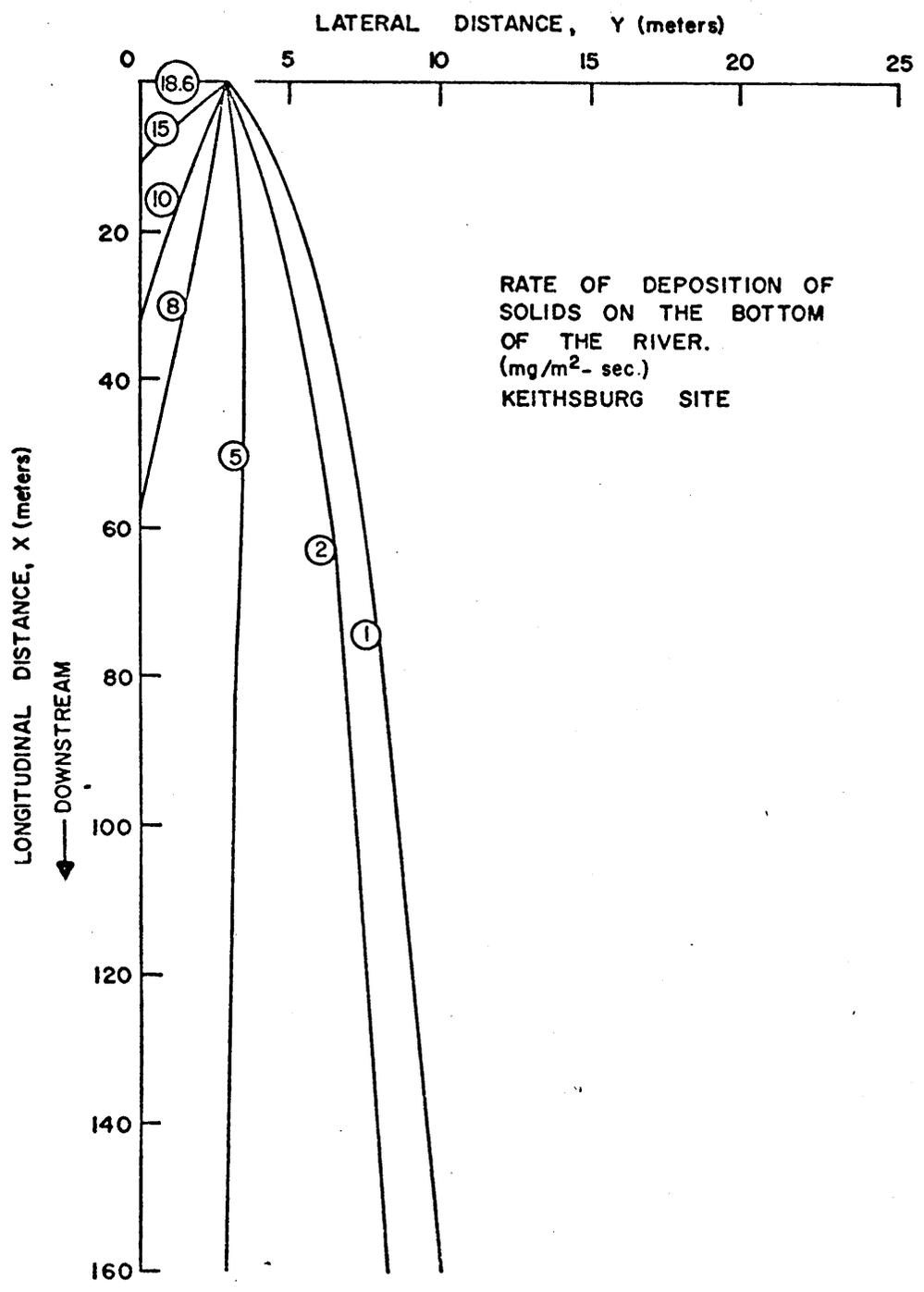
Figure 5-14. Deposition rate at all points in plume for Keithsburg, Illinois.
