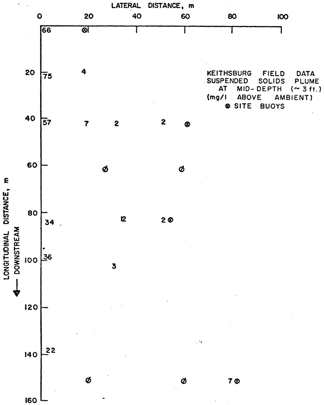
Figure 4-7. Mid-depth suspended solids plume at Keithsburg, Illinois site.
