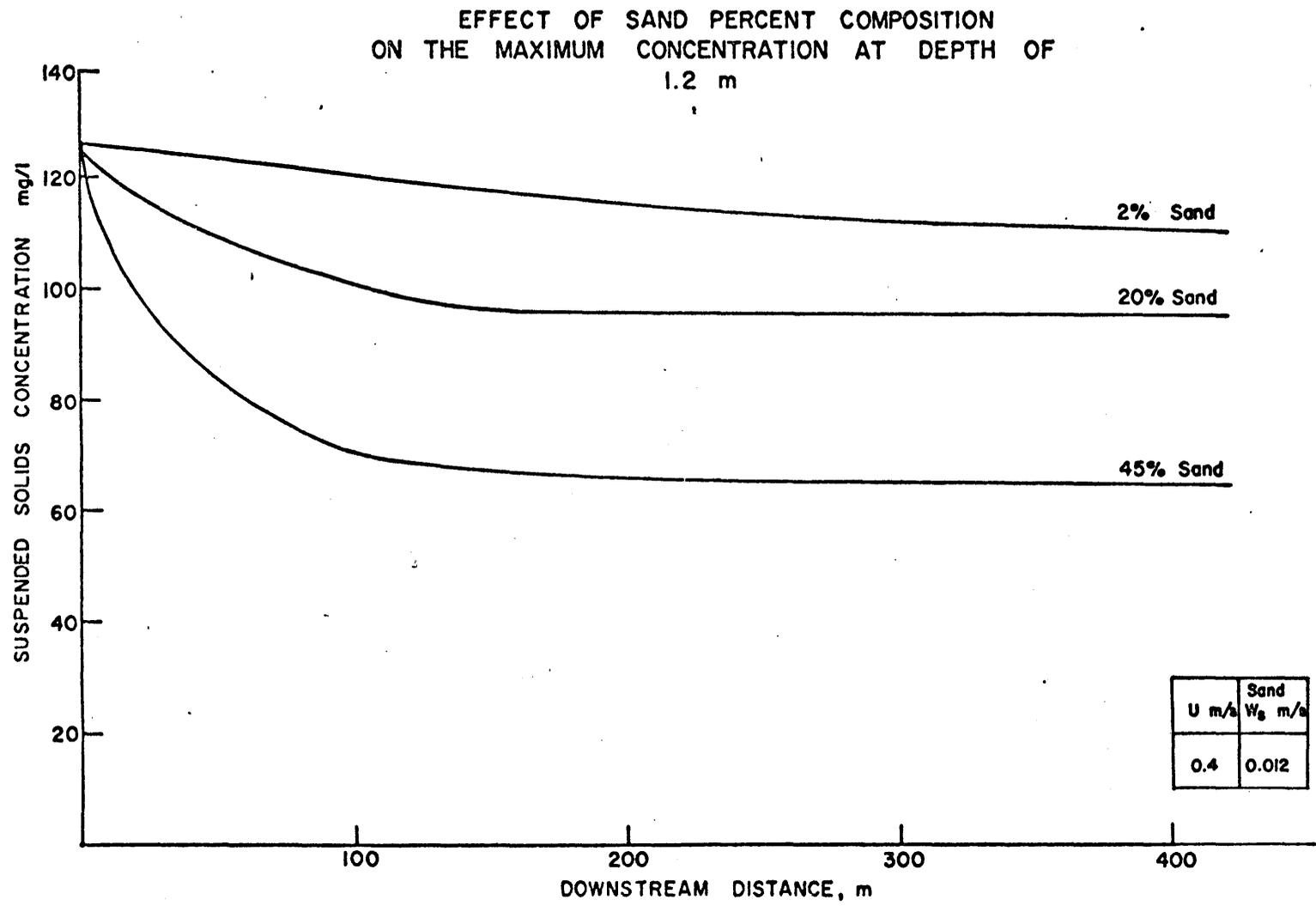
Figure 6-15. Effect of amount of sand in the sediment on maximum concentration at depth of 1.2 m - Rock Island, Illinois.
