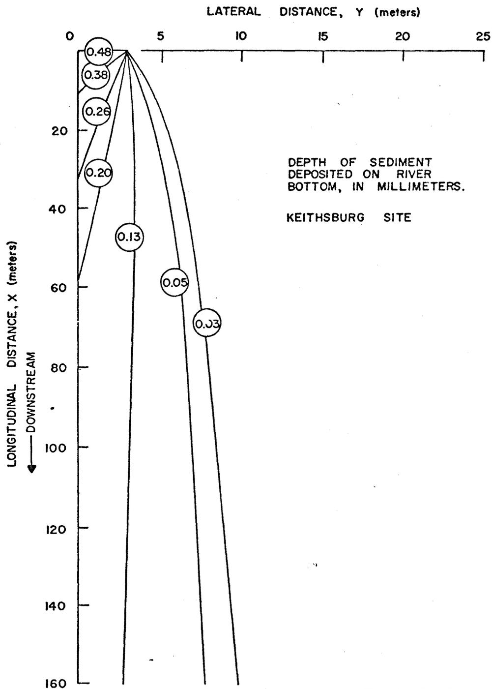
Figure 5-16. Depth of sediment deposited from plume at Keithsburg, Illinois, mm.
