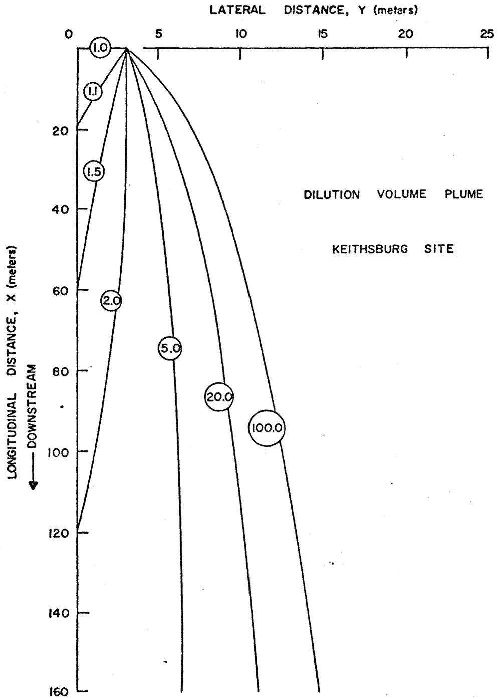
Figure 5-18. Dilution volume at points in plume, Keithsburg, Illinois.
