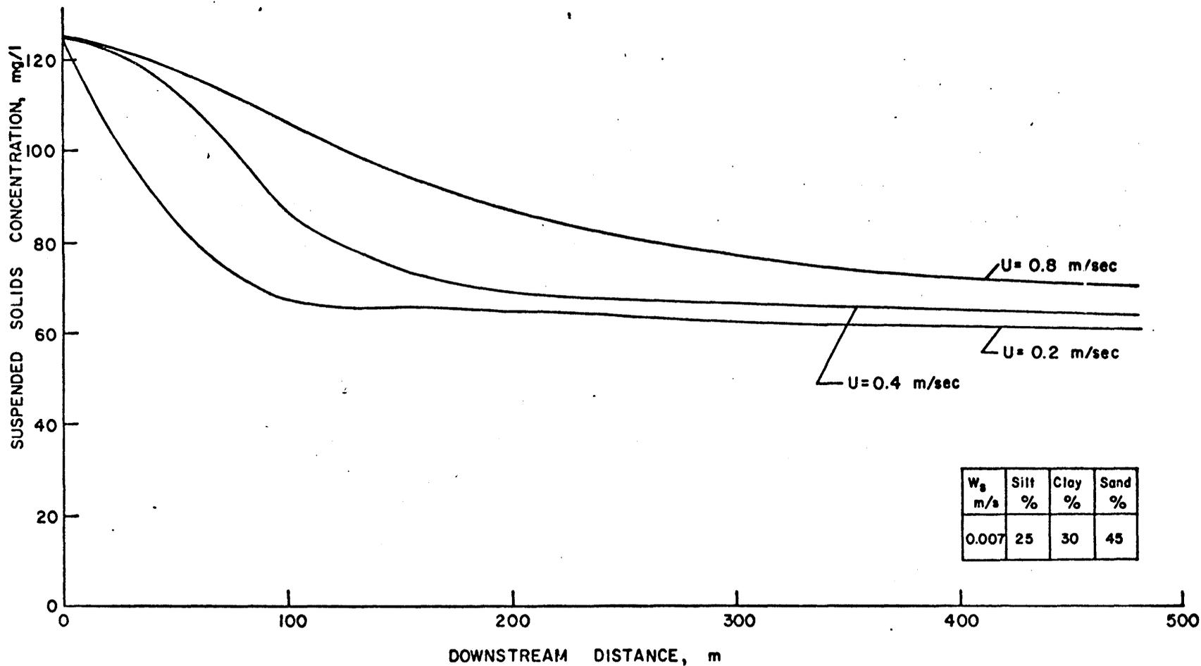
Figure 6-16. Effect of river velocity on maximum concentration at depth of 1.2 m - Rock Island, Illinois.
