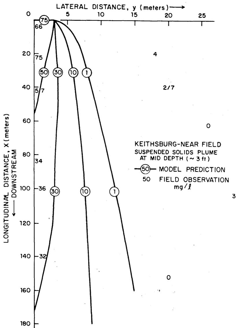
Figure 5-8. Simulated suspended solids plume for Keithsburg, Illinois site superimposed on field data.
