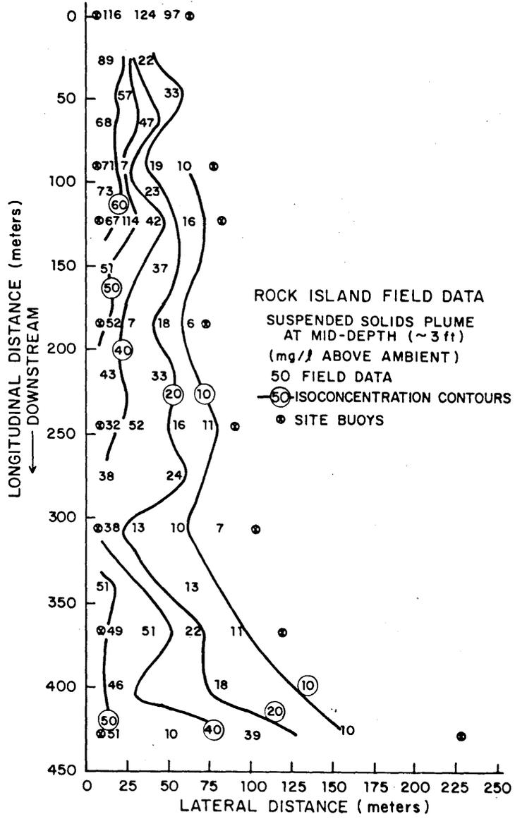
Figure 4-8. Mid-depth suspended solids plume at Rock Island, Illinois site.
