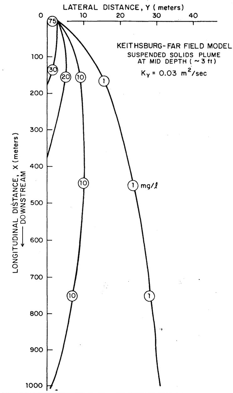
Figure 5-9. Far field suspended solids plume for Keithsburg, Illinois site.  $K_Y = 300 \text{ cm}^2/\text{sec}$ .
