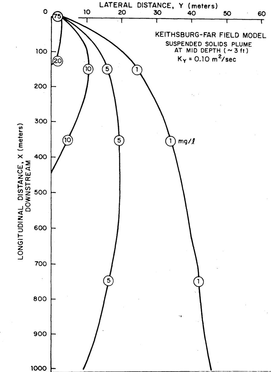
Figure 5-10. Far field suspended solids plume for Keithsburg, Illinois site.  $k_y = 1000 \text{ cm}^2/\text{sec}$ .
