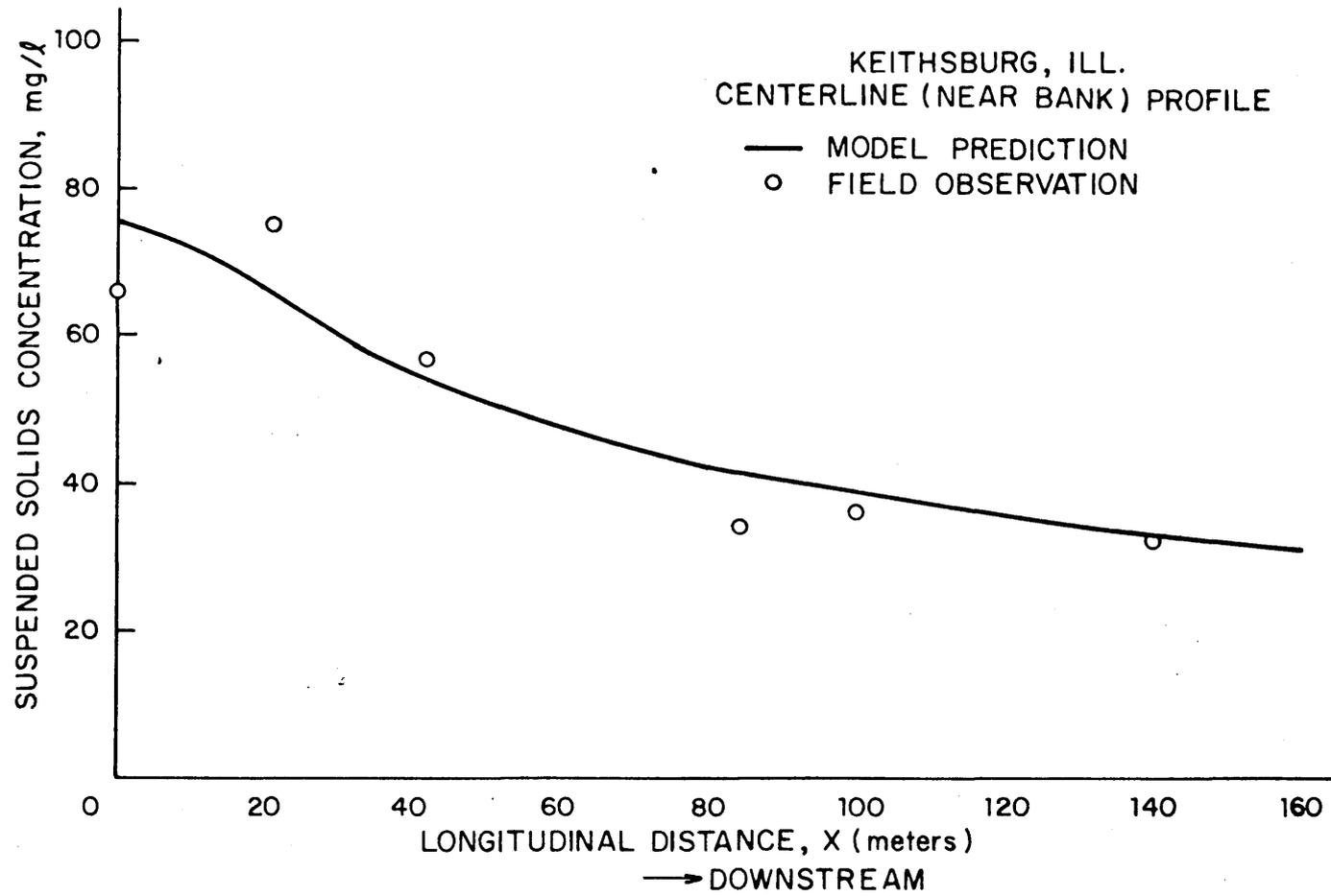
Figure 5-12. Model prediction vs. field observation for centerline Keithsburg site.
