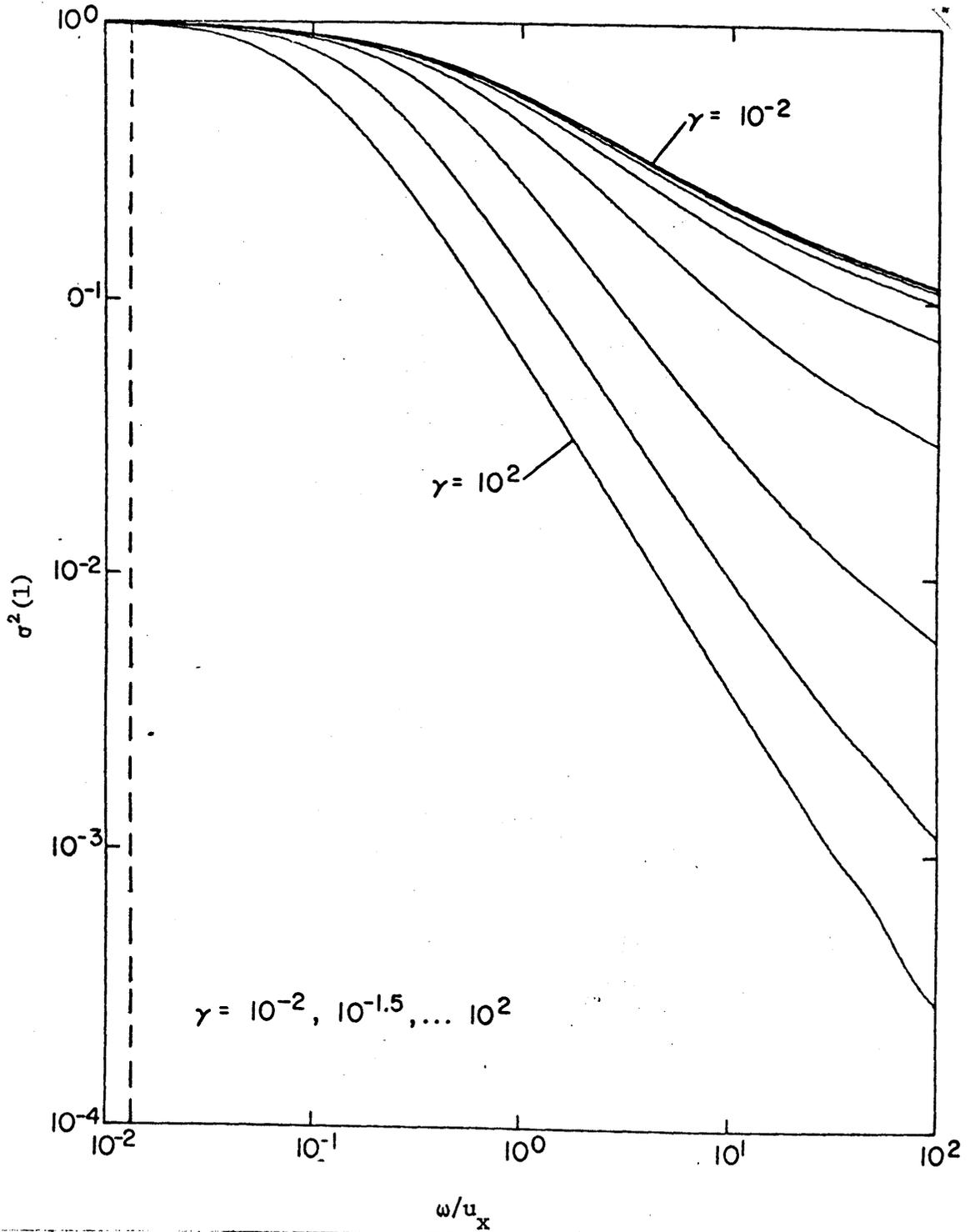
Figure 5-4. Relationship between  $\sigma^2(L)$  and  $\omega/u_x$  for determining the lateral dimensions of the plume.
