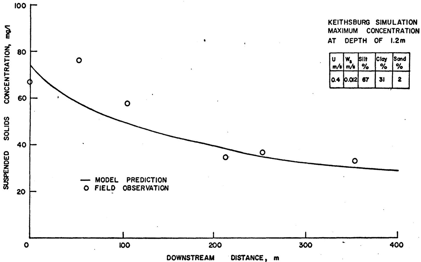
Figure 6-28. Line of maximum sediment concentration at depth of 1.2 m - Keithsburg, Illinois.
