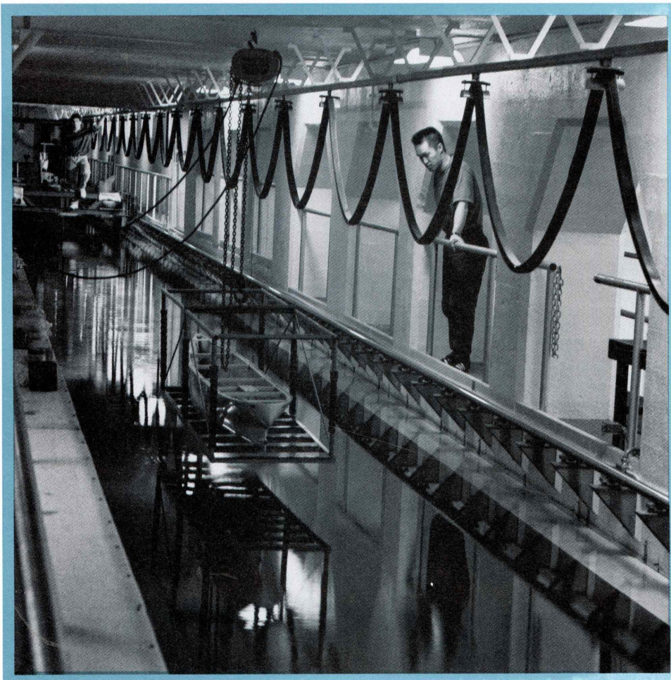
the 100 meter x 3 meter x 3 meter ship towing tank
