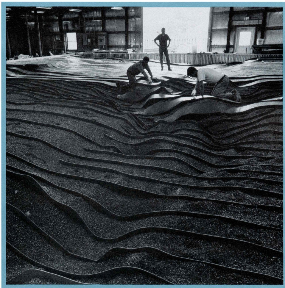
rock island dam forebay model under construction in oakdale annex
