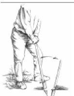
Insert planting bar at an angle, then push forward to an upright position.
