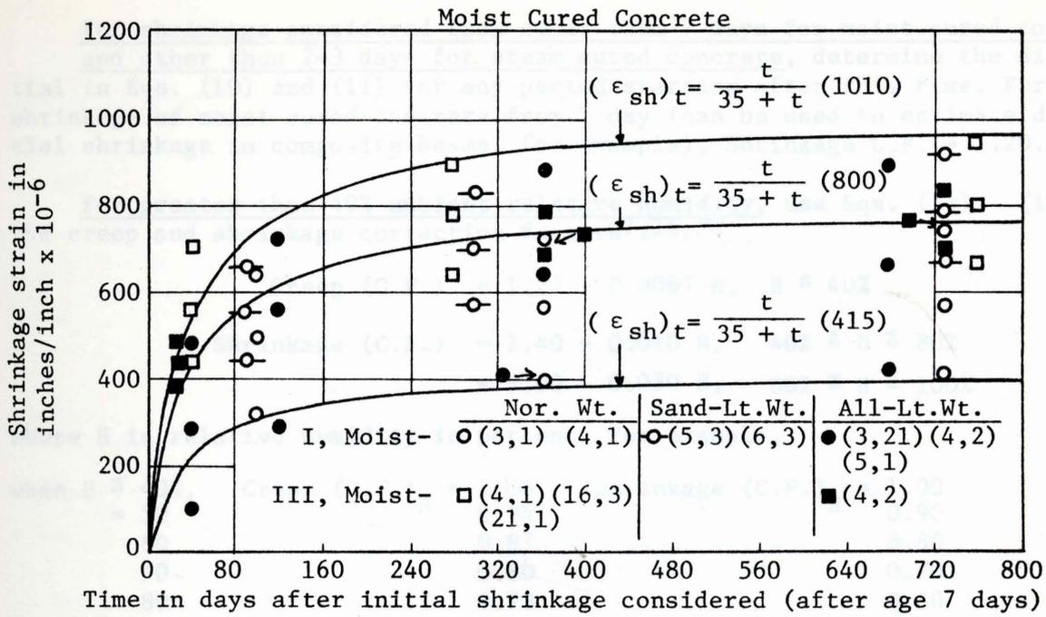
Fig. 4--Shrinkage strain versus time curves using Eq. (12), and comparisons with the data from Refs. 3 - 6, 16, 21. For each condition indicated, upper and lower limits and average values are plotted. All data were reduced to "standard conditions" using the corr. factors herein. For each set of data, (3,21) refers to Ref. 3, and 21 data pts., for example
