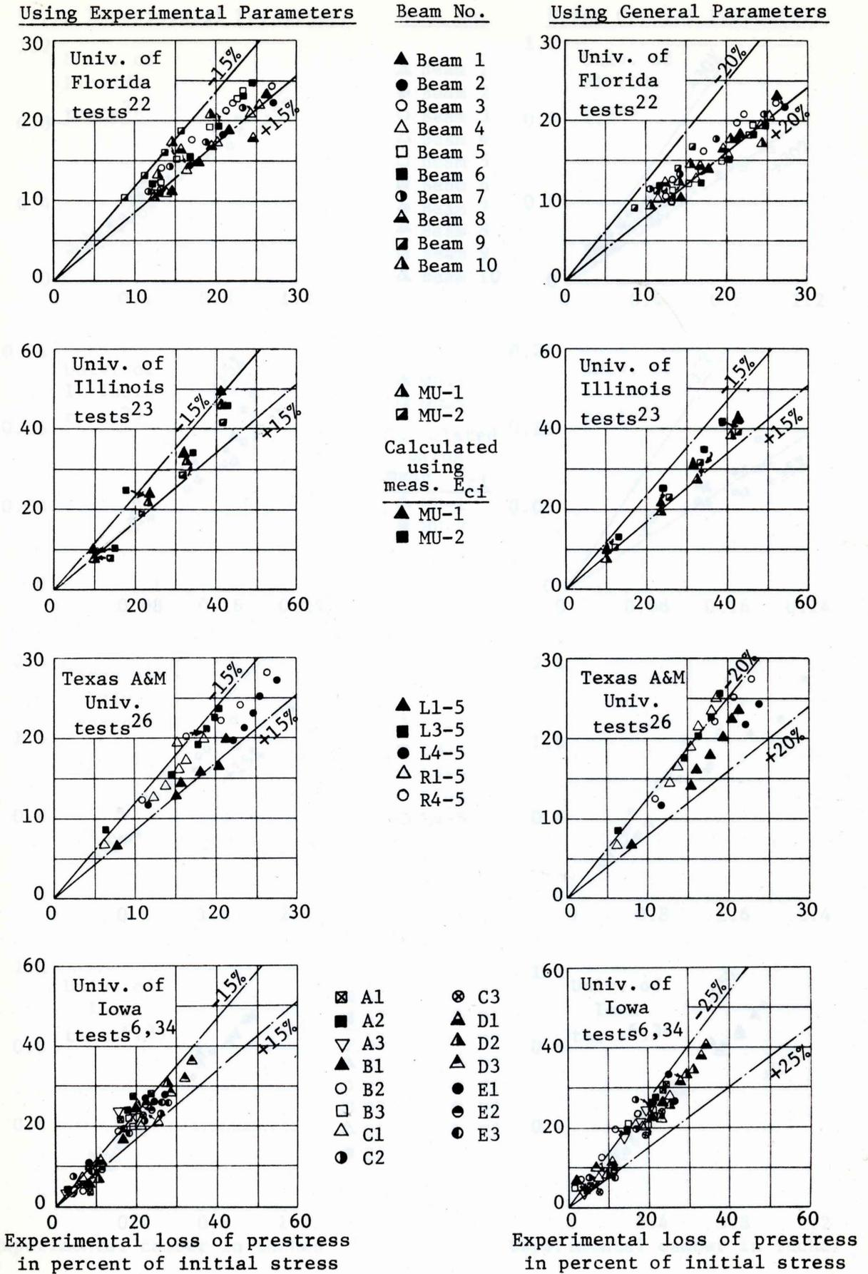
Fig. 8--Comparison of experimental and computed (using Eqs. 17 and 19 with both experimental and general or average parameters) midspan loss of prestress at various ages, for several studies in the literature
