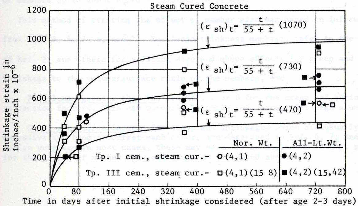
Fig. 5--Shrinkage strain versus time curves using Eq. (13), and comparisons with the data from Refs. 4 and 15. For each condition indicated, upper and lower limits and average values are plotted. All data were reduced to "standard conditions" using the corr. factors herein. For each set of data, (15,8) refers to Ref. 15 and 8 data pts., for example
