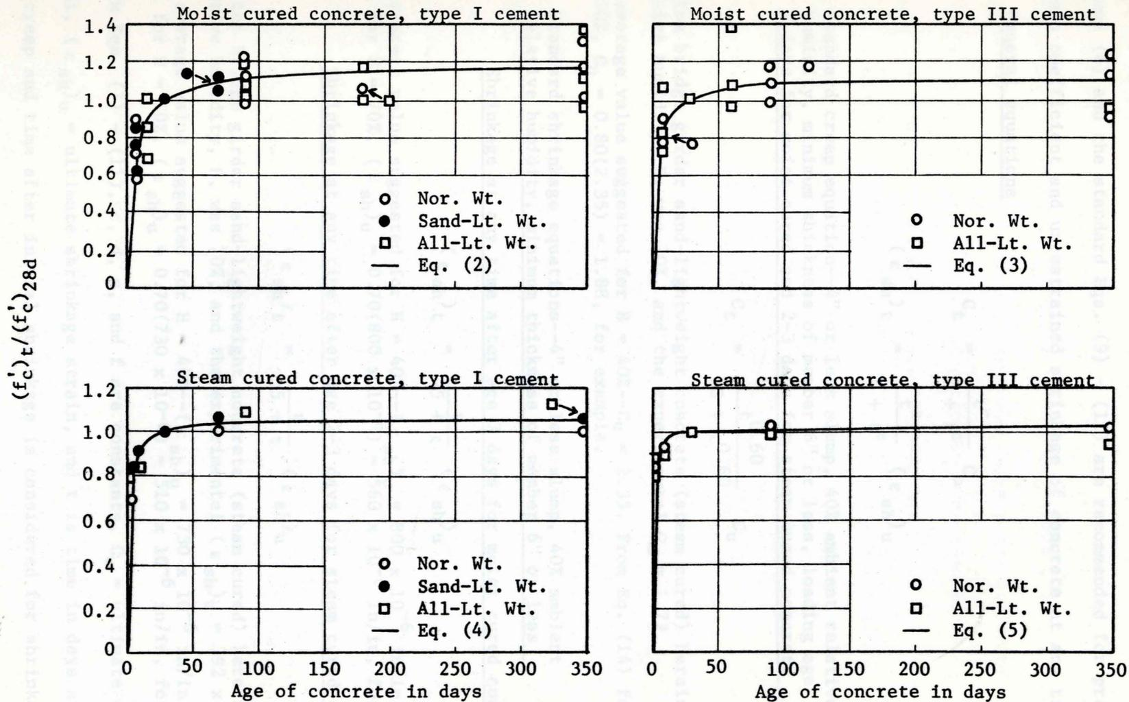
Fig. 1--Concrete strength versus time curves using Eqs. (2) - (5), and comparison with experimental data from References 1 through 6 for different weight concretes (using both moist and steam curing, and types I and III cement). Where three data points are shown for a given age, they refer to the upper and lower limits and the average value for a given set of data
