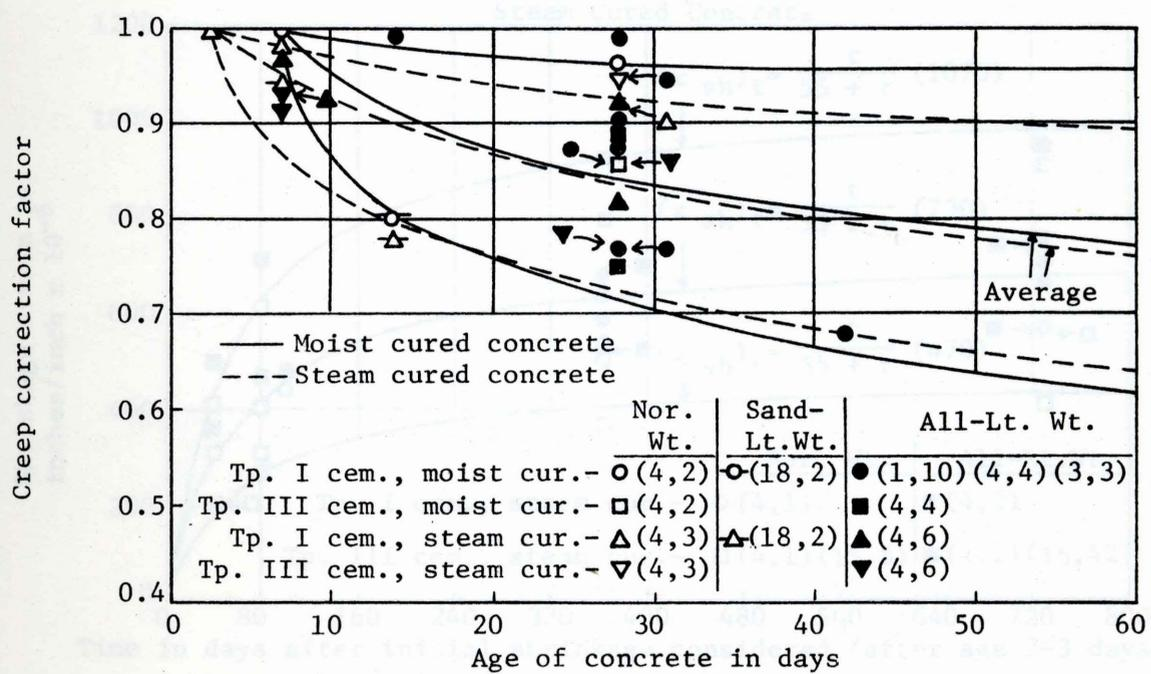
Fig. 3--Creep correction factor for time of initial loading, based on loading ages of 7 d. for moist cured and 2-3 d. for steam cured concrete. For each set of data, (4,2) refers to Ref. 4, and 2 data pts., for example. Upper and lower limit and average value curves are shown
