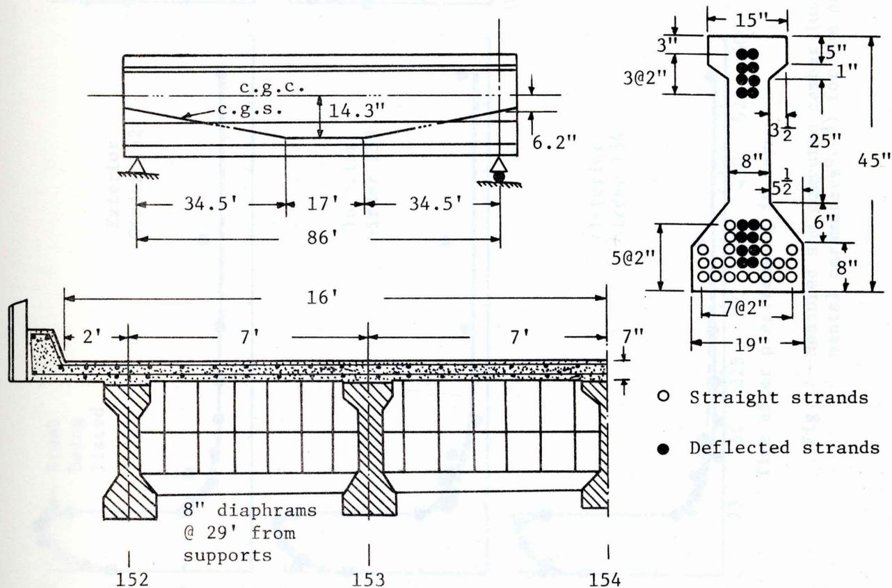
Fig. 6--Sand-lightweight concrete composite prestressed bridge girders with normal weight concrete deck slab<sup>6, 33</sup>
