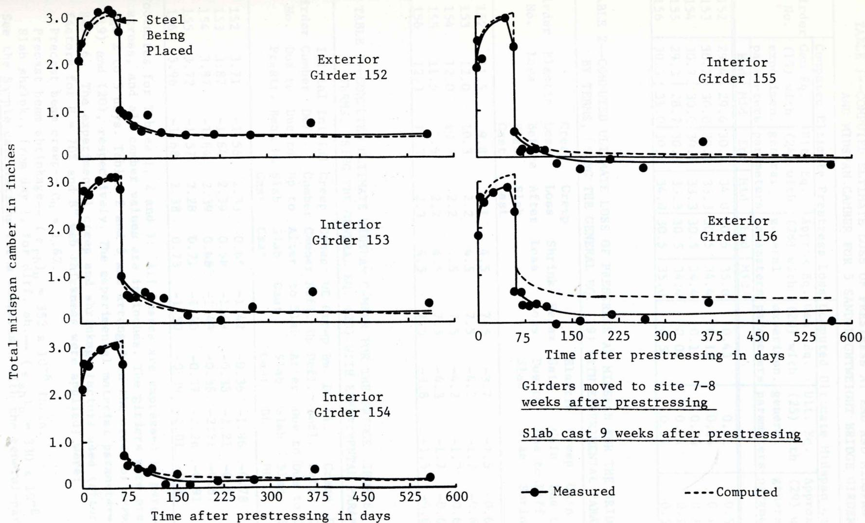
Fig. 7--Measured and computed camber (using Eq. 20 herein with experimental parameters<sup>6,33</sup>) for the sand-lightweight bridge girders
