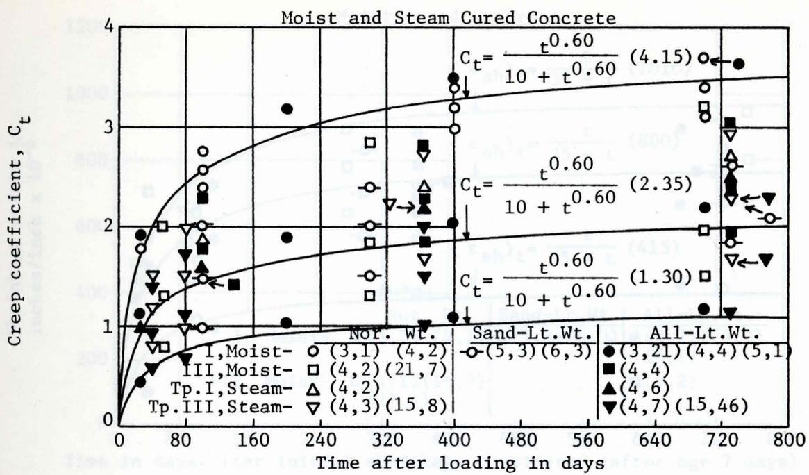
Fig. 2--Creep coefficient versus time curves using Eq. (11), and comparisons with the data from Refs. 3 - 6, 15, 21. For each condition indicated, upper and lower limits and average values are plotted. All data were reduced to "standard conditions" using the corr. factors herein. For each set of data, (3,21) refers to Ref. 3, and 21 data pts., for example
