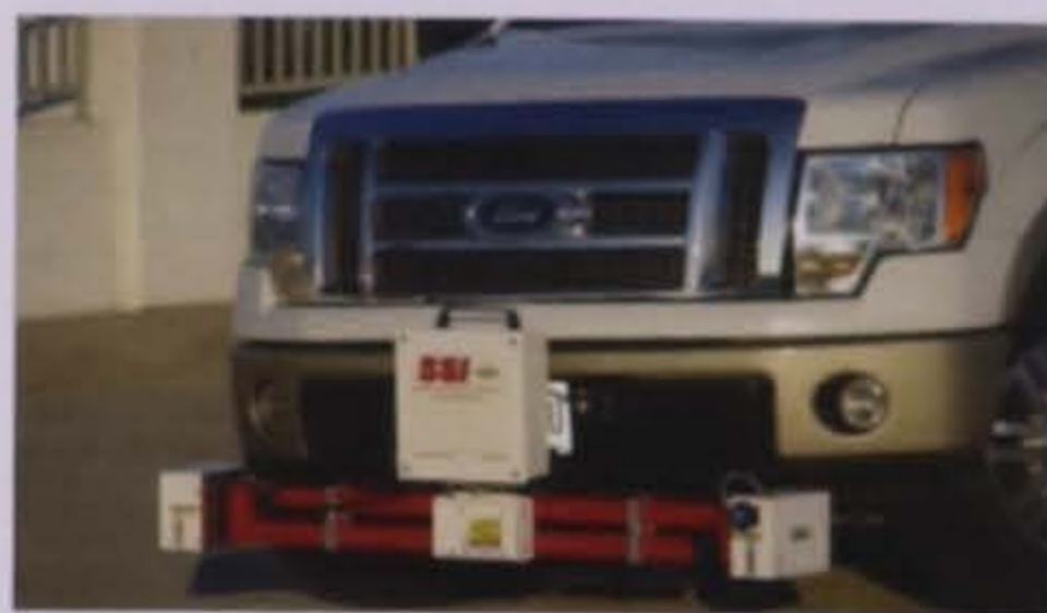
Figure 3.22. Noncontact lightweight profiler
