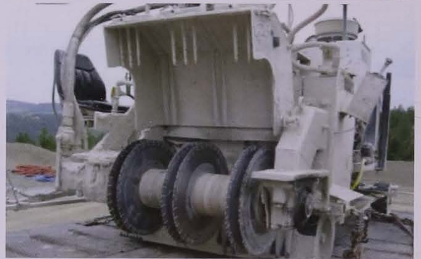
Figure 8.7. Example of diamond-bladed slot-cutting machine—three dowel bar slots per wheelpath (Pierce, Uhlmeyer, and Weston 2009)
