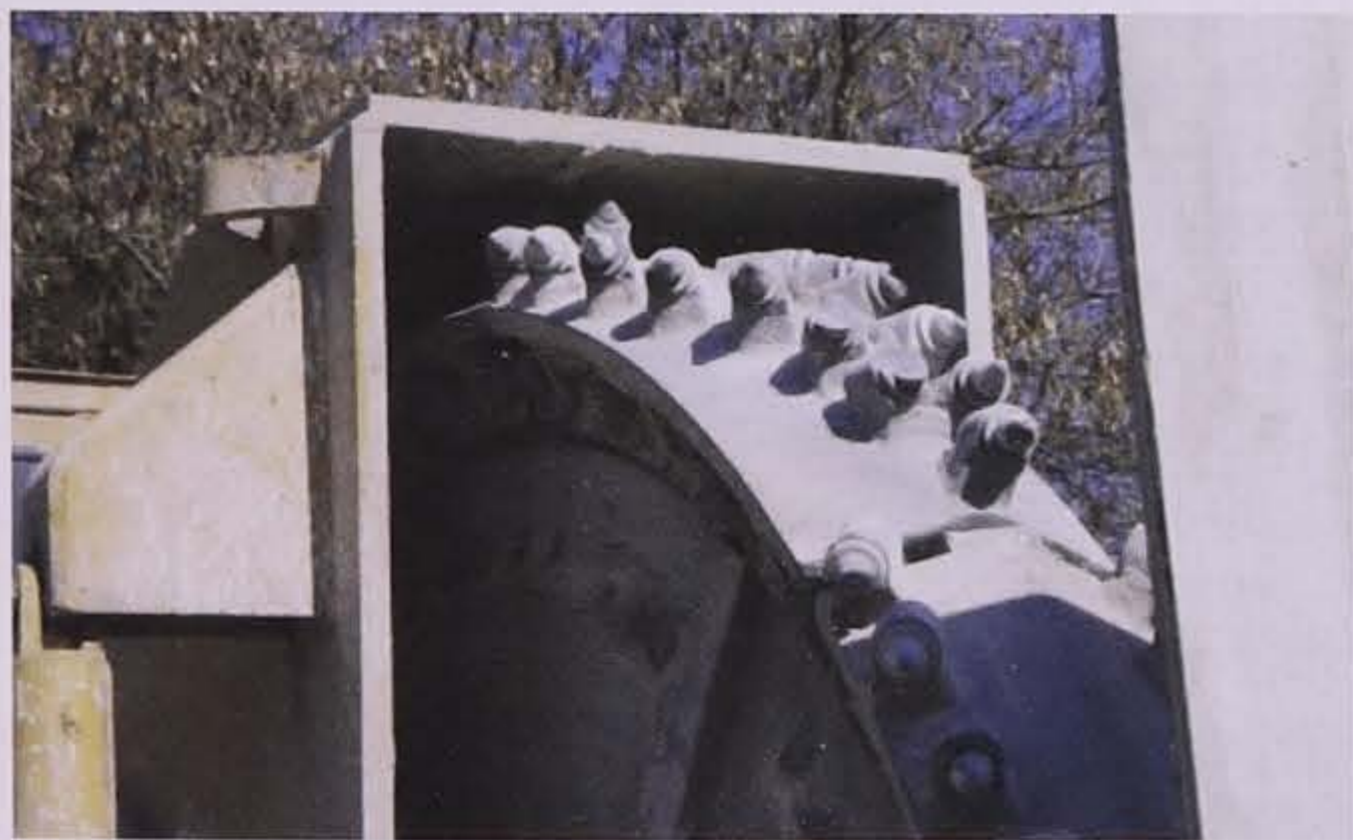
Figure 5.14. "V" shape milling head (top) and milling pattern (bottom) (Frentress and Harrington 2012)
