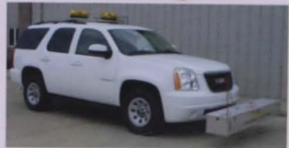
Figure 3.23. Examples of portable laser profiler (SSI 2013, ICC 2013, Ames 2013)
