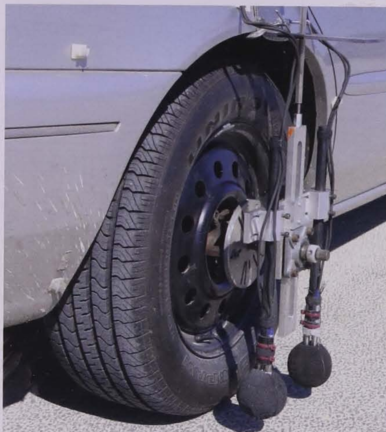
Figure 3.20. OBSI testing configuration (Rasmussen, Sohaney, and Wiegand 2011)
