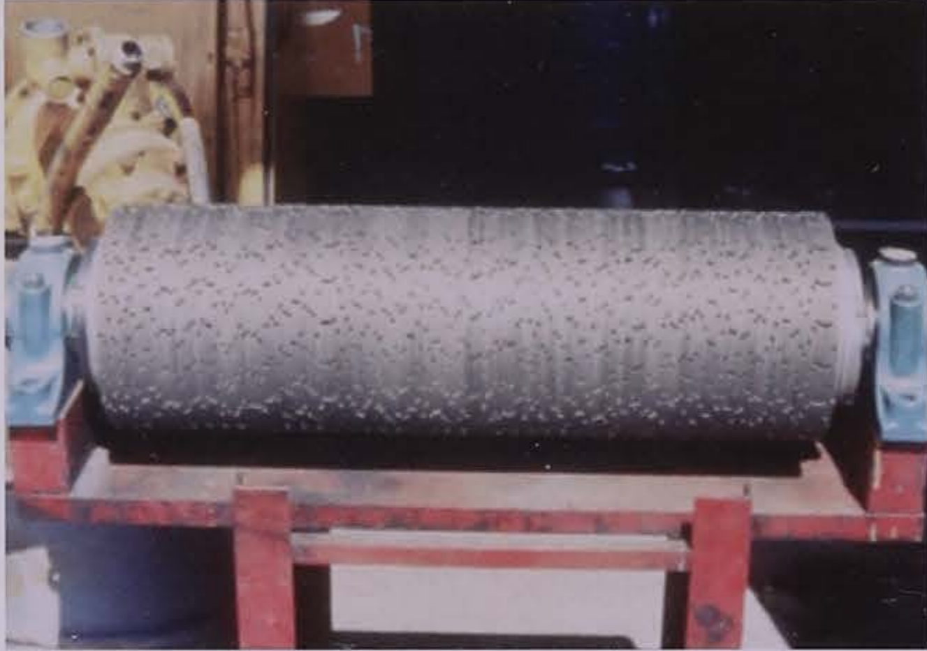
Figure 9.14. Diamond grinding cutting head (courtesy of John Roberts, IGGA)
