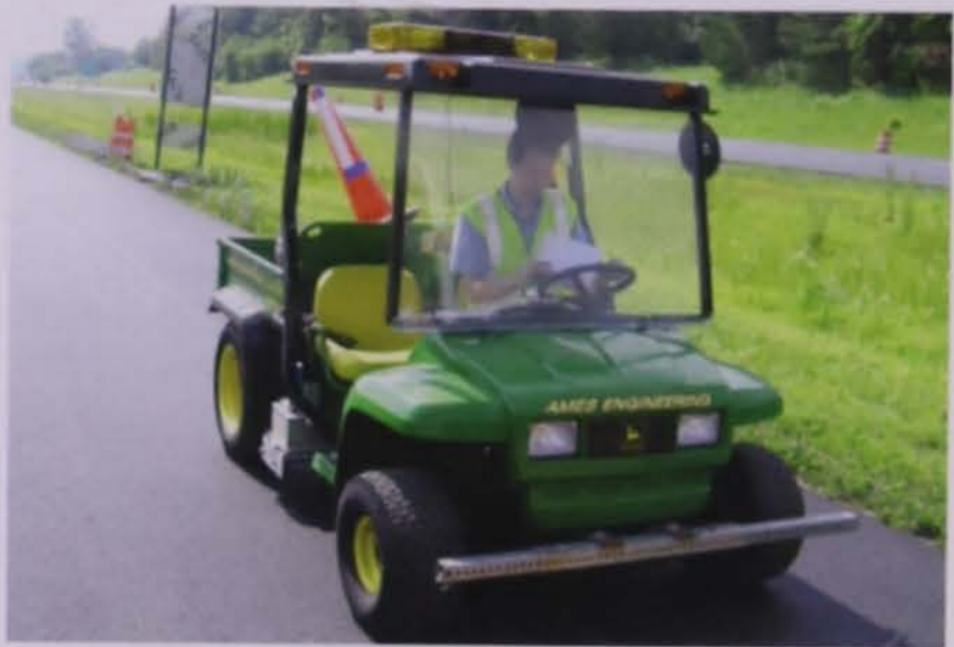
Figure 3.22. Noncontact lightweight profiler
