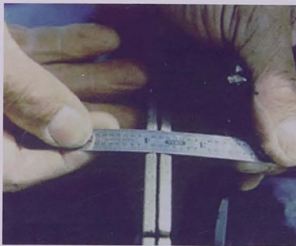
Figure 10.8. Ganged sawblades to provide desired cutting width
