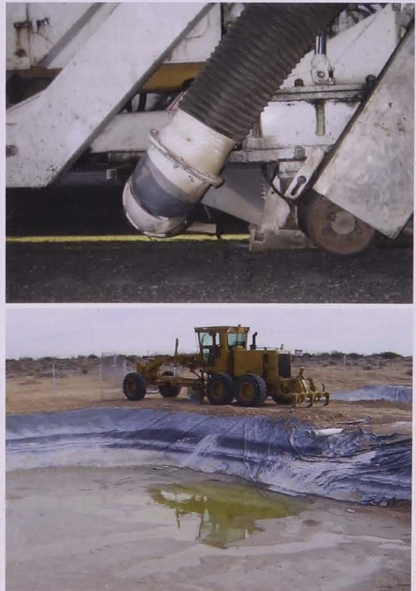
Figure 9.20. Vacuum system (top) and slurry deposit in settlement pond (bottom) (IGGA 2010)
