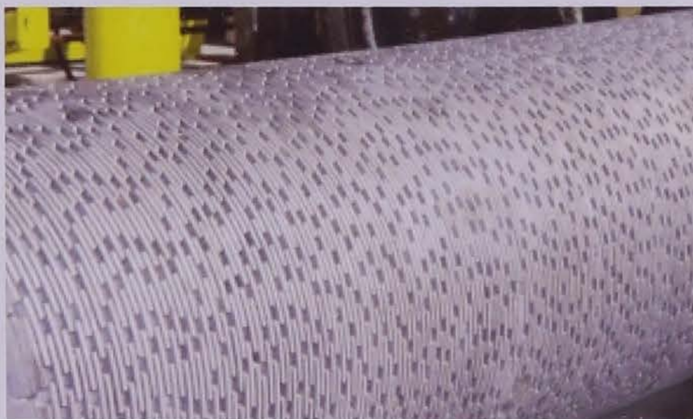
a. Conventional diamond grinding head
