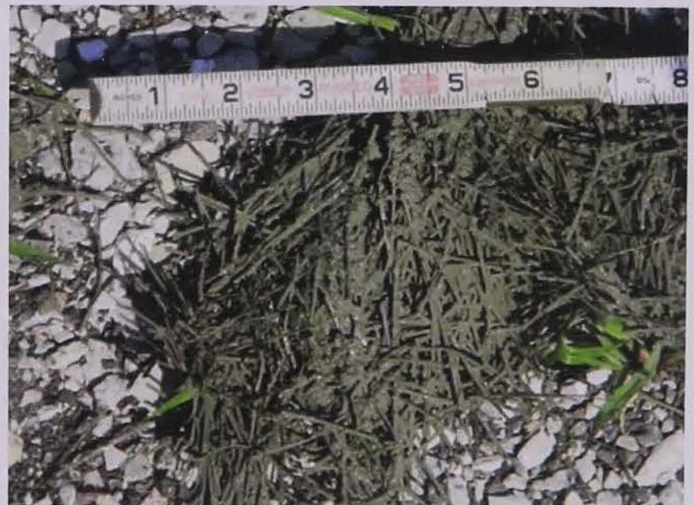
Figure 11.15. Synthetic fibers (Harrington and Fick 2014)
