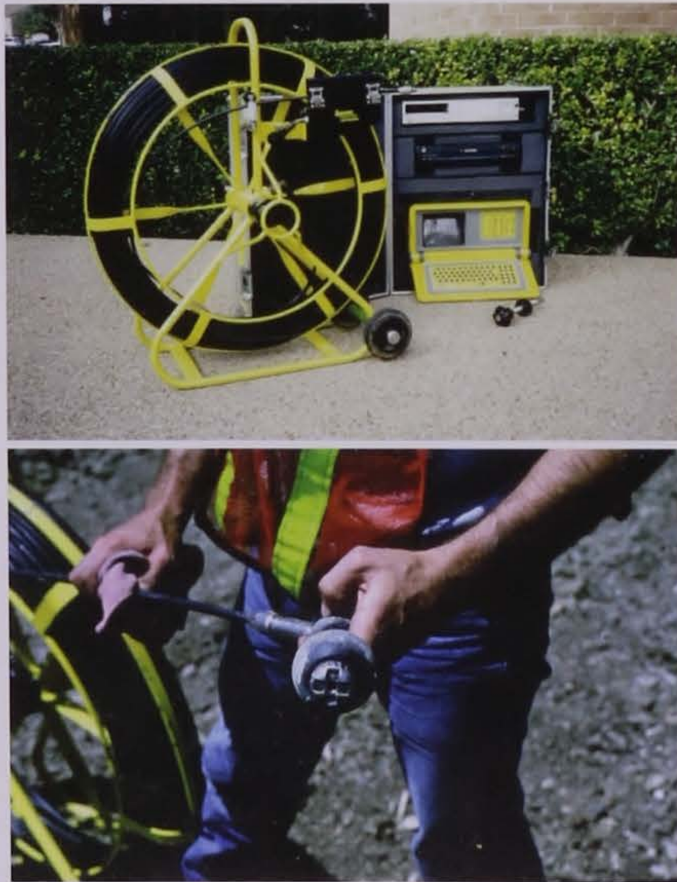
Figure 7.18. Video system (top) and camera head (bottom) (NHI 1999)
