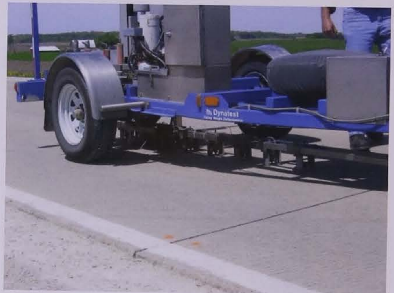
Figure 3.5. Example of FWD showing sensor bar
