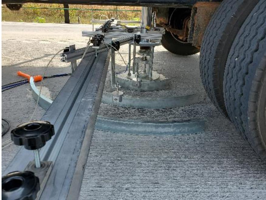
**Figure 18. 12 in. diameter plate setup with reference beam for deflection basin measurements on PCC overlay**
