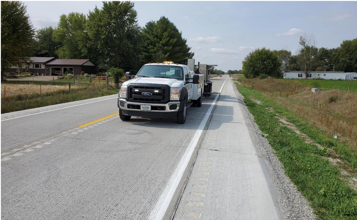
**Figure 15. APLT equipment setup on the existing ACC layer (top) and after PCC overlay (bottom)**
