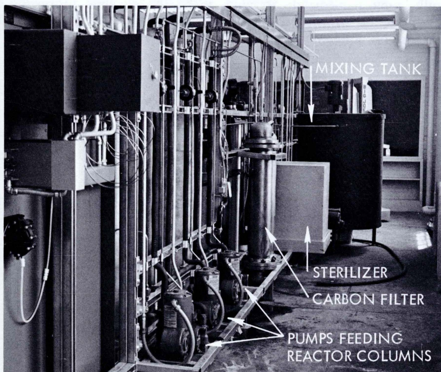
Two views of the pilot scale glucoamylase reactor system. The water tank flows into the mixing tank, where starch, water, and acid are mixed. This mixture is fed through a steam sterilizer, cooler, carbon adsorber, and filter before being pumped into the reactor columns, where the starch intermediates are converted to glucose.
