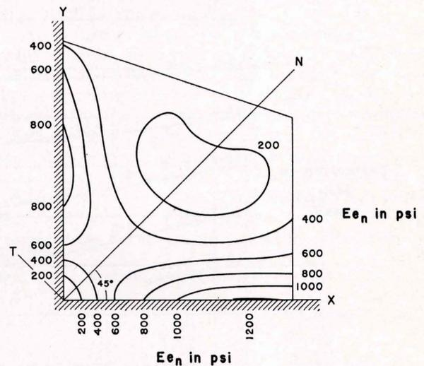
Fig. 26.  $E_{e_n}$  contours for  $p_f = 1$  psi.
