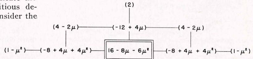
This procedure was followed for all typical points of a plate resembling a wingwall (with simplified upper edge) and the various quantities were evaluated for  $\mu = 0.30$ . Resulting coefficient patterns for these typical points are
