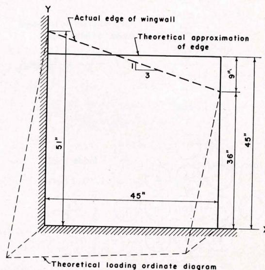
Fig. 4. Theoretical approximation of sloping edge.
