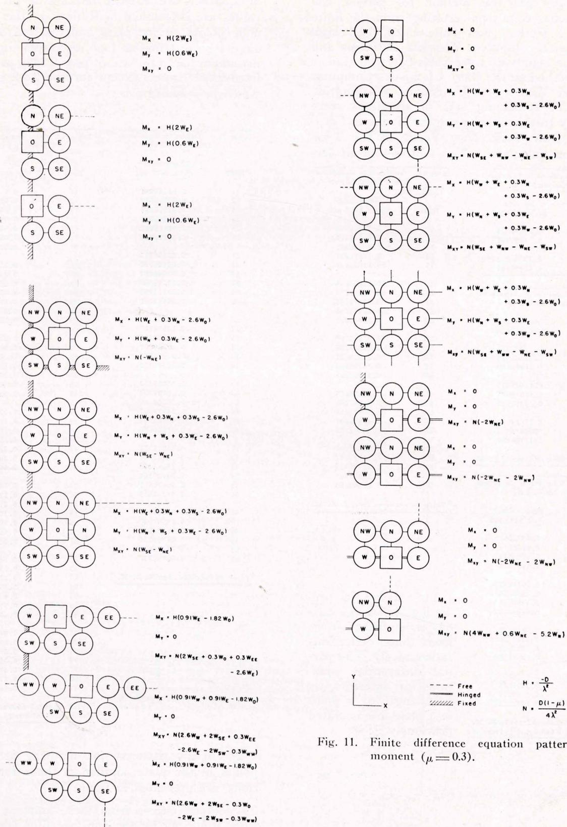
Fig. 11. Finite difference equation patterns for moment ( $\mu = 0.3$ ).
