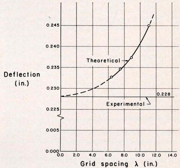
Fig. 28. Convergence graph for deflection at free corner for  $p_f=1$  psi.
