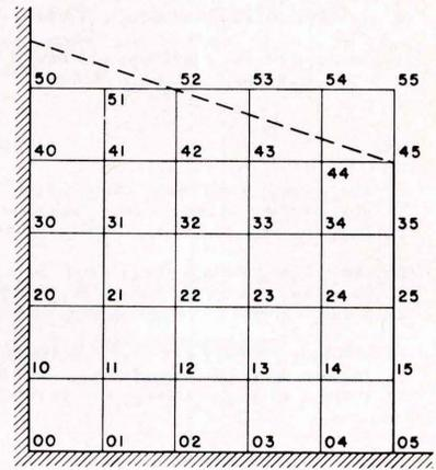
Fig. 8. Node notation for 5 x 5 grid.
