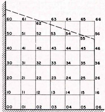
Fig. 9. Node notation for 6 x 6 grid.
