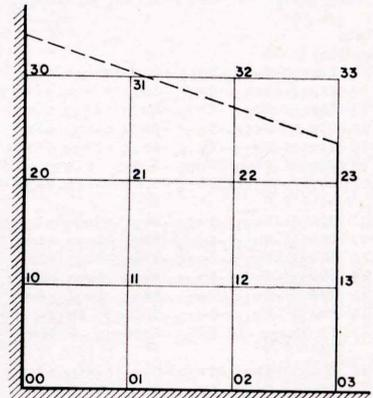
Fig. 6. Node notation for 3x3 grid.
