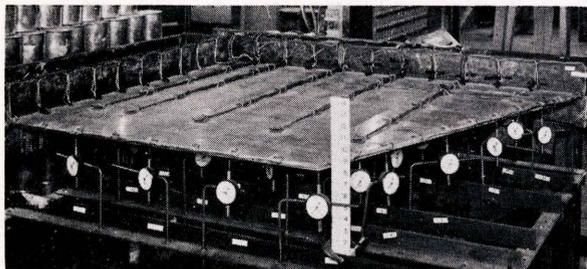
Fig. 13. Plate before loading.
