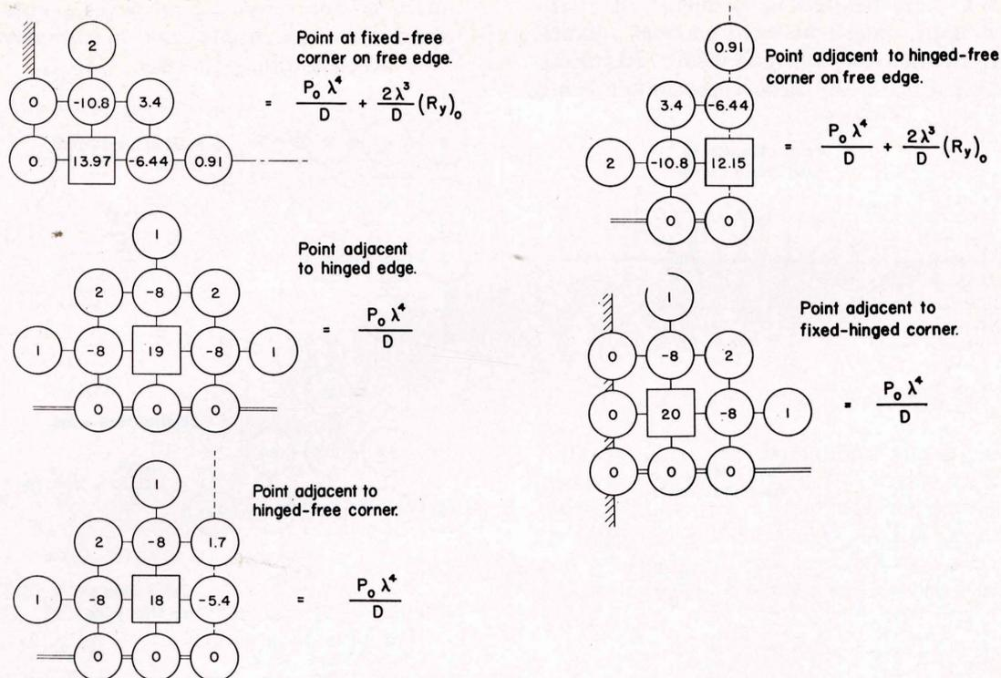
Fig. 3 cont'd. Finite difference equation coefficient patterns for deflection ( $\mu = 0.30$ ).
