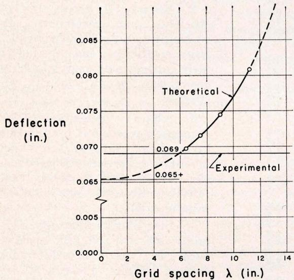
Fig. 27. Convergence graph for deflection at center of  $\frac{1}{2}$  in. plate for  $p_f=1$  psi.
