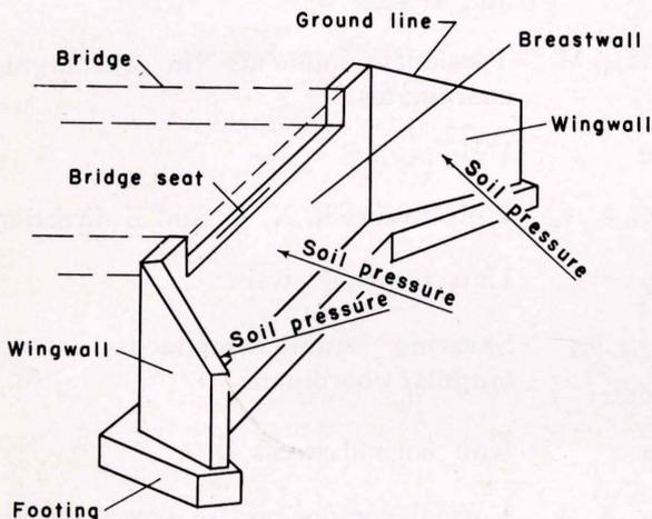
Fig. 1. Reinforced concrete bridge abutment.
