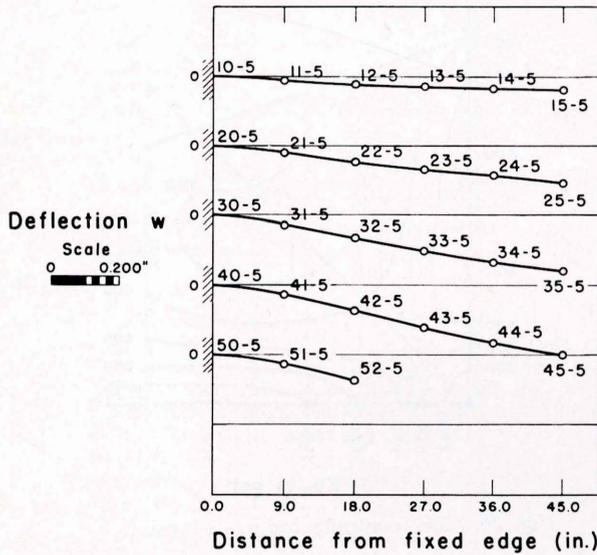
Fig. 19. Deflection sections parallel to x-axis.
