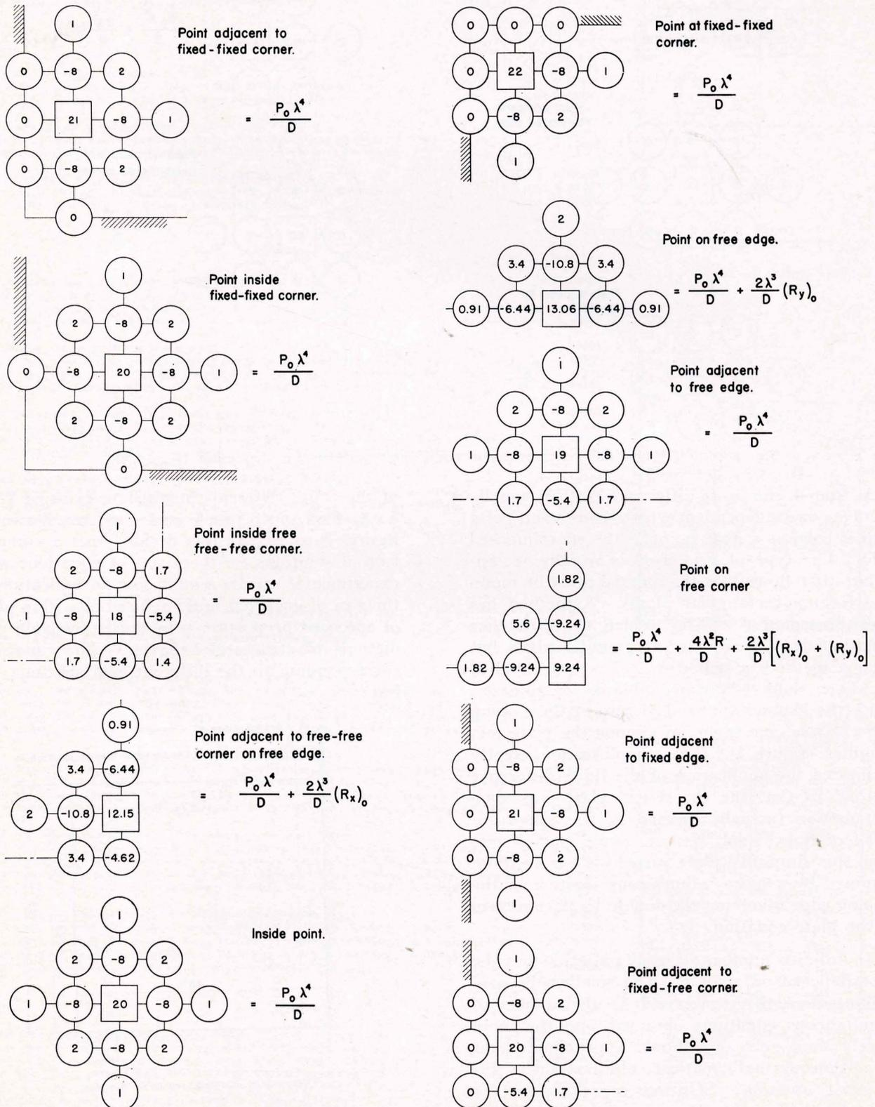
Fig. 3. Finite difference equation coefficient patterns for deflection ( $\mu = 0.30$ ).
