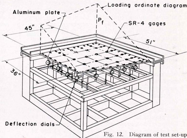
Fig. 12. Diagram of test set-up.
