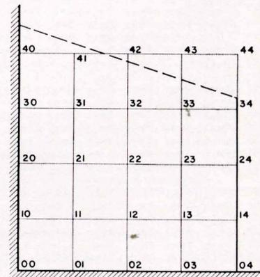
Fig. 7. Node notation for 4x4 grid.
