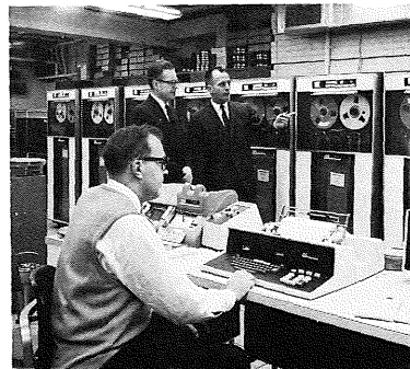
Figure 3-1a and b. State University of Iowa Computer Facility, Including IBM 7040, Two IBM 1401 Units
