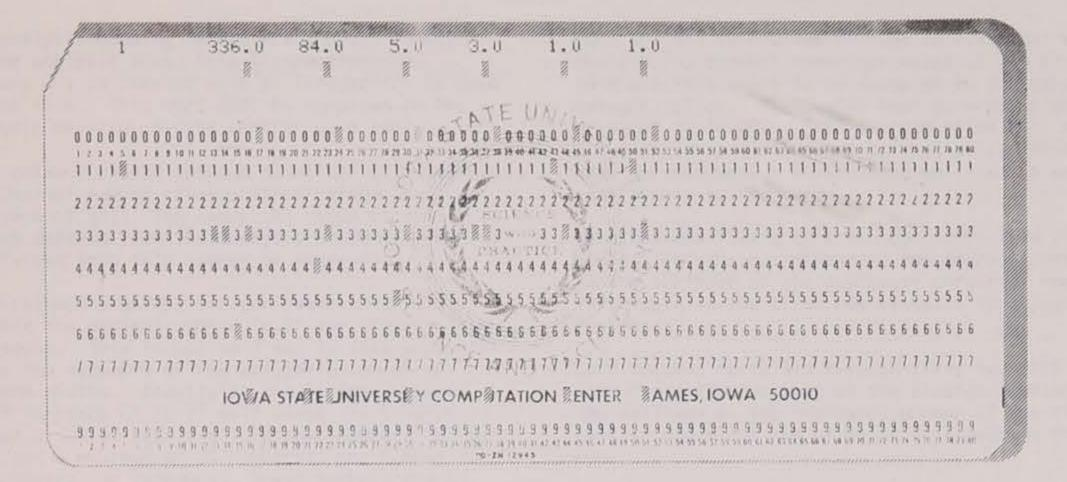
Figure #2, Instruction card for specifying the output and process parameters for the map matrix.
