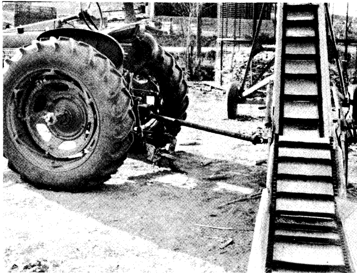
Figure 12: The tractor and PTO driven elevator in the above picture were being used during the harvesting of eared corn. While using this equipment, the operator would mount the tractor platform from the left rear to start the tractor and engage the PTO. However, he dismounted from the right rear and stepped across the PTO to return to the elevator hopper. Such a pattern was particularly dangerous because of two conditions: (a) there was eared corn strewn on the ground around the tractor, and (b) the portion of the PTO which connects to the elevator was unshielded and the end of the bolt protruded from the shaft.
