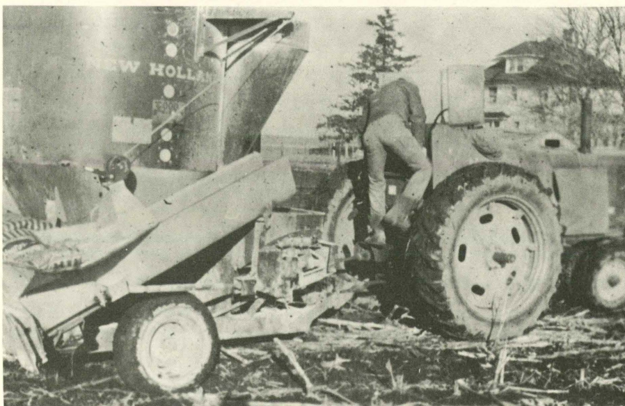
Figure 14: Operator mounting tractor to disengage PTO and move the equipment.
