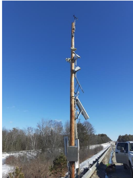
Figure 22. Friction sensors mounted at the Etna, Maine, site
