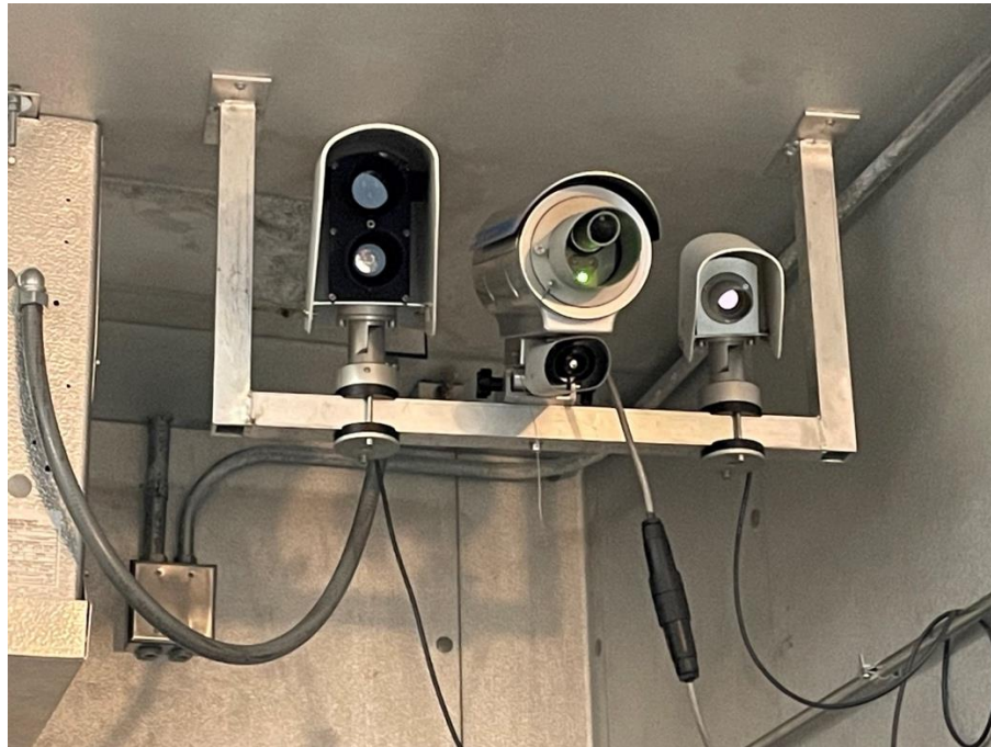
Figure 5. Sensor mounting configuration in the NCAR cold laboratory
