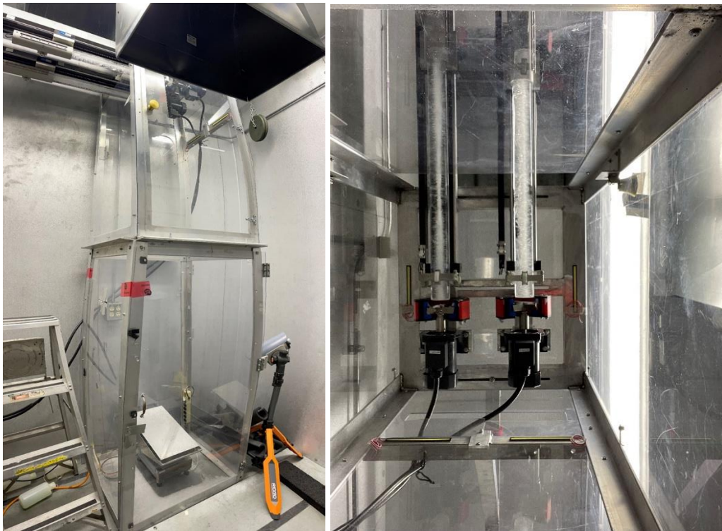
Figure 1. Snow machine in cold chamber (left) and ice cylinders mounted in the machine used to make snow (right)
