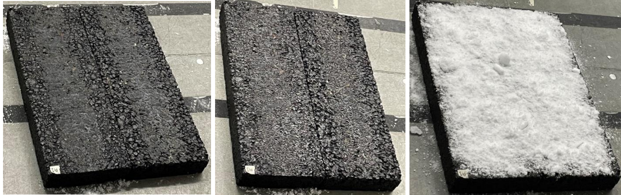
Figure 4. Warm to cold storm scenario showing dry pavement above freezing (above 32°F, left), wet pavement at freezing temperatures (below 32°F, middle), and snow on icy pavement with temperatures well below freezing (below 32°F, right)
