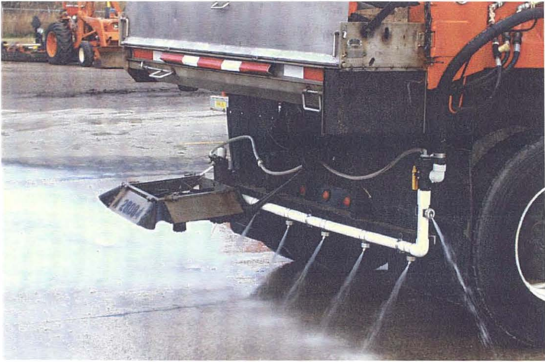
Streamer nozzles - Provide traveling public with dry surface on part of the roadway
