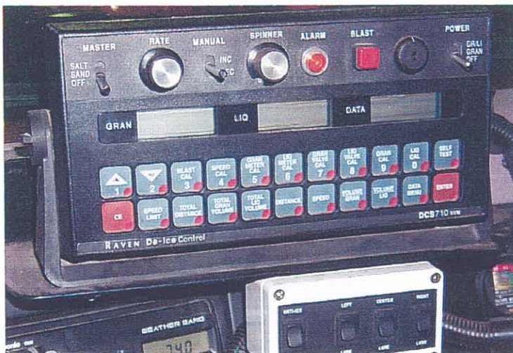
Old Raven DCS 710, with boom control, will control granular (salt/ sand) or granular with prewet, or anti-ice liquid only.
