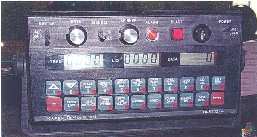
Raven DCS 700 spreader controller will control either salt or sand only or with a liquid simultaneously. (ground speed oriented)
