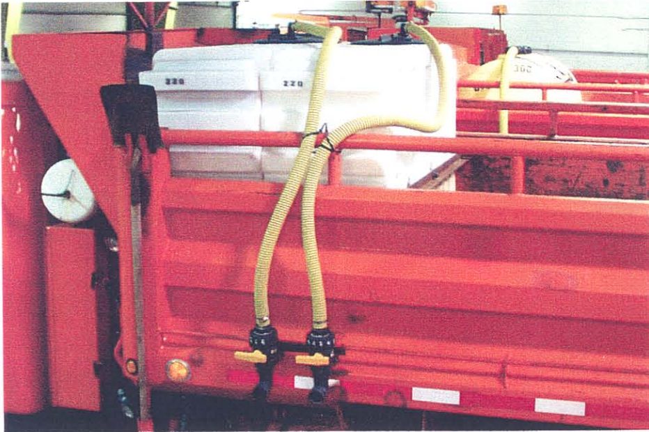
2 – 220 gallon ice ban/ brine tanks in a tandem axle that can carry an additional 9.5 tons of dry material.
