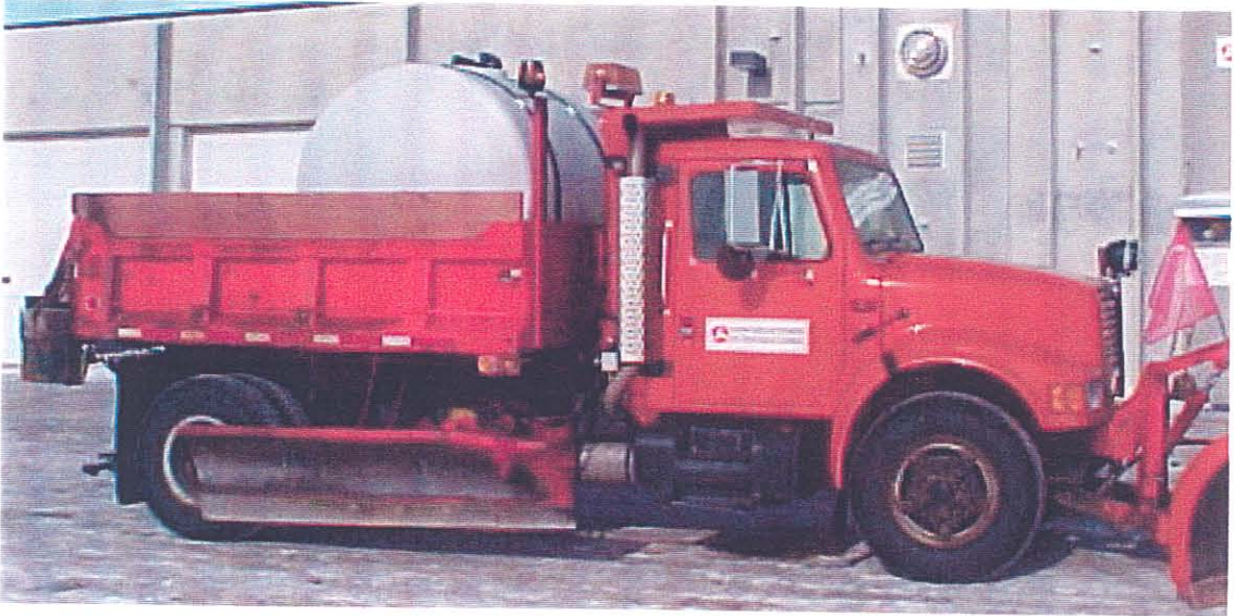
900 gallon single axle, with dry capacity of 3 tons of salt
