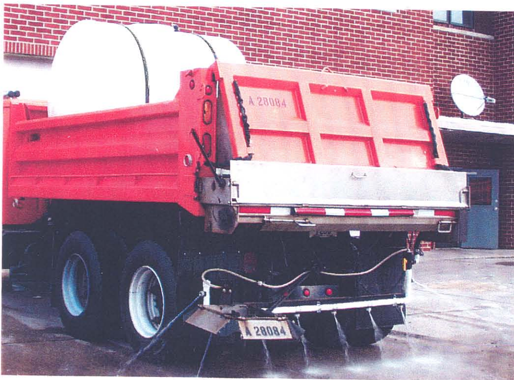
1-900 gallon tank mounted on a tandem axle truck, capable of dry and liquid salt applications simultaneously and carry an additional 7.4 tons of dry material.
