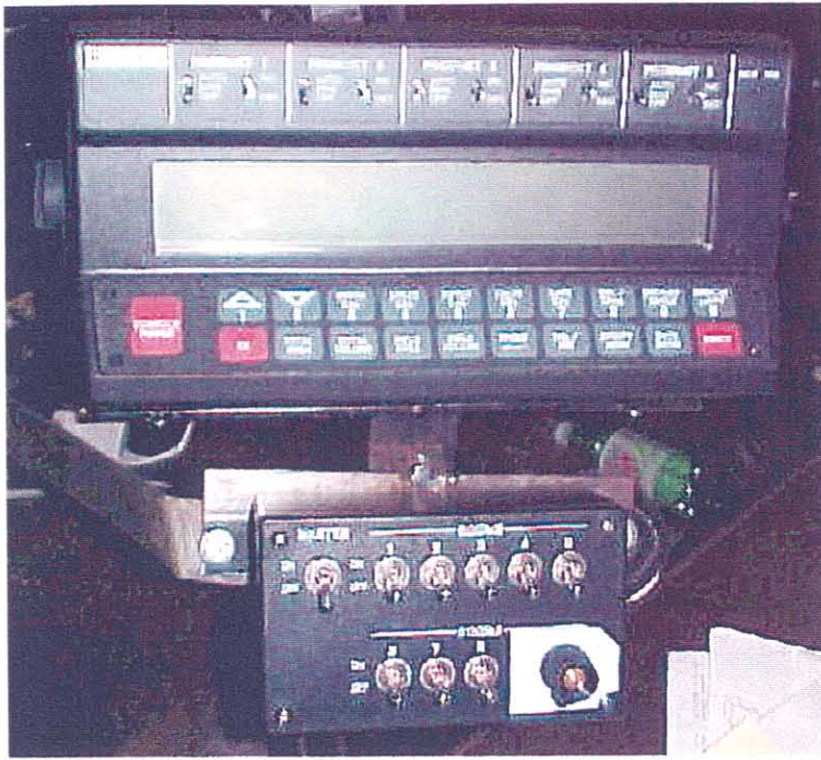
Raven SCS 760 control unit will control five products independently.
