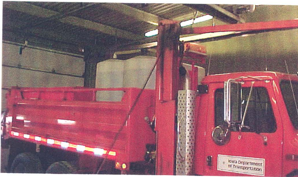
2 – 375 gallon tanks mounted on a tandem axle truck that can carry an additional 8 tons of dry material.
