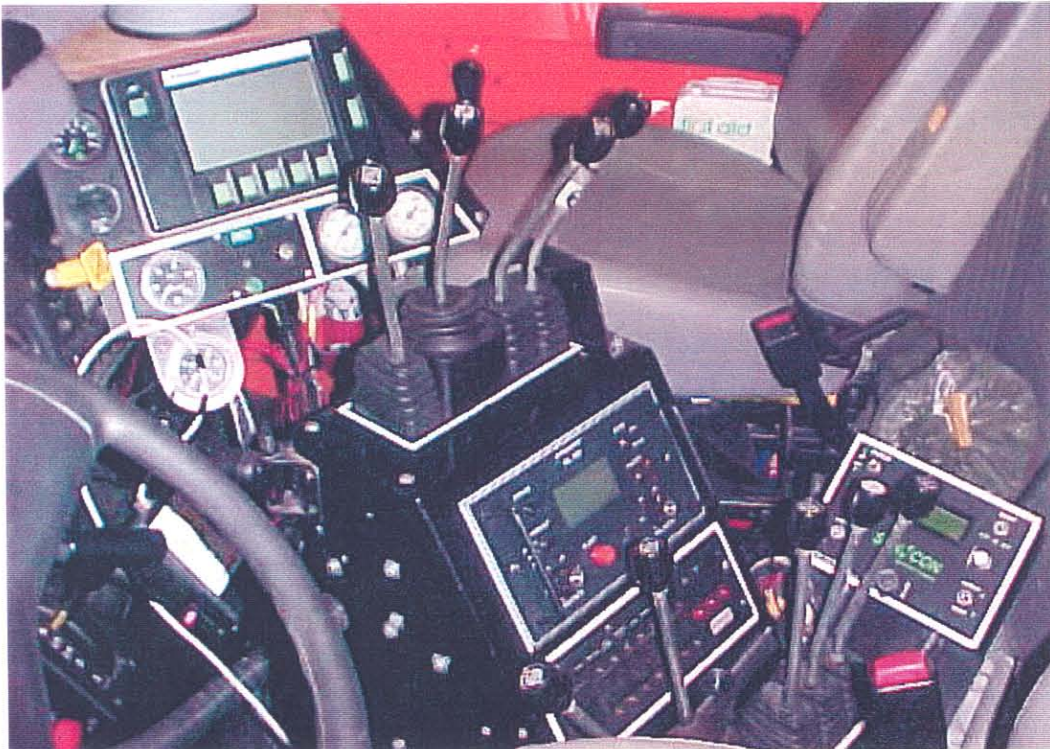
1998 Concept Vehicle has a separate Raven granular and Tee Jet liquid spreader controls.
