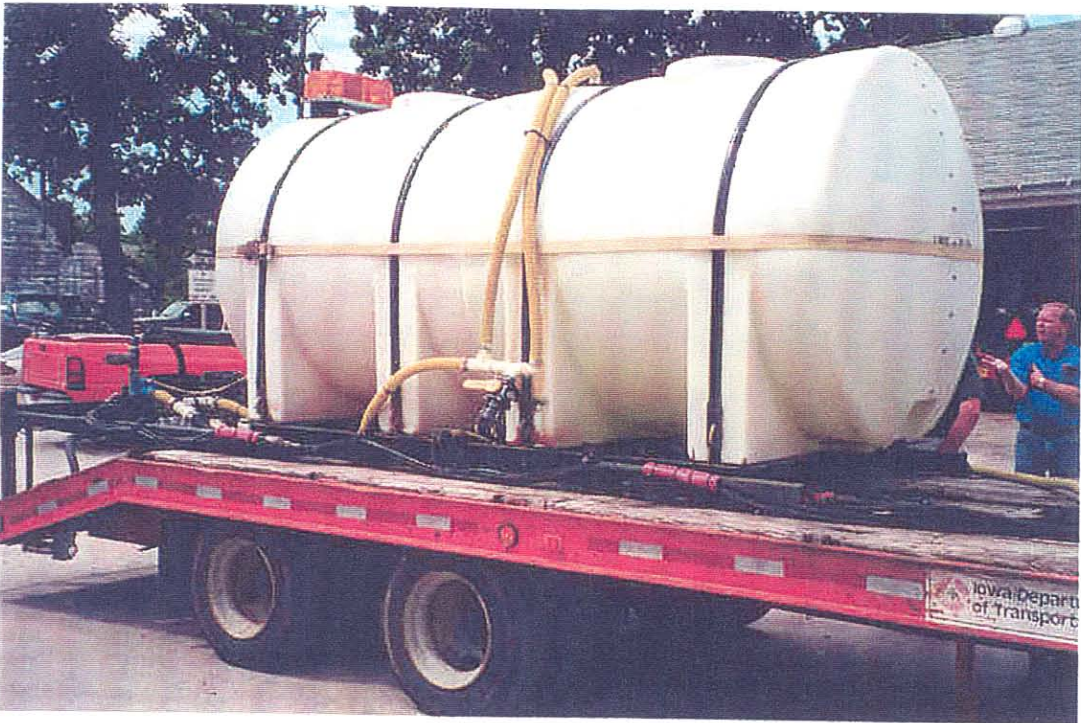
1,800 gallons mounted on a 15 ton trailer
